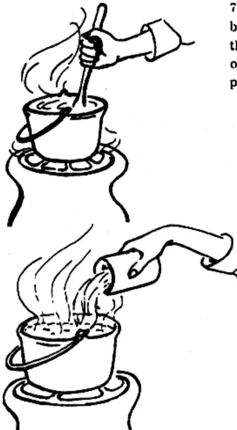
2. If available, add the ferric oxide (rust) to the solution. Increase the flame under the mixture until it boils gently.
