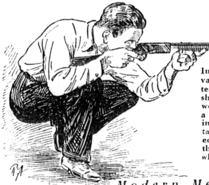
Impact power of cartridges of various makes can be handily tested by the simple method shown here. A block of hardwood is placed on the edge of a box and bullets discharged into it from a uniform distance. Comparison is afforded by the varying distances the block will be thrown when different shells are used.
