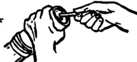
b. Press the rod about 1/2 in. (1 cm) into the middle of the top of the explosive charge to form a hole for the blasting cap.
