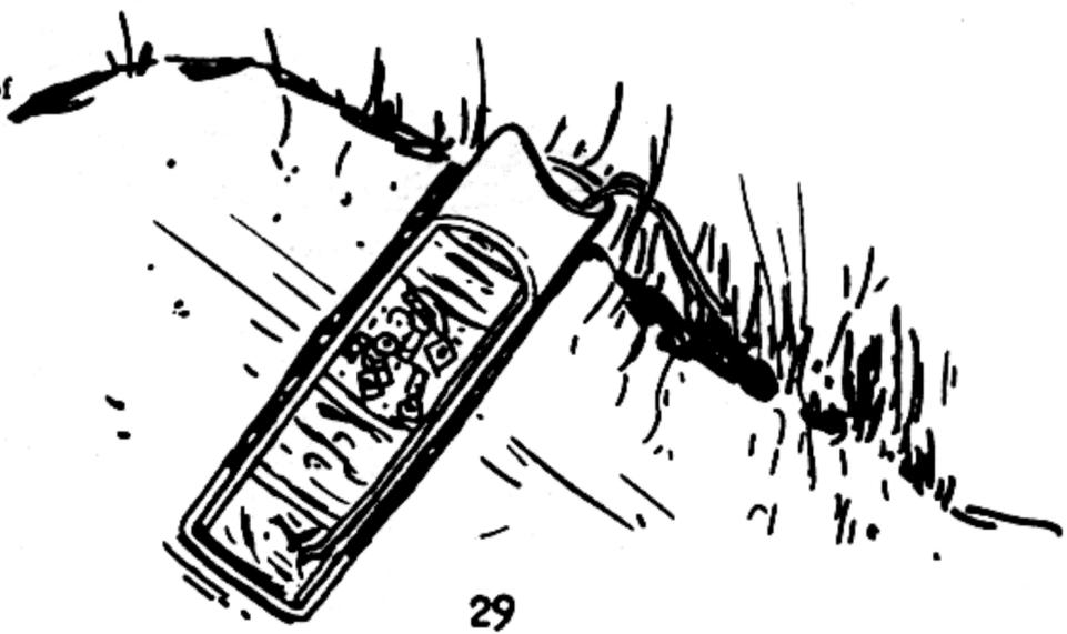
2. Connect firing leads to battery and switch. Mine can be remotely fired when needed or attached to trip device placed in path of advancing troops.
