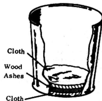
2. Place wood ashes on cloth and spread to make a layer about the thickness of the cloth. Place second piece of cloth on top of ashes.
