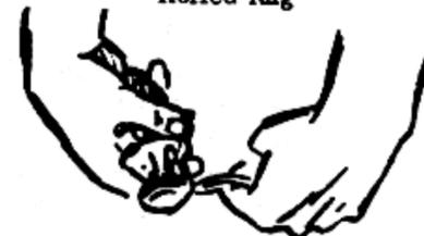
**CAUTION:** If grenade safety lever is released for any reason, grenade will explode after regular time. (4 - 5 sec.)
