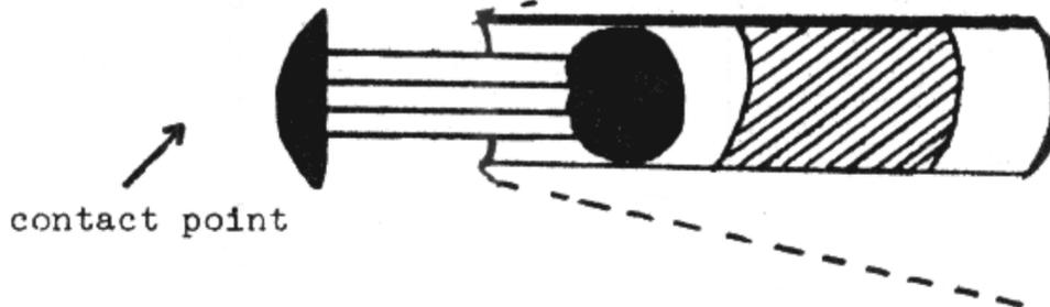
Cutaway view of friction detonator (used to detonate flying bombs)
