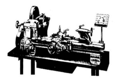
Engine Lathes are the type most frequently used in manufacturing. They are heavy-duty machine tools with all the components described previously and have power drive for all tool movements except on the compound rest.
