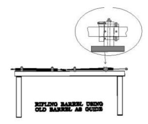
The fourth clamp is also used on the barrel being used for a guide. This must be a different type from the other, for this clamp must hold a flanged sleeve, which is clamped, tightly to the guide barrel. In this sleeve are as many holes drilled in a line around its circumference, as you desire grooves in the barrel to be rifled. A pin passes through this last clamp at a point in line with the holes drilled in the sleeve.
