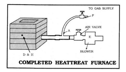
The basic tools for heat-treating are the gas torch. The torch is a simple apparatus consisting of a mixing tube into which fuel gas and a blast of air are introduced to be mixed and burned at the end of the tube. An old vacuum cleaner can be used for the air blast.
