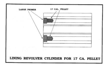
The short piece of barrel is centered in the lathe and is shaped just like a 38 or 357 case. It is made to just slip full length inside the chamber in the cylinder, with no play. The primer end is drilled to accept a large pistol primer. Drill just deep enough that it will be flush. Using a taper reamer, just ream the barrel in front of the primer so a .177 pellet will just start inside the barrel.
