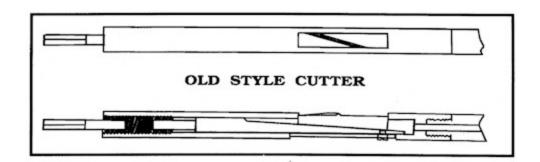
After the rifling cutter makes a cut in each groove, another shim is placed beneath the cutter. Another cut is then made in each groove until all the grooves are cut to the proper depth. A small hole is first drilled through the rifling head on the bottom of the cutter slot so a small punch can be inserted through the hole to remove the cutter out of the slot in the rifling head.
