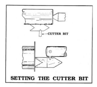
After this setup is made and the work is turned to the proper outside diameter, the work piece is left right in the lathe and the threading operation is performed. The jobs are threaded while held in a three or four jaw chuck in which they were mounted to be turned to size.
