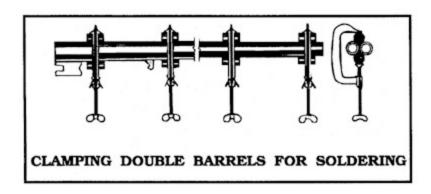
Take the finish barrel and turn the chamber end to the size needed to just slip in the old chamber section of the double barrel, or single shot. I might point out that the fit has to be very close, or you may get a bulged chamber. You can use a good low melting point SILVER
