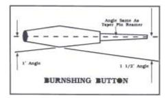
Now to set up the lathe for this taper, you will need 2 dial indicators; one will need to be at least a 1-inch travel. You will need a piece of tool steel the exact length as the carbide and end pieces. So both have to be the exact length, if not the angle will change. Make sure the tool steel is running true and center both ends.
