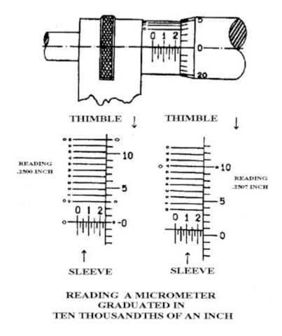
If you want very accurate measurements are required, a micrometer that has an extra scale added to the sleeve is used, enabling the micrometer to be read in ten-thousandths of an inch. This scale consists of a series of lines on the sleeve parallel to its axis.
