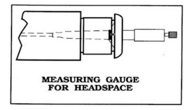
Now knowing the depth is .100 we can keep feeding the reamer in until the headspace gauge will be the right depth. The correct depth would be .095. Allowing .003 for compression of the barrel to the action, this would leave .002 on the headspace, which is about right. To set the depth, use a depth mike, placing the depth mike on the end of the headspace gauge, and measuring the depth until it read .095.
