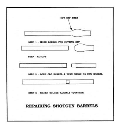
When you have achieved this fit, and have the extension barrel turned so it will just fit the counter bore with no play, it can be soldered.
