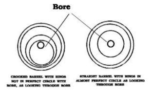
A shotgun barrel is good to practice on, as it is big, and smooth with no rifling to confuse you. It is next to impossible to straighten a barrel with a rough bore. I will also show you here how to make barrel-straightening equipment necessary to straighten the barrels.
