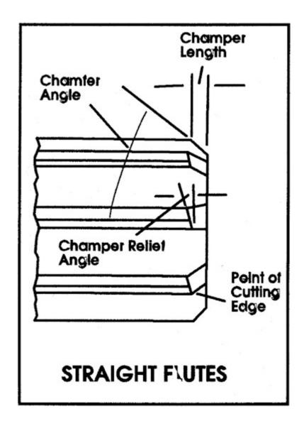
The relief of the cutting edges should be comparatively slight. They can be ground close on the tool post grinder and stoned flat with an Arkansas stone. The flat relief is what I have used all along, because the reamer has a keener cutting edge.
