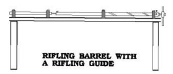
The rod, with the guide in place in the guide barrel near the end closest to the barrel to be rifled. This should be long enough so the rifling cutter clears by an inch or more the opposite end of the barrel to be rifled. With the clamps all locked and the rifling cutter in position in the head, the rifling cutter is now drawn through the barrel to be rifled, making the first cut.
