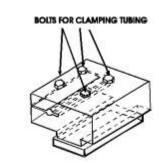
CARRIAGE BLOCK FOR HOLDING TUBING
