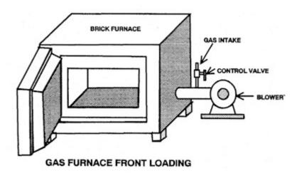
Next, you will need to cover the firebrick on the outside. Cut 1/8 inch metal to fit to the outside and top and weld this together, to form a box for the firebrick. Be sure to have a metal bottom already cut out to put under the brick so the sides can be welded to it.
