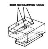
CARRIAGE BLOCK FOR HOLDING TUBING
