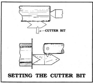
Setting the cutter bit for threading
