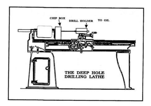
Turn on the oil, but before you do make sure that the valve is open all the way, so there is no pressure in the line. If everything is OK you are pumping the oil back to the tank, with very little oil going through the drill. Now close the valve slowly, watching the pressure on the gauge, when it gets up to 600 to 700 lbs., which is about the right pressure for 30 caliber barrels.
