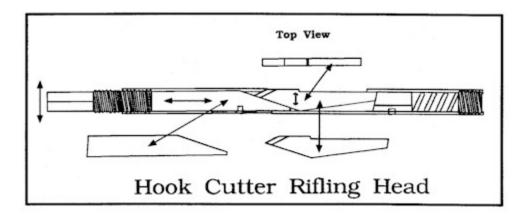
The bevel of the wedge is the same as the bevel on the bottom of the cutter, ten degrees. This beveled wedge is pushed forward by a screw. The rear of the rifling head has fine threads and is tapped into the rear of the rifling head. Turning this screw forward in the rifling head results in pushing the beveled wedge farther forward under the cutter and raises the cutting edge.
