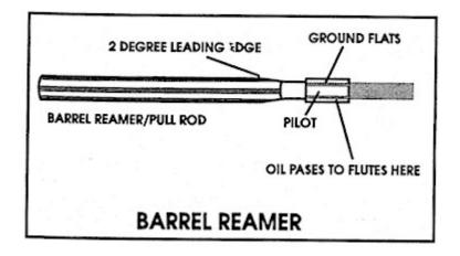
I will go through with you on making a complete set of tools for a 308-barrel. You will need two each, 5/16-inch (.312) drill rod, and 6 inches long. Once you have the two - 5/16 inch drill rod cut, go to the lathe. Chuck up one of the pieces and using a 1/4 inch center drill, center one end just deep enough to get a good center. The other end uses 3/8-inch center, and center it to the outside edge of the drill rod.
