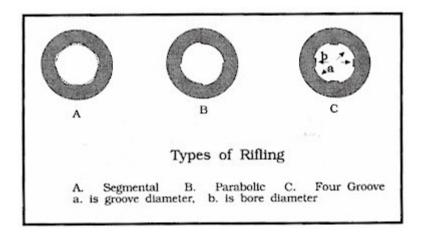
There is no way of rifling so secure as that in which the walls of the grooves are parts of radius of the bore. They should be numerous, that the hold of the lands, or the projection left between the grooves, may divide the friction and resistance as much as possible, and so permit the grooves to be as shallow as may be.
