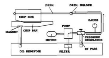
COOLANT SETUP FOR DRILLING
