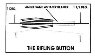
Button rifling is a cold forming process in which a small carbide button or swage, with lands cut in the button. It pulled through the gun barrel bore embosses the rifling in the bore. The button is made a few thousands larger than the finish size that is required, since the metal will return .001 to .0015 thousands.
