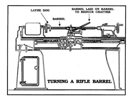
The reason for this is that if the angle on the end of the barrel is off, one side of the barrel will be thicker than the other. In turning, the barrel will probably warp. Now that the barrel is squared, put the faceplate on the lathe. Take a bar of steel that is 24 inches long that has centers in each end and has been turned true.
