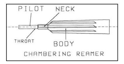
Leave all diameters about .020 larger than shown. The tool steel blank should be cut 6 1/2 to 7 inches long. Use the smallest center drills for center drilling the blank. When turning the shoulder can be left square, but there should be a recess cut in front of the shoulder, end of neck, etc. for clearance when grinding.
