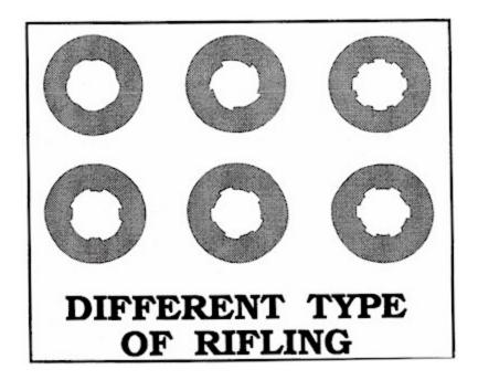
The English gunsmiths avoided the dilemma by giving the requisite pitch and making the Rifling grooves very deep, and even by having wings or lugs cast on the ball to keep it in the grooves expedients which increase the friction in the barrel and the resistance of the air enormously.
