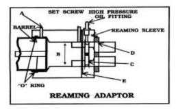
It has to be shooting out under enough pressure to get rid of the chips so they won't plug up the reamer. If it plugs up it could ruin the barrel, and probably break the reamer. Start up the lath in back gear. Make sure that the pilot of the reamer is inside the barrel, and engage the feed lever. As the reamer is starting to feed into the barrel, it may cut a little rough but it
