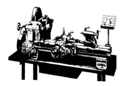
The lathe should be able to turn at least 2000 rpm or higher. It should have tapered bearings in the head stock spindle.
