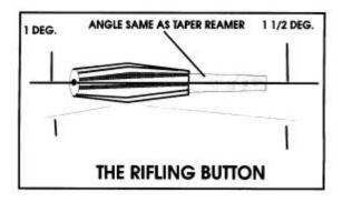
Now cut 2 pieces of the 5/16-drill rod, 1/2 inch long, square and true the ends, center drill one end. You will need a small V center bar. Lay the carbide piece in the V, and the short drill rod, with the centers to the outside. Put some low melting silver solder paste on the ends, press them together and heat them up until the silver solder melts, and let cool. Be careful that you do not over heat the carbide or heat it up to fast, as it will crack.
