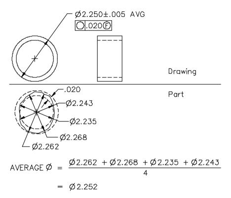
Figure 5-45 Circularity tolerance with average diameter
