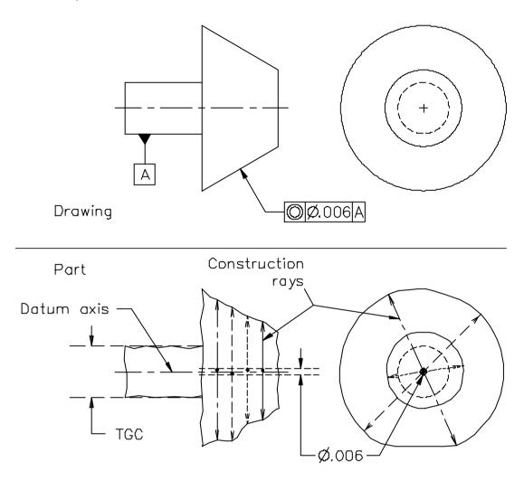
Figure 5-146 Symmetry construction rays
