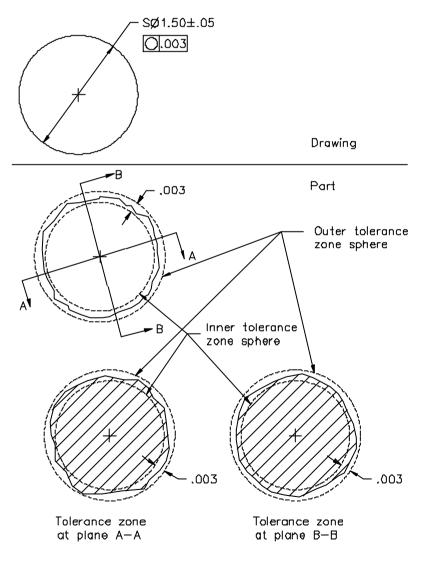
Figure 5-43 Circularity tolerance applied to a spherical feature
