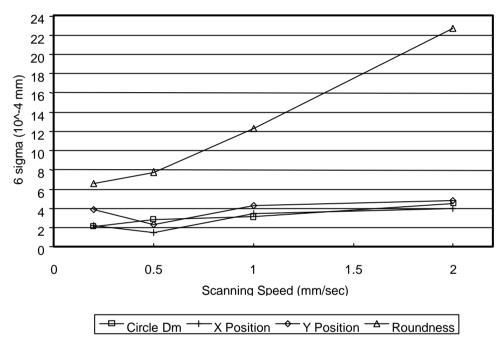
Figure 20-16 Circle features versus scanning speed
