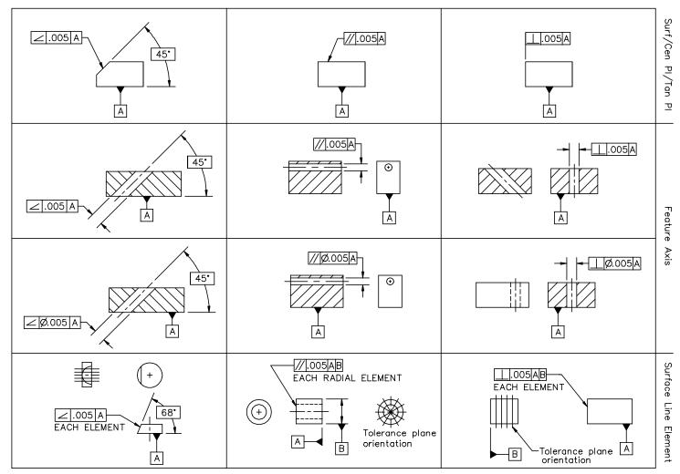
Figure 5-98 continued Applications of orientation tolerances
