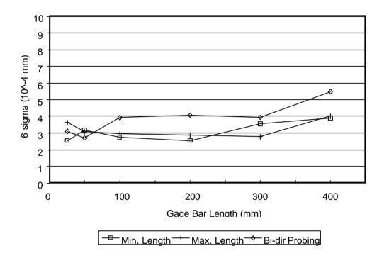
Figure 20-10a Bidirectional probing versus varying lengths (x-axis)
