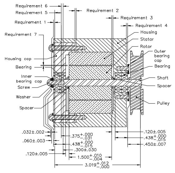
Figure 9-2 Motor assembly
