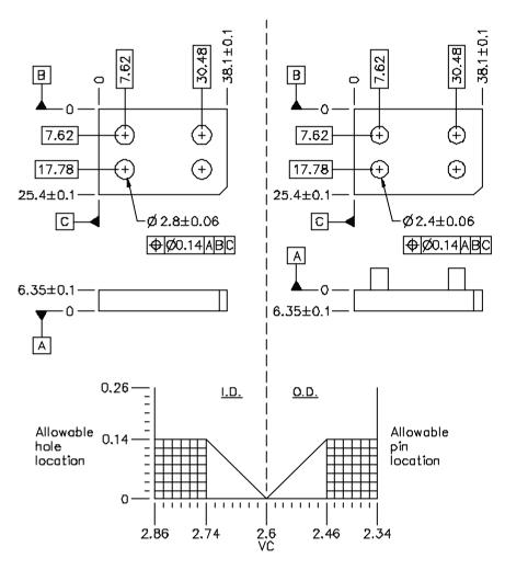
Figure 3-6 Tolerance stack-up graph (position at RFS)
