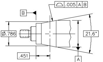
**Figure 5-140** Profile tolerancing to control a combination of characteristics
