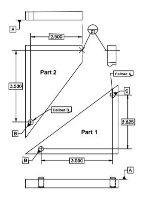
**Figure 24-11** Dimensioning methodology for two round pins with one hole and edge contact (only Type I shown)
