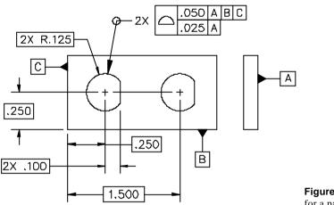
Figure 5-142 Composite profile for a pattern
