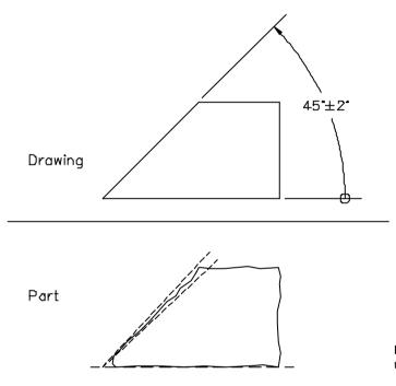
Figure 5-99 Erroneous wedge-shaped tolerance zone
