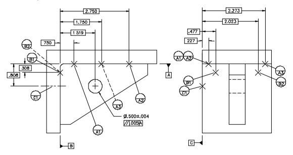
Figure 5-85 Datum target application on a rectangular part
