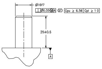
Figure 8-10 Illustration of statistical tolerancing under MMC
