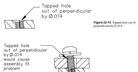
Figure 22-16 Variation in perpendicularity could cause assembly problems
