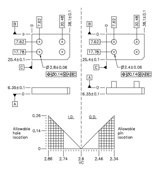
Figure 3-7 Tolerance stack-up graph (position at MMC)
