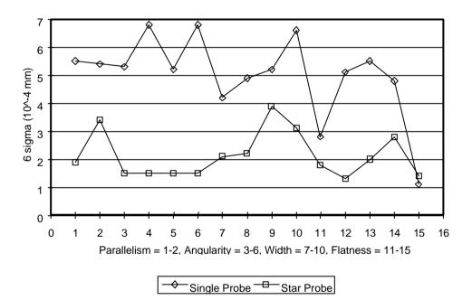
Figure 20-15 25-mm cube test—single versus star probe setup
