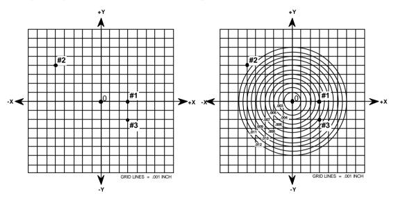
Figure 18-15 Verifying hole pattern prior to datum shift
