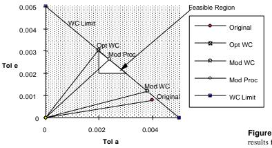
Figure 14-10 Tolerance allocation results for the modified WC Model
