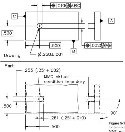
**Figure 5-112** Virtual condition boundaries for bidirectional positional tolerancing at MMC, rectangular coordinate system
