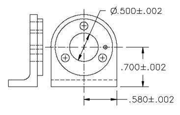
Figure 5-1 Drawing showing distance to ideal hole location
