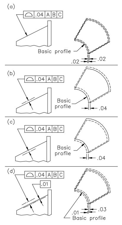
Figure 5-135 Profile tolerance zones
