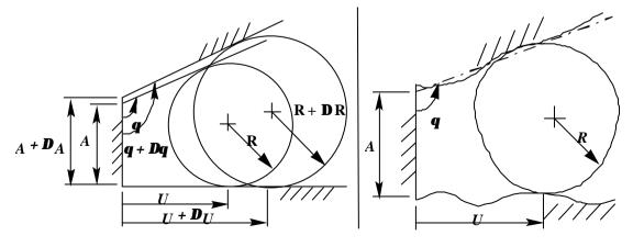
**Figure 13-1** Kinematic adjustment due to component dimension variations
