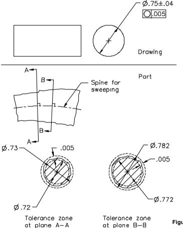
**Figure 5-42** Circularity tolerance (for nonspherical features)
