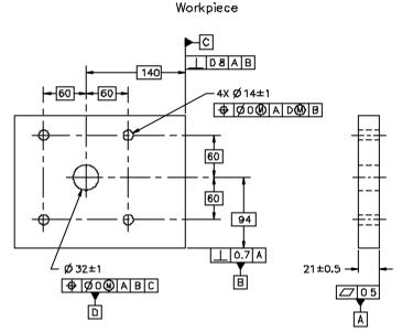
Figure 19-10 Multiple datum structures
