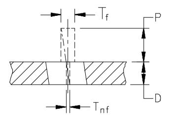
**Figure 22-18** Projected tolerance zone — location and orientation components
