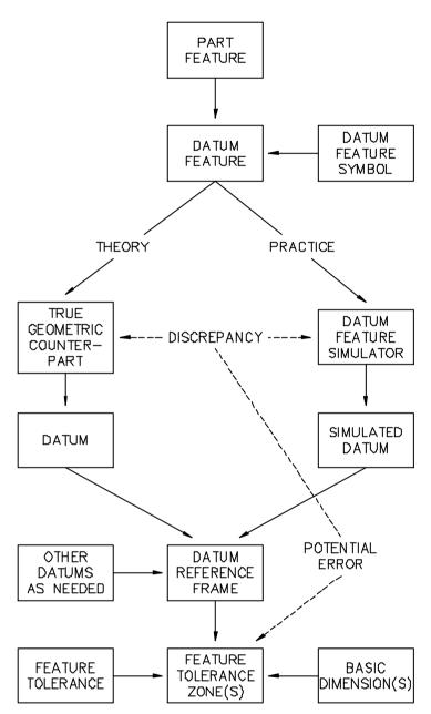
Figure 5-52 Establishing datum reference frames from part features
