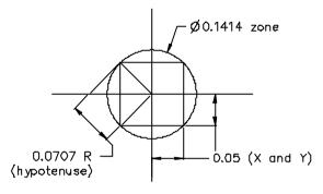
2 √∆X<sup>2</sup> +∆Y<sup>2</sup> = Ø tolerance zone 2 √0.05<sup>3</sup> + 0.05<sup>2</sup> = 2(0.0707)=0.1414 Ø tolerance zone Note: ±0.05 square zone = Ø zone of 0.1414 Note: Benefit of changing square zone to diameter tolerance zone is \*Increases position tolerance zone by 57 % \*Allows use of MMC principle
