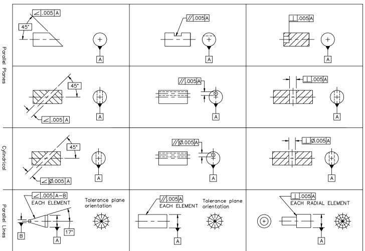
Figure 5-98 Applications of orientation tolerances
