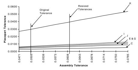
**Figure 9-9** Graph of piecepart tolerances versus assembly tolerance before and after resizing using the MRSS Model  $t_{kv,mrss,resized} = F_{mrss} t_{kv}$
