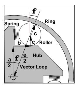
Figure 14-6 Clutch assembly with vector loop
