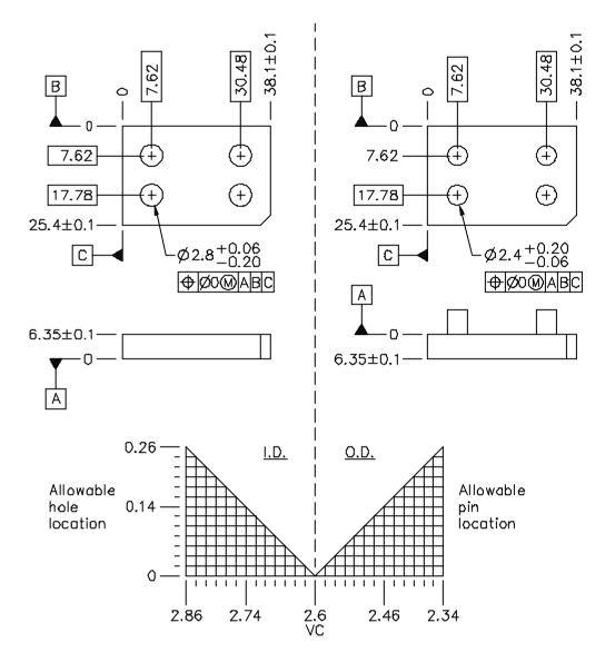
Figure 3-8 Tolerance stack-up graph (zero position at MMC)
