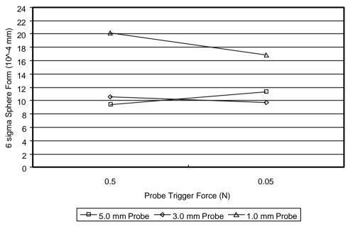
Figure 20-4 Sphere form versus probe trigger force (10-mm sphere)
