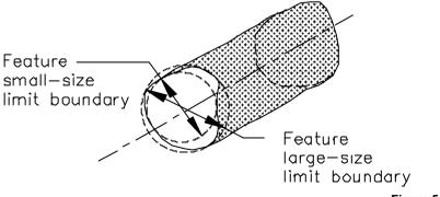
Figure 5-16 Size limit boundaries control circularity at each cross section
