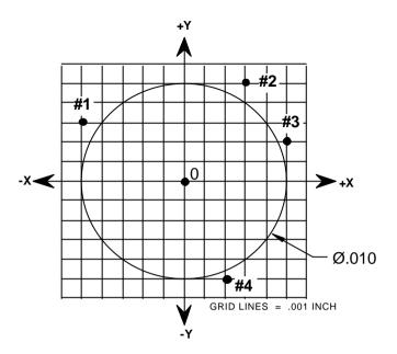
Figure 18-19 Verifying hole pattern prior to rotational shift
