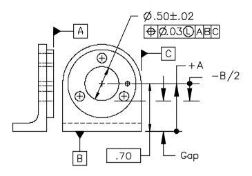
Figure 9-14 Position at LMC internal feature
