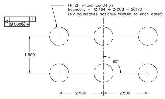
Note: All boundaries are oriented perpendicular to primary datum A. Figure 5-121 FRTZF virtual condition boundaries for Fig. 5-119
