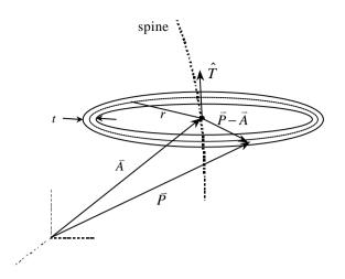
Figure 7-4 Circularity tolerance zone definition
