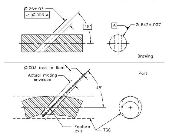
Figure 5-96 Applying an angularity tolerance to a cylindrical feature
