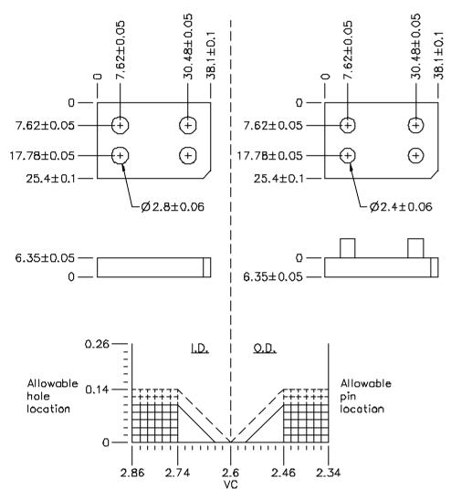
Figure 3-4 Tolerance stack-up graph (linear tolerancing)
