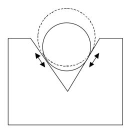
Figure 15-2 Small kinematic adjustments
