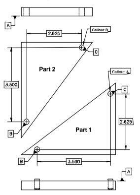
**Figure 24-6** Dimensioning methodology for two round pins with two holes (only Type I shown)
