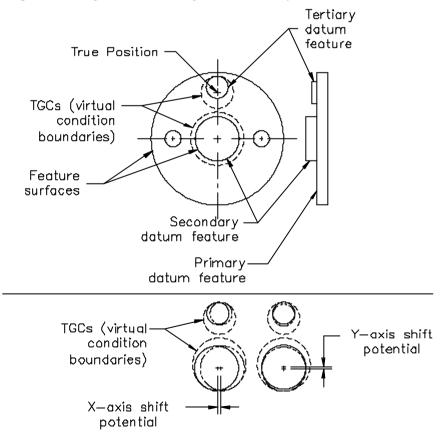
Figure 5-77 Unequal X and Y DRF displacement allowed by datum feature location variation
