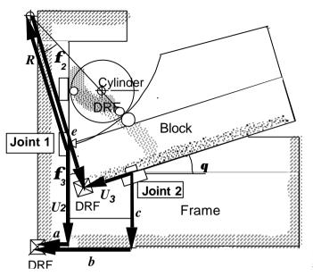
Figure 13-7 Datum paths for Joints 1 and 2
