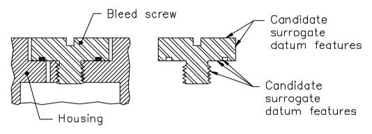
Figure 5-55 Selecting nonfunctional datum features
