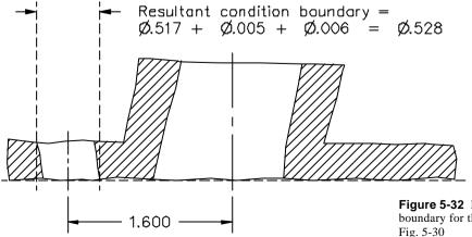
**Figure 5-32** Resultant condition boundary for the  $\emptyset$ .514 hole in Fig. 5-30
