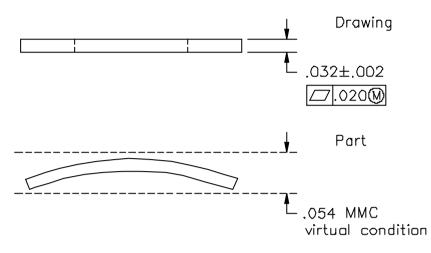
**Figure 5-27** MMC virtual condition of a width-type feature
