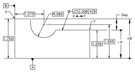
Figure 9-19 Equal bilateral tolerance profile
