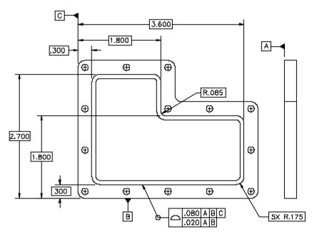
Figure 5-144 Composite profile tolerance for a single feature
