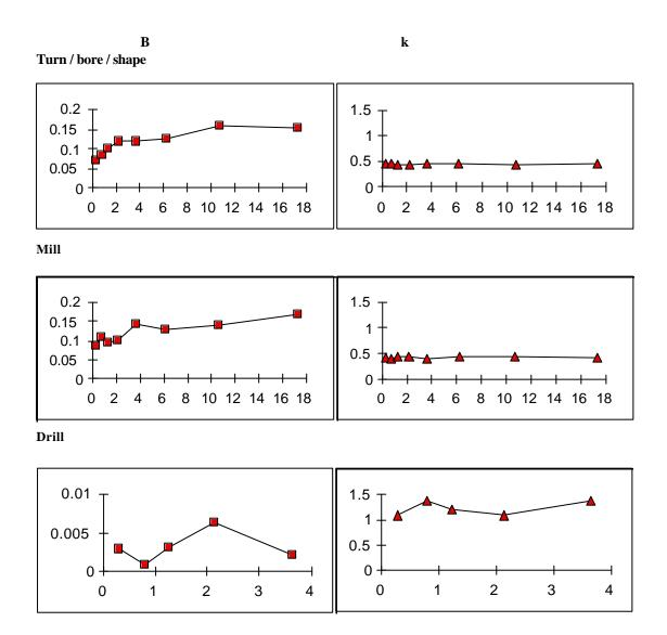
Figure 14A-3 continued Plot of coefficients versus size for cost-tolerance functions
