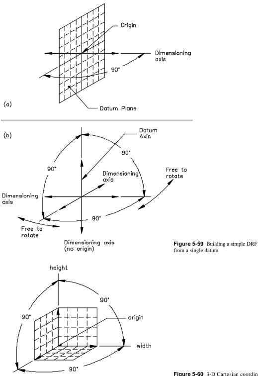
Figure 5-60 3-D Cartesian coordinate system
