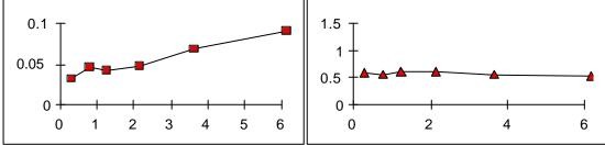
Figure 14A-3 Plot of coefficients versus size for cost-tolerance functions
