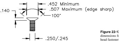
Figure 22-13 Flat head fastener dimensions for a .250-28-UNC 2B flat head fastener
