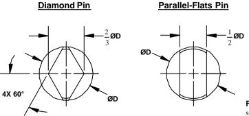
Figure 24-2 Two common crosssections for modified pins
