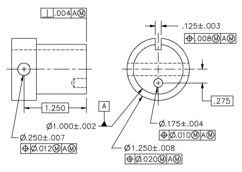
Figure 5-79 Using simultaneous requirements rule to tie together the boundaries of five features
