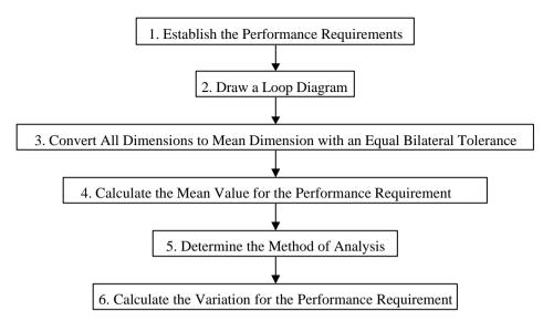
Figure 9-1 Tolerance analysis process
