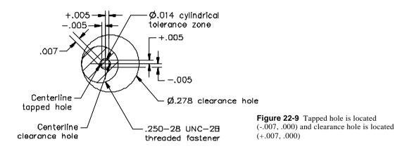
Allowing a tolerance of  $(\pm.007, .000)$  for the clearance hole and (-.007, .000) for the tapped hole, the tolerance zone is effectively a diametrical (cylindrical) tolerance zone of  $\emptyset$ .014. The use of a cylindrical tolerance zone is the preferred method because it allows all functional parts to be used. If a  $\pm.005$  tolerance zone had been used, this part would have been rejected (see Fig. 22-10).
