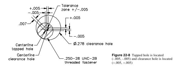
If the tapped holes and the clearance holes that are located by (+.005, -.005) are functional parts that have a .007 radial location, then a tapped hole manufactured at (-.007, .000) and the clearance hole manufactured at (+.007, .000) is also functional. Its tolerance zone also results in a .007 radial location (see Fig. 22-9). The resulting tolerance zone is a diameter .014.
