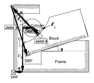
Figure 13-8 Datum paths for Joints 3 and 4
