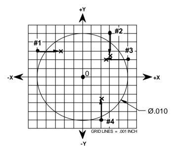
**Figure 18-20** Verifying hole pattern after rotational datum shift
