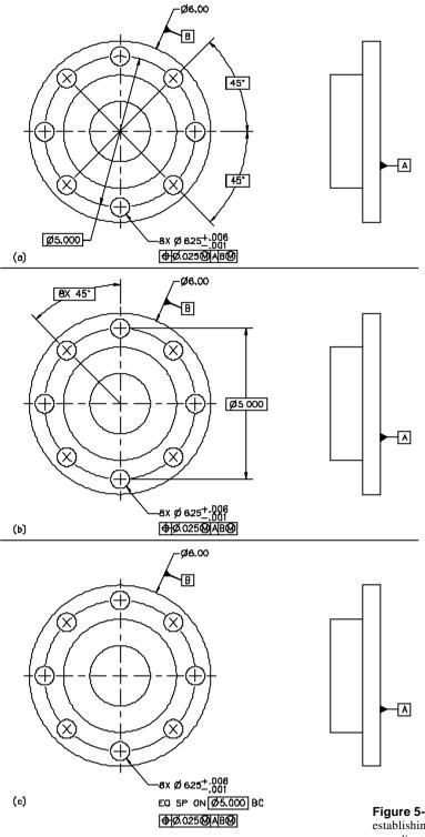
**Figure 5-102** Alternative methods for establishing true positions using coordinate dimensioning
