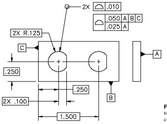
**Figure 5-143** Composite profile tolerancing with separate Level 2 control
