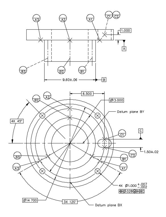
Figure 5-86 Datum target application on a cylindrical part
