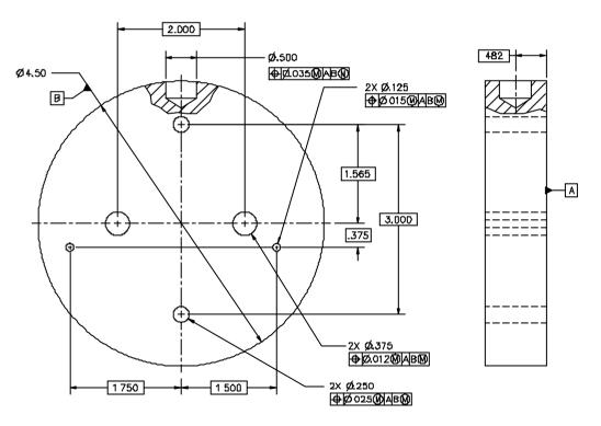
Figure 5-101 Methods for establishing true positions
