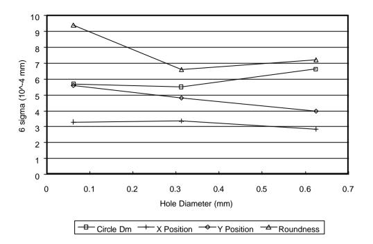
Figure 20-8 Circle features versus hole diameter
