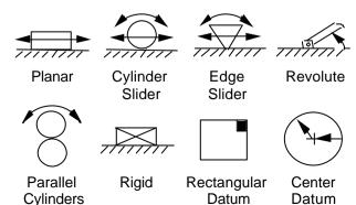
Figure 13-5 2-D kinematic joint and datum types
