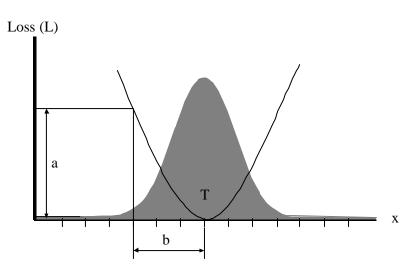
**Figure 1-1** Taguchi's loss function and a normal distribution
