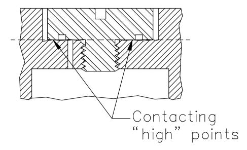
Figure 5-58 Parts contacting at high points
