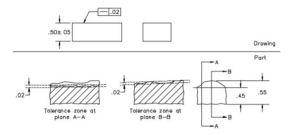
Figure 5-40 Straightness tolerance for line elements of a planar feature
