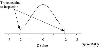
**Figure 11-8** Normal distribution that has been truncated due to inspection
