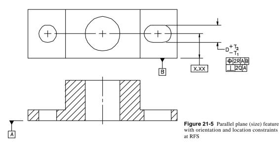
In this case, q is the orientation angle between the center plane of the feature and a plane orthogonal to datum A. If an internal feature is toleranced at MMC, or an external feature is toleranced at LMC,  $R - L^* \sin(q)/2$  is replaced by  $R_M$ . It is replaced by  $R_L$  when an internal feature is toleranced at LMC or an external feature is toleranced at MMC.
