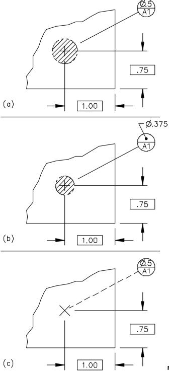
Figure 5-84 Datum target identification
