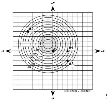
Figure 18-16 Verifying the hole pattern after datum shift
