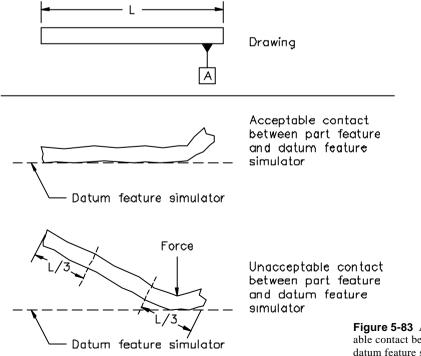
**Figure 5-83** Acceptable and unacceptable contact between datum feature and datum feature simulator
