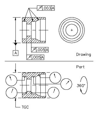
Figure 5-133 Application of circular runout
