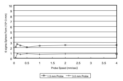
Figure 20-3 Probe speed versus sphere form
