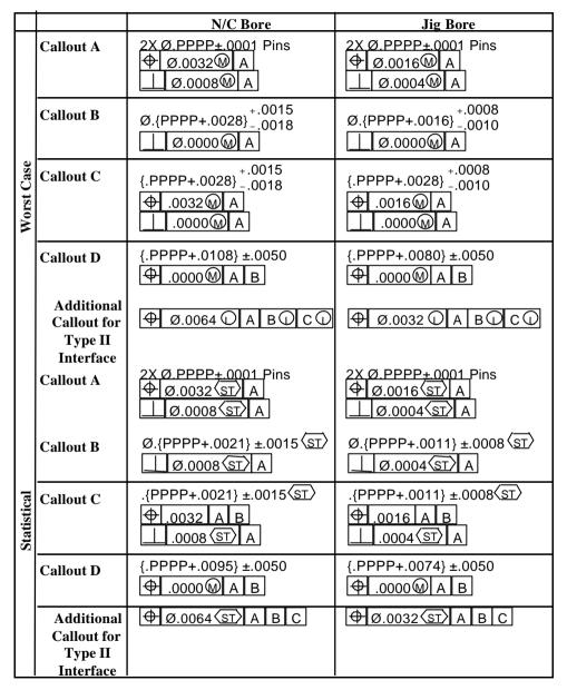
Table 24-6 GD&T callouts for two round pins with one hole and one slot
