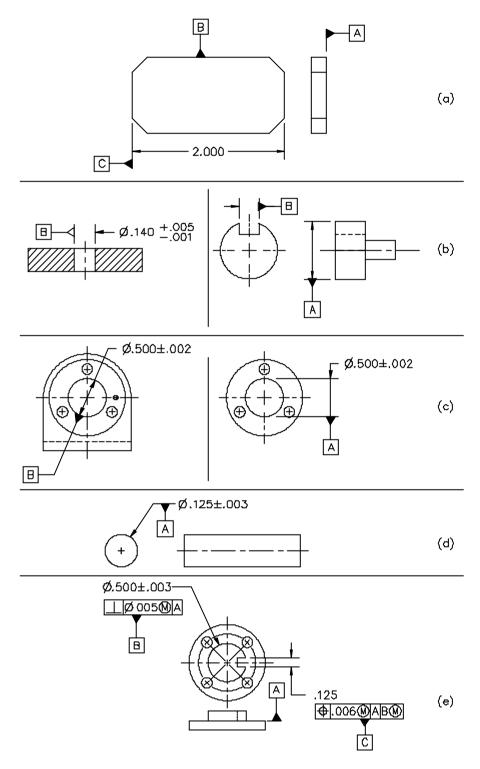
Figure 5-57 Methods of applying datum feature symbols
