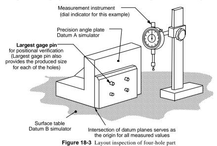
The pins placed in the holes aid the inspector when measuring the hole location. Actual "X" and "Y" measurements are made to the surface of the pin and as near to the part face as practicable. With the size of each pin known, adding 1/2 of the pin's diameter to the measured value will provide the total actual measurement to the center of each hole.
