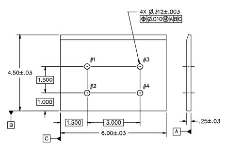
Figure 18-2 Example four-hole part
