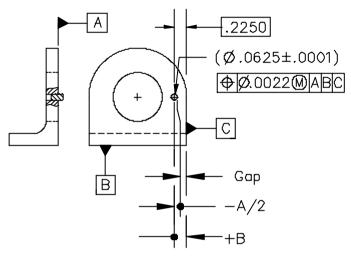
Figure 9-13 Position at MMC external feature
