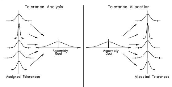
Figure 11-1 Comparison of tolerance analysis and tolerance allocation
