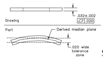
Figure 5-35 Tolerance zone for flatness control RFS
