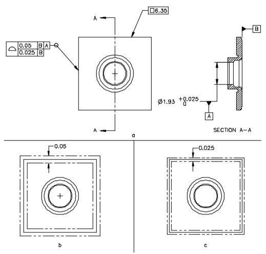
Figure 3-3 Fully geometric dimensioned and toleranced boundary example
