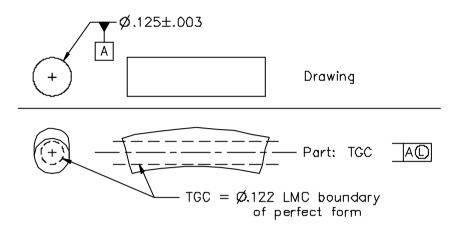
Figure 5-68 Feature of size referenced as a primary datum at LMC
