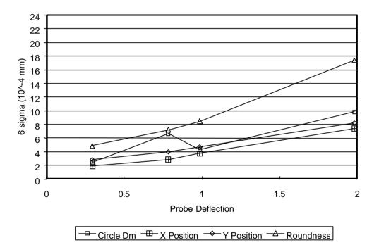
Figure 20-5 Circle features versus probe deflection
