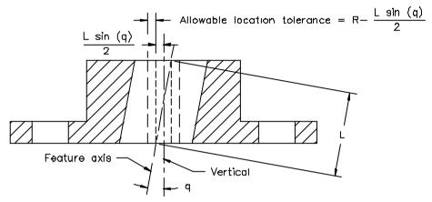
Figure 21-2 Allowable location tolerance as a function of orientation error (q)
