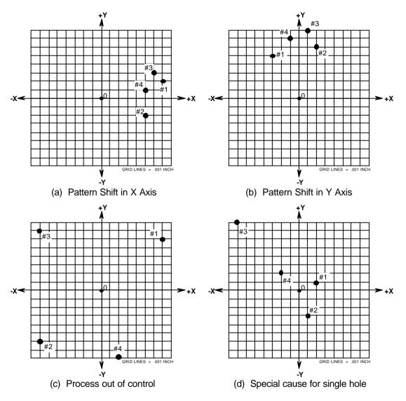
Figure 18-25 Process evaluation using a paper gage
