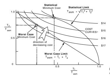
**Figure 14-2** Graphical interpretation of minimum cost tolerance allocation
