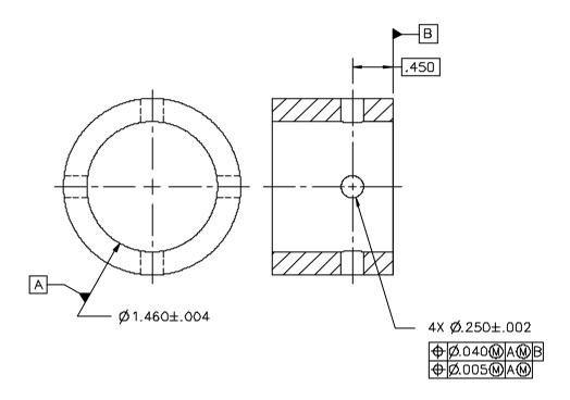
Figure 5-124 Two stacked single-segment feature control frames
