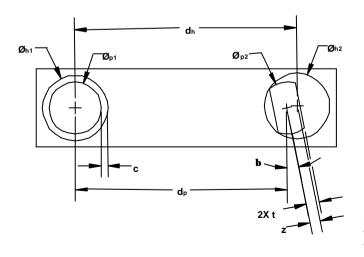
**Figure 24-13** Variables contributing to the fit of one pin and one parallel-flats pin with two holes
