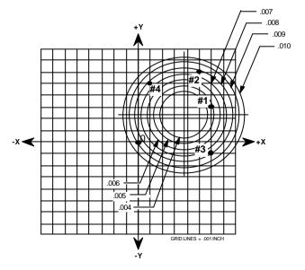
**Figure 18-10** Paper gage verification of feature-to-feature location
