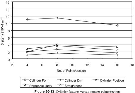
Figure 20-13 Cylinder features versus number points/section
