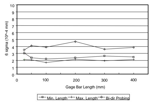
Figure 20-10b Bidirectional probing versus varying lengths (y-axis)
