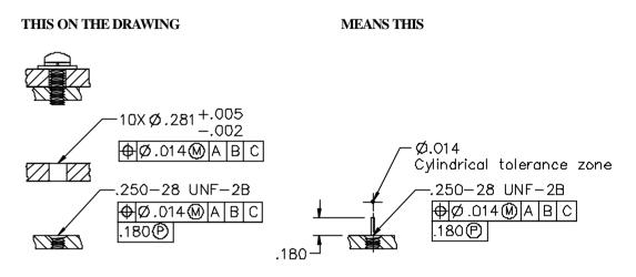
Figure 22-17 Projected tolerance zone example
