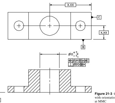
**Figure 21-3** Cylindrical (size) feature with orientation and location constraints at MMC
