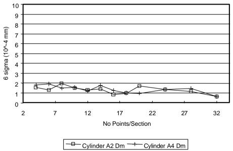
Figure 20-14 Cylinder features versus number of points/section
