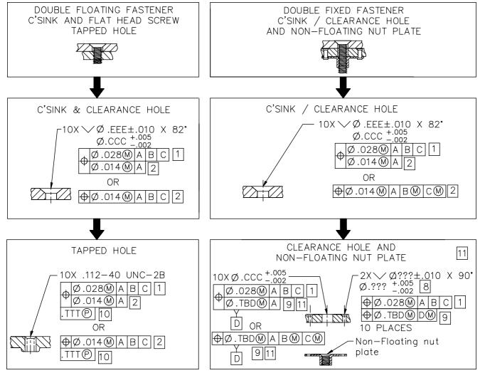
Figure 22-22 Double-fixed fastener tolerance and callouts
