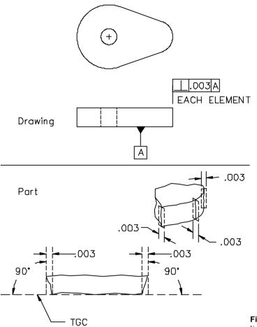
**Figure 5-97** Controlling orientation of line elements of a surface
