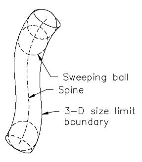
Figure 5-13 Generating a size limit boundary
