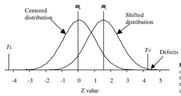
**Figure 11-5** Effect of shifting the mean of a normal distribution to the right.  $T_{i}$  is the lower tolerance limit,  $T_{u}$  the upper tolerance limit,  $\mathbf{m}_{i}$  is the unshifted mean, and  $\mathbf{m}_{i}$  is the shifted mean
