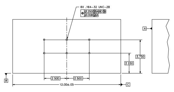
Figure 5-119 Avionics "black box" with composite positional tolerance on pattern of holes
