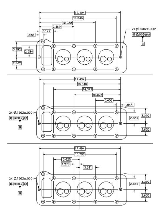
Figure 5-90 Three options for establishing the origin from a pattern of dowel holes
