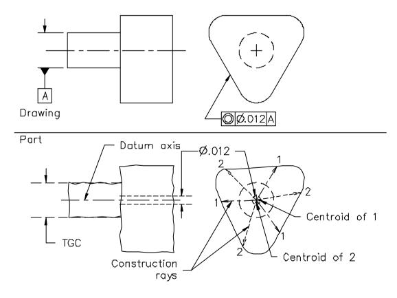
Figure 5-148 Multifold concentricity tolerance on a cam
