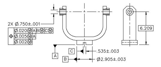
Figure 5-127 Three-segment composite feature control frame
