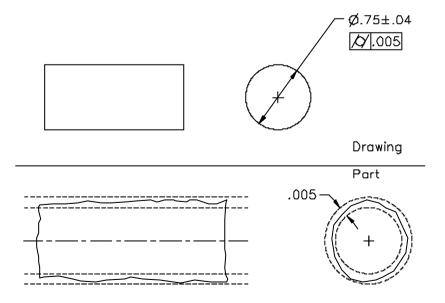
Figure 5-44 Cylindricity tolerance
