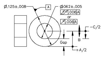
Figure 9-17 Circular and total runout
