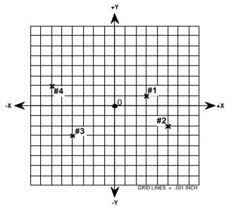
**Figure 18-4** Plotting the holes on the coordinate grid
