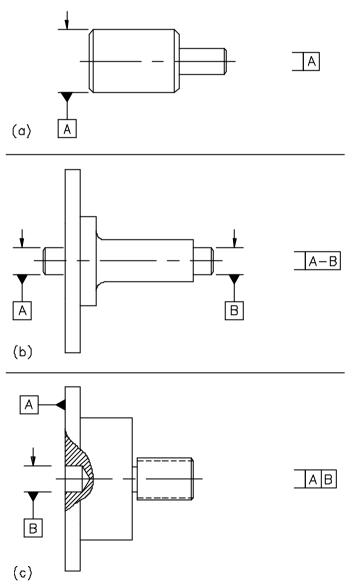
Figure 5-130 Datums for runout control
