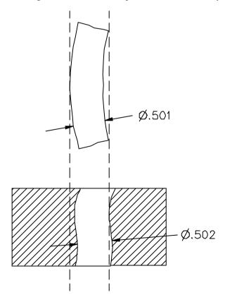
Figure 5-20 Level 1's size limit boundaries will not assure assemblability
