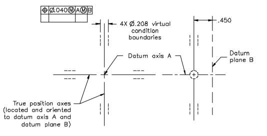
Figure 5-125 Virtual condition boundaries of the upper frame for Fig. 5-124
