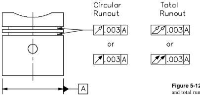
Figure 5-129 Symbols for circular runout and total runout
