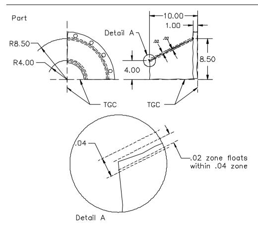
Figure 5-134 Application of profile tolerances
