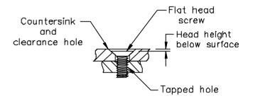
Figure 22-12 Worst case head height below the surface
