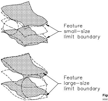
**Figure 5-15** Conformance to limits of size for a width-type feature
