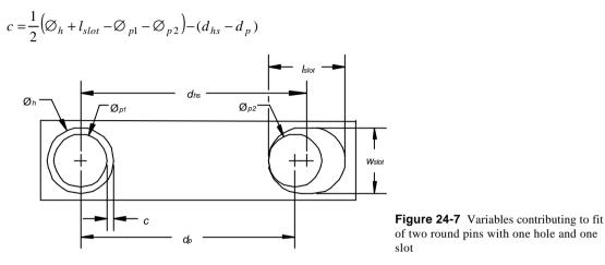
Since clearance in this direction is not critical, the callouts in Table 24-6 allow the slot width to vary by  $\pm$ .005. This tolerance is well beyond the Six Sigma capability but is not large enough to require excessive slotting of the hole.
