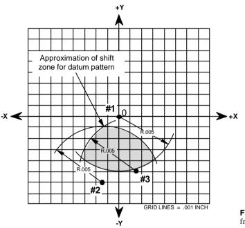
Figure 18-24 Approximating datum shift from a hole pattern
