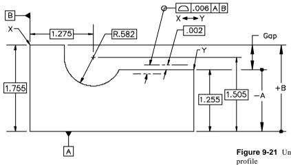
Figure 9-21 Unequal bilateral tolerance profile
