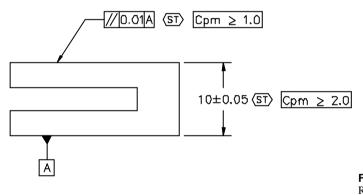
**Figure 8-2** Statistical tolerancing using RMS deviation index
