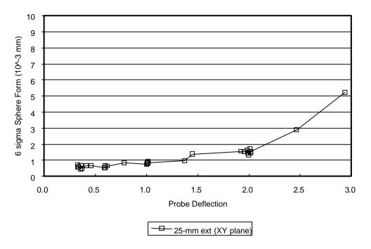
Figure 20-7 Probe deflection versus sphere form
