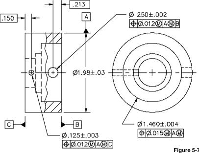
Figure 5-78 "Common DRF" means "identical DRF"
