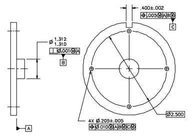
Figure 18-17 Part allowing rotational datum shift
