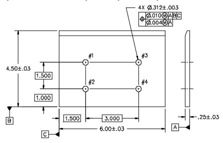
Figure 18-8 Four-hole part controlled by composite positional tolerancing
