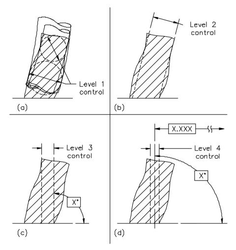
Figure 5-18 Levels of control for geometric tolerances modified to LMC
