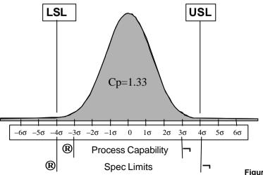
Figure 10-15 Capability index at  $\pm 4$  sigma
