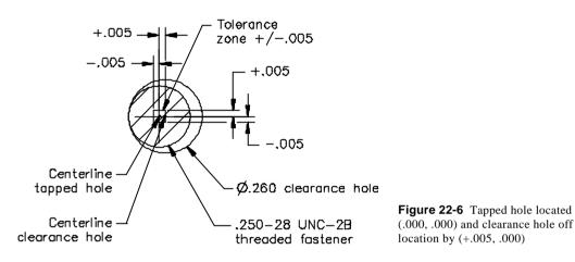
Let's assume the design engineer takes into account the allowable variation for both the clearance hole and the tapped hole. If the .250-28 UNF-2B tapped hole was located (-.005, .000) and the clearance hole was located (+.005, .000), the size of the clearance hole for this example would be .270 diameter ( $\emptyset$ .270). This would account for the possibility of a +.005 / -.005 shift of both the tapped hole and the clearance hole (see Fig. 22-7).
