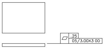
Figure 5-48 Flatness tolerance applied on a unit basis
