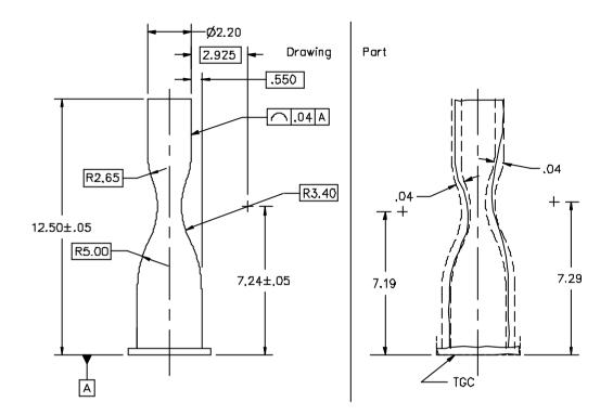
Figure 5-136 Profile of a line tolerance
