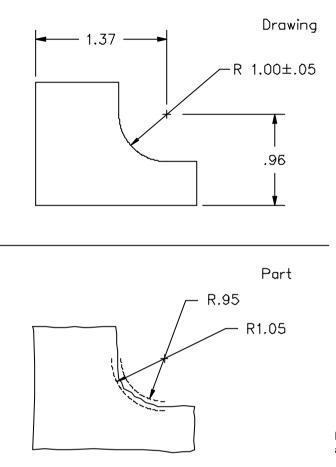
**Figure 5-50** Radius tolerance zone where a center is drawn
