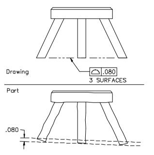
Figure 5-141 Profile tolerance to control coplanarity of three feet
