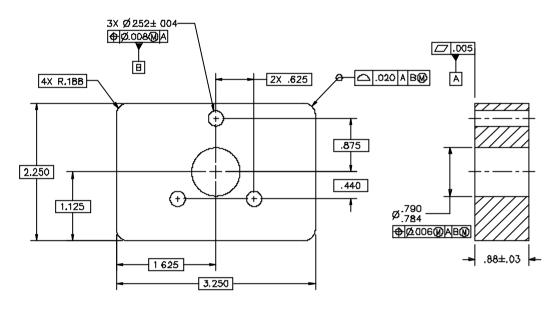
Figure 18-21 Example of datum established from a hole pattern
