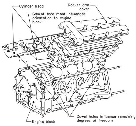
Figure 5-54 Establishing datums on an engine cylinder head
