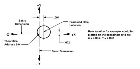
Figure 18-1 Directional indicators for data point plotting
