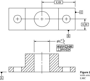
**Figure 21-4** Cylindrical (size) feature with orientation and location constraints at LMC
