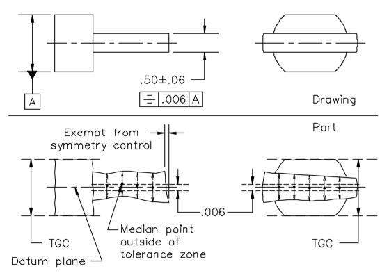
Figure 5-147 Symmetry tolerance about a datum plane
