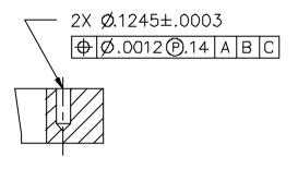
**Figure 5-107** Specifying a projected tolerance zone
