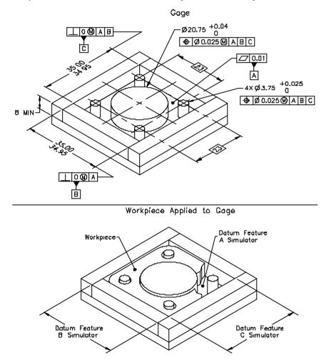
Figure 19-9 Gage for verifying four-hole pattern in Fig. 19-8
