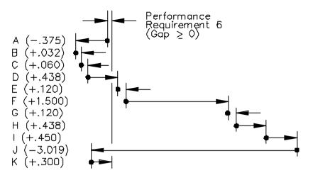
Figure 11-4 Dimension loop for Requirement 6
