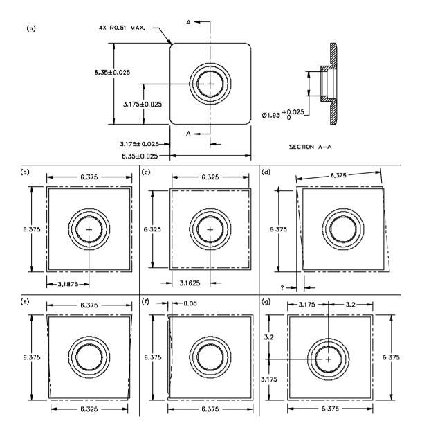
Figure 3-1 Linear dimensioning and tolerancing boundary example
