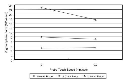
Figure 20-2b Sphere form versus probe settling time (25-mm sphere)
