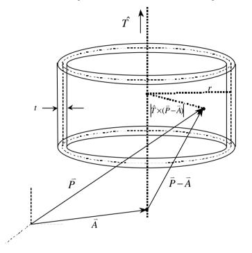
Figure 7-6 Cylindricity tolerance definition
