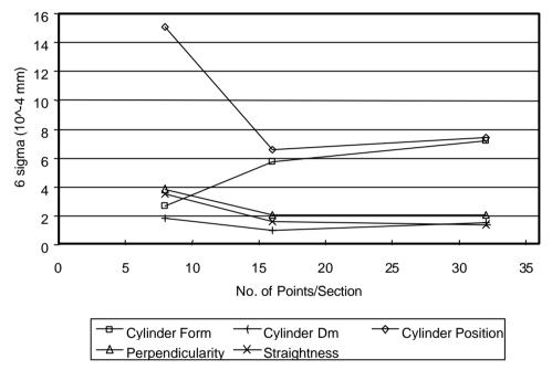
Figure 20-12 Cylinder features versus number of points/section
