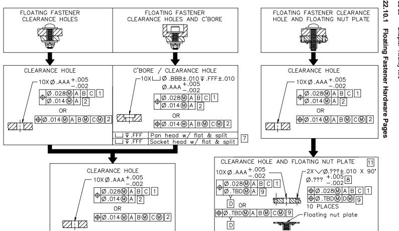
Figure 22-20 Floating fastener tolerance and callouts
