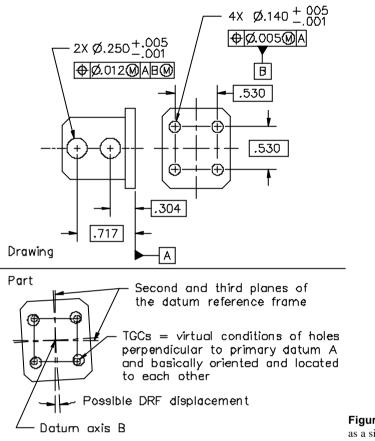
**Figure 5-91** Pattern of holes referenced as a single datum at MMC
