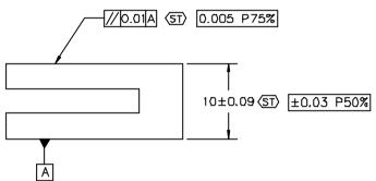
Figure 8-3 Statistical tolerancing using percent containment
