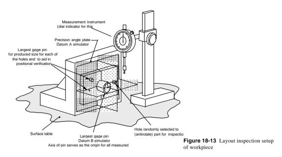
The amounts each hole deviated from the basic dimensions as defined by the engineering drawing are entered in the Inspection Report as "X" and "Y" deviations as shown in Fig. 18-14.
