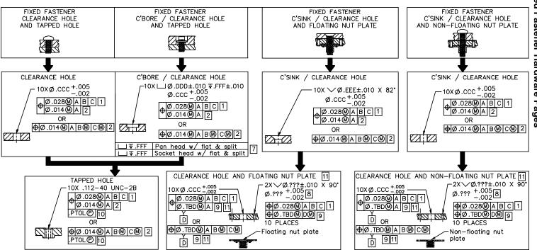
Figure 22-21 Fixed fastener tolerance and callouts
