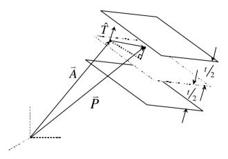
Figure 7-7 Flatness tolerance definition
