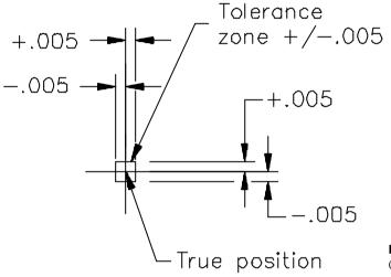
**Figure 22-4** Rectangular tolerance zone (plus/minus tolerancing)
