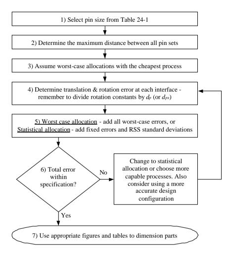
Figure 24-3 Design process for using alignment data
