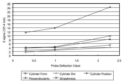
Figure 20-6 Cylinder features versus probe deflection
