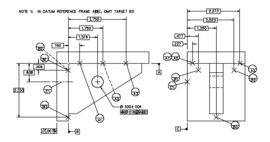
Figure 5-89 Target set with switchable datum precedence
