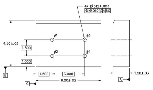
Figure 18-6 Example four-hole part with long holes
