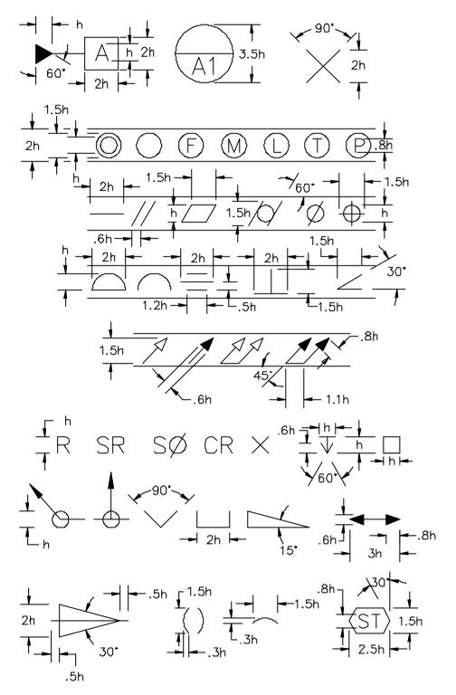
Figure 5-8 Symbols used in dimensioning and tolerancing
