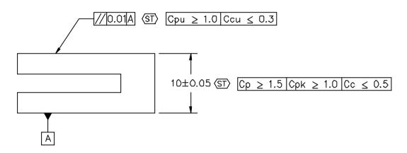
Figure 8-1 Statistical tolerancing using process capability indices
