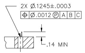
**Figure 5-108** Showing extent and direction of projected tolerance zone
