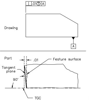
Figure 5-94 Application of tangent plane control
