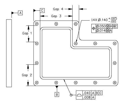
Figure 9-16 Composite position and composite profile
