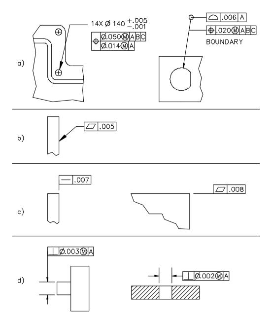
Figure 5-10 Methods of attaching feature control frames
