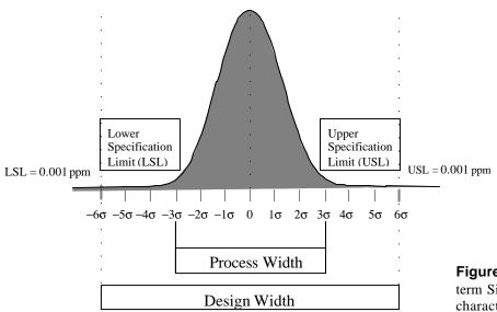
**Figure 1-2** Graphical definition of shortterm Six Sigma performance for a single characteristic
