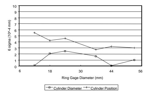
Figure 20-9 Cylinder features versus hole diameter
