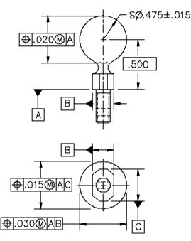
**Figure 5-111** Bidirectional positional tolerancing, rectangular coordinate system
