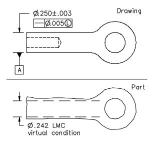
Figure 5-28 LMC virtual condition of a cylindrical feature
