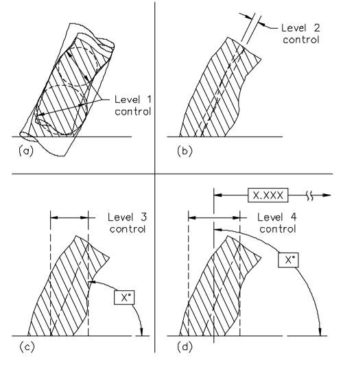
Figure 5-33 Levels of control for geometric tolerances applied RFS
