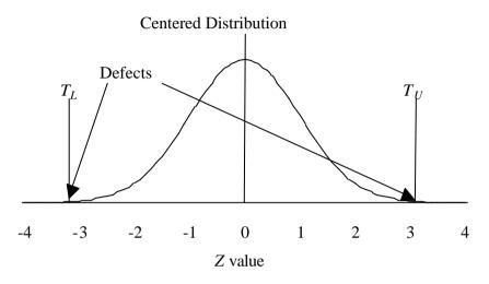
Figure 11-6 Centered normal distribution. Both tails are significant.
