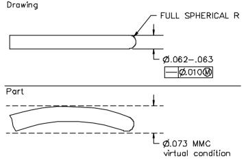
**Figure 5-26** MMC virtual condition of a cylindrical feature
