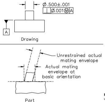
Figure 5-36 Example of restrained and unrestrained actual mating envelopes
