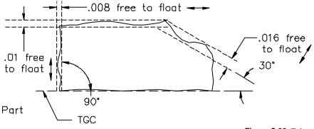
Figure 5-93 Tolerance zones for Fig. 5-92
