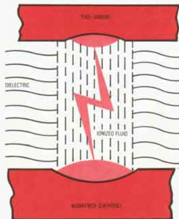
A controlled spark removes metal during electrical discharge machining
