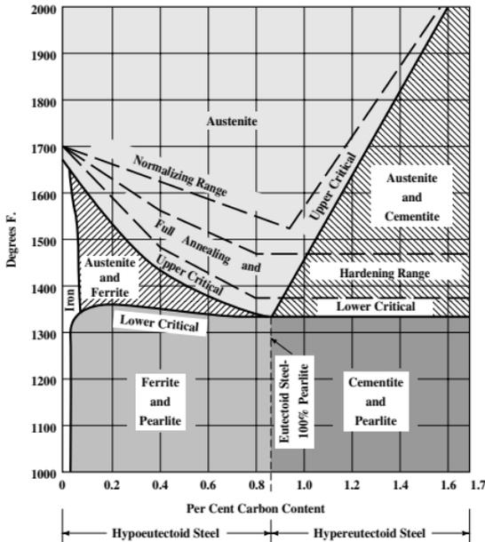
Fig. 1. Phase Diagram of Carbon Steel
