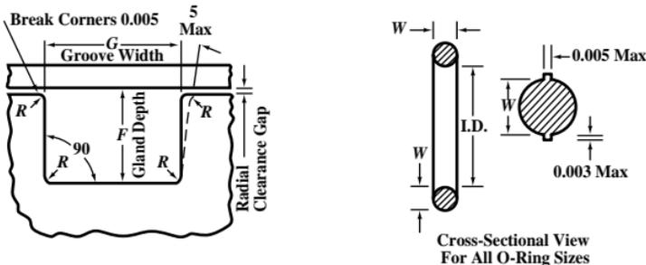
Fig. 2. Groove and Ring Details
