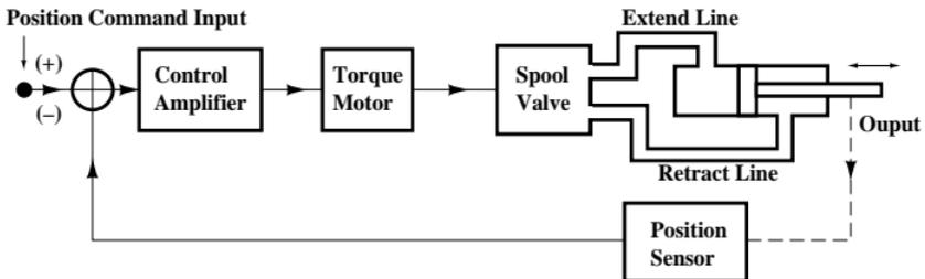
Fig. 6. A Pneumatic Closed-Loop Linear Control System
