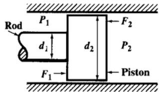
Fig. 1. Elementary Hydraulic Force/Area Formulas
