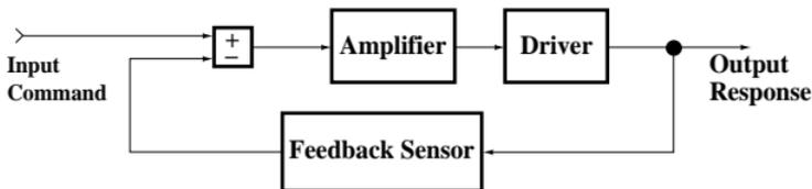
Fig. 1. General Arrangement of a Closed-Loop Control System
