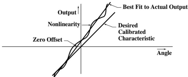
Fig. 3. Output Characteristics of a General Linear Position Transducer
