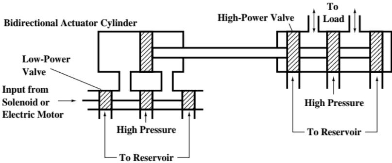
Fig. 5. Two-Stage Valve for Large-Power Control from a Low-Power Input
