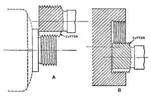
Examples of External and Internal Thread Milling with a Multiple Thread Milling Cutter
