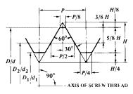
Fig. 1. Basic Profile of ISO Metric Thread
