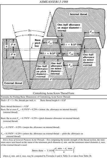
Shear Area of General Purpose Acme Threads. For computing the shear area per inch length of engagement of the external thread, the maximum minor diameter of the internal thread  $D_1$  max., and the minimum pitch diameter of the external thread  $D_2$  min. Table 2b or Formulas 12 and 4, Table 2a, are used:
