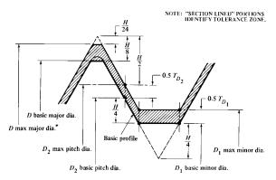
Fig. 7. Internal Thread - Limiting M Profile. Tolerance Position H
