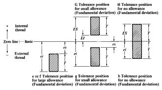
Fig. 6. Metric Tolerance System for Screw Threads
