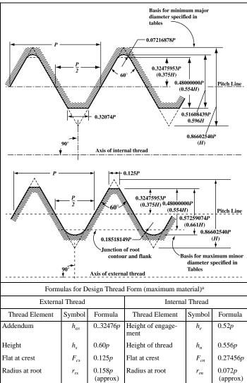
Table 2. Unified Miniature Screw Threads - Design Thread Form
