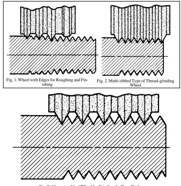
Fig. 3. Alternate-ribbed Wheel for Grinding the Finer Pitches **Multi-ribbed Wheels.**—This type of wheel is employed when rapid production is more important than extreme accuracy, which means that it is intended primarily for the grind-
