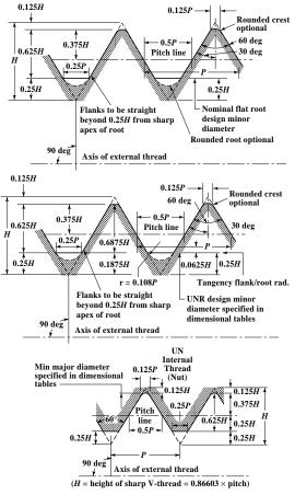
*Thread Series:* Thread series are groups of diameter-pitch combinations distinguished from each other by the numbers of threads per inch applied to a specific diameter. The various diameter-pitch combinations of eleven standard series are shown in Table 2. The limits of size of threads in the eleven standard series together with certain selected combinations of diameter and pitch, as well as the symbols for designating the various threads, are given in Table 3.
