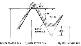
Fig. 2. Internal Thread Design M Profile with No Allowance (Fundamental Deviation) (Maximum Material Condition). For Dimensions see Table 3
