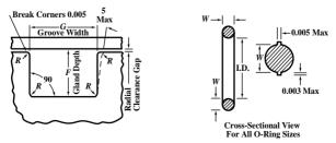
Fig. 2. Groove and Ring Details
