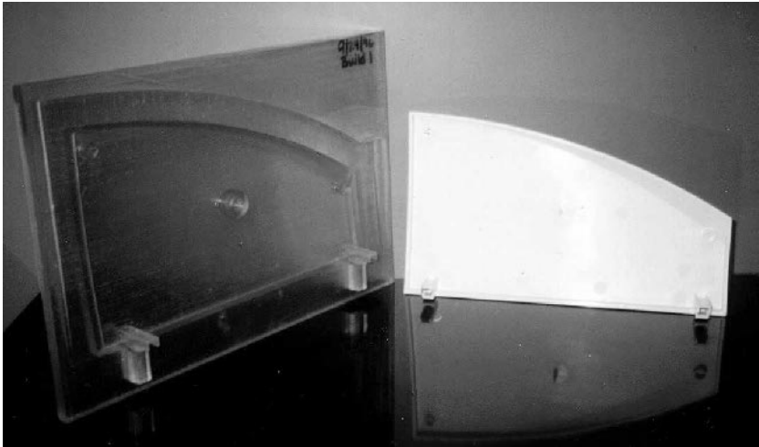
Figure 12 A SIMPLE tool SL mandrel of appearance part (left), shown opposite a molded part (right) to show relationship. (SL mandrel supplied by 3D Systems.)
