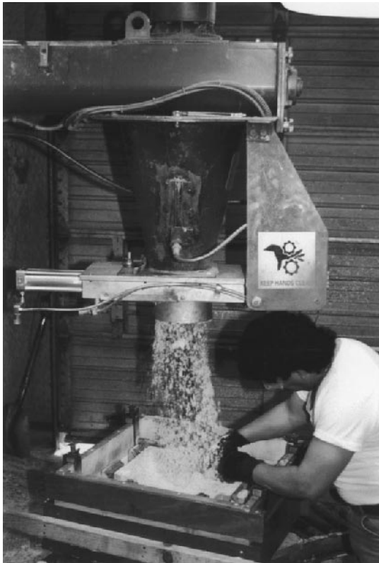
Figure 9 Precision sand-casting mold formation.
