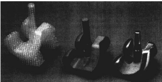
Fig. 21 Left-to-right: QuickCast pattern, raw casting, finished product.
