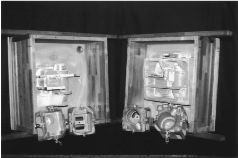
Figure 10 Rapid tooling for precision sand casting, including the cope and drag plate and associated core boxes.
