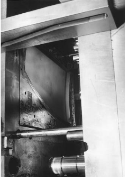
Figure 13 Appearance part tool in press. The textured side of the mold is on the left. Reverse ejection with slide action features are shown on the right.
