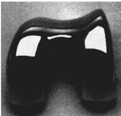
Fig. 7 Complex geometry of femoral component for knee replacement system.
