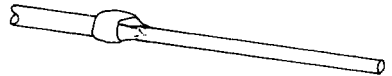
(d) Reduce filler wire by grinding if necessary; see next paragraph 'Welding fine details'
