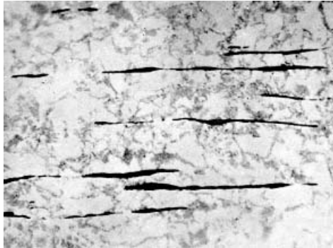
Figure 17.31 Microstructure of a lamellar-tearing susceptible steel. From Dickinson and Nichols (51).
