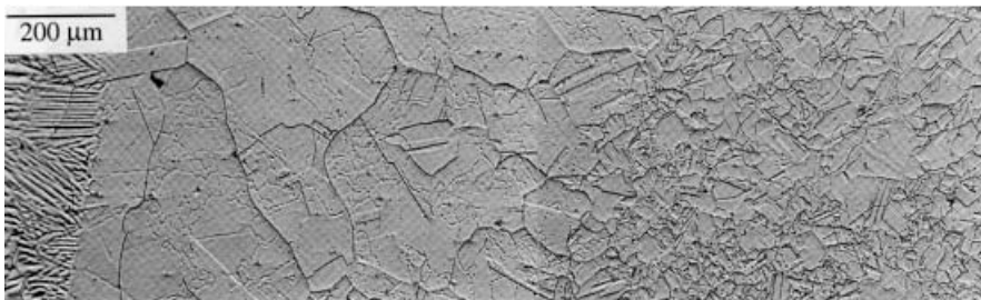
Figure 12.9 Ghost GBs near fusion boundary of gas-tungsten arc welds: (a) 18-Ni maraging steel; magnification 125 \times . Reprinted from Pepe and Savage (6). Courtesy of American Welding Society. (b) Ni-base superalloy 690. Reprinted from Lee and Kuo (14).
