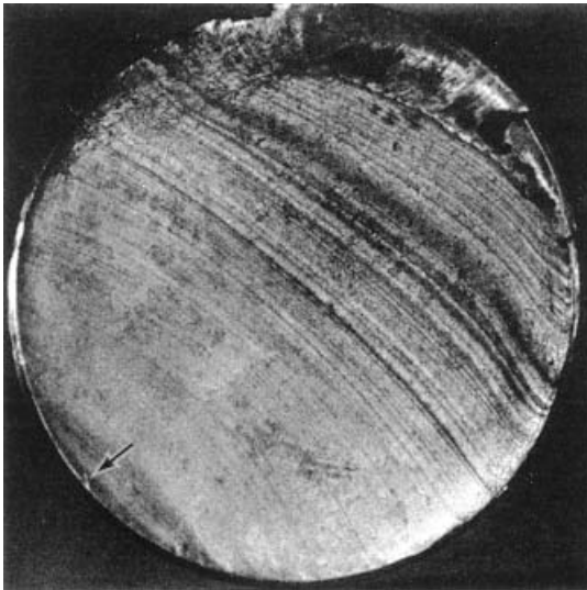
Figure 5.14 Fatigue fracture surface showing beach marks and origin of fracture. Reprinted, with permission, from Wulpi (12).
