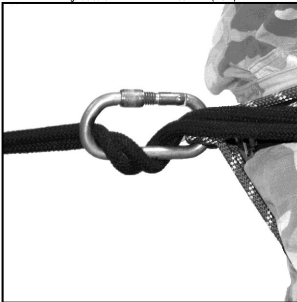
Figure 9-30. CARABINER WRAP DESCENDER (INSET)
