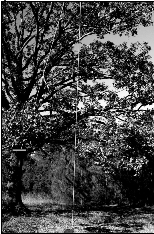
Figure 4-1. FIELD EXPEDIENT, END-FED QUARTER, HALF, OR FULL WAVE ANTENNA
