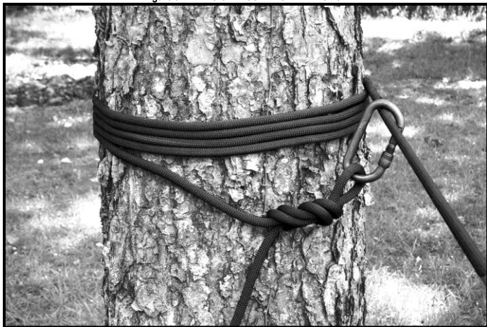
Figure 9-4. TENSIONLESS NATURAL ANCHOR
