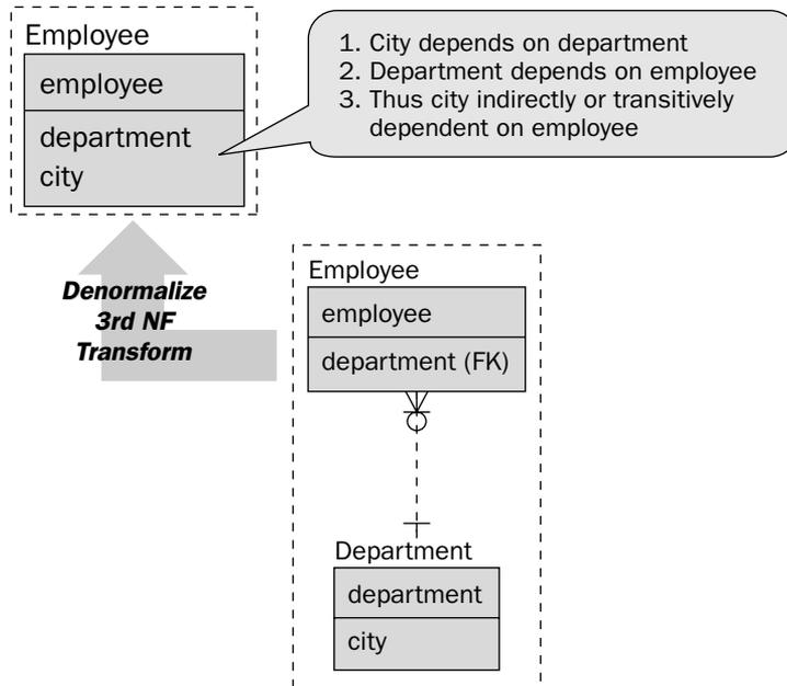
Figure 6-9: Denormalization of 3NF transitive dependence resolution table.
