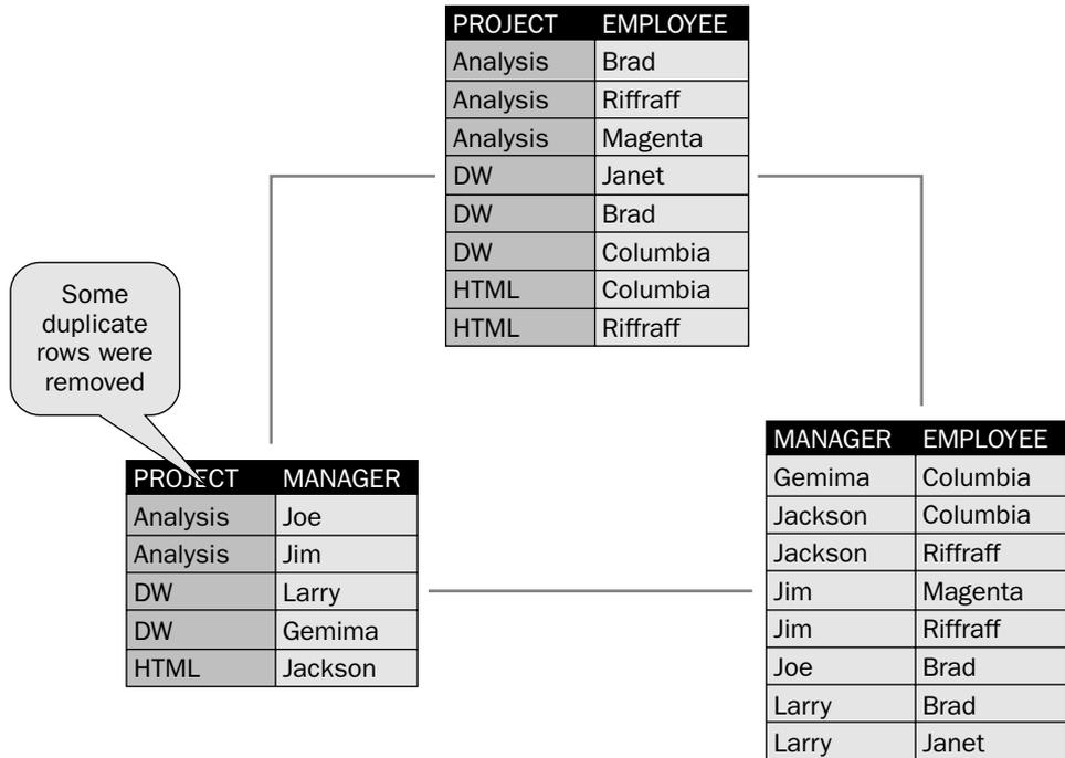
Figure 4-43: 5NF transformations sometimes remove duplicates.
