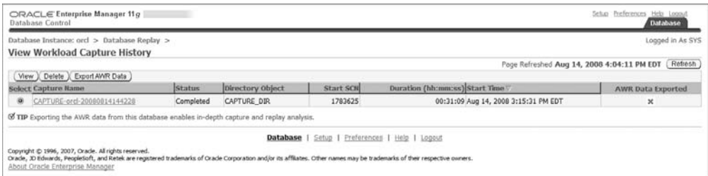
FIGURE 10.55 The View Workload Capture History screen
