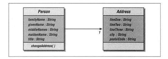
Figure 8-3. The object model supporting a simple address book application
