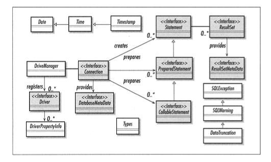
Figure 14-1. The classes and interfaces of the JDBC API
