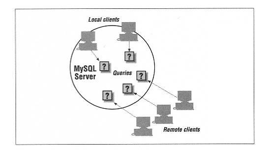
Figure 4-1. The client/sever design of MySQL
