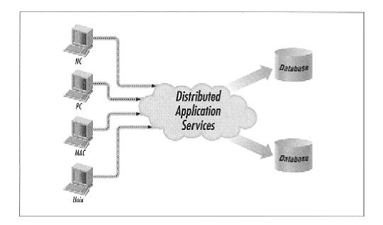
Figure 8-4. Three-tier architecture
