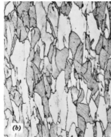
particular deformation, the grains become elongated along the direction in which the specimen was extended.
