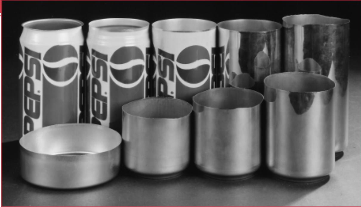
**T**his photograph shows the aluminum beverage can in various stages of production. The can is formed from a single sheet of an aluminum alloy. Production operations include drawing, dome forming, trimming, cleaning, decorating, and neck and flange forming. (PEPSI is a registered trademark of PepsiCo, Inc. Used by permission.)
