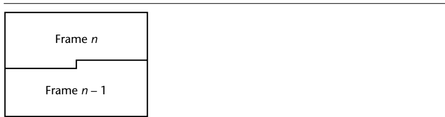
Figure 10.3 Tearing results when there is only one frame buffer or when rendering and refresh cycles are unsynchronized, resulting in simultaneous display of two partial frames.
