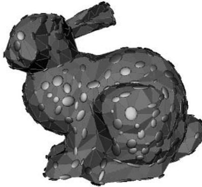
Figure 3.12 Ellipsoids (level surfaces of error quadrics) illustrate the orientation and size of the error quadrics associated with a simplified bunny [Garland 97]. Copyright © 1997 Association for Computing Machinery, Inc.
