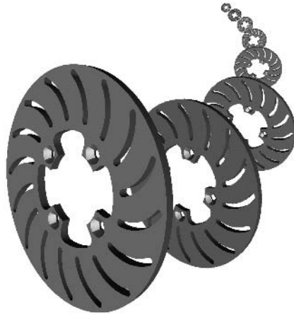
Figure 2.18 A topology-preserving LOD hierarchy for a rotor from a brake assembly [Cohen 96]. Copyright © 1996 Association for Computing Machinery, Inc.
