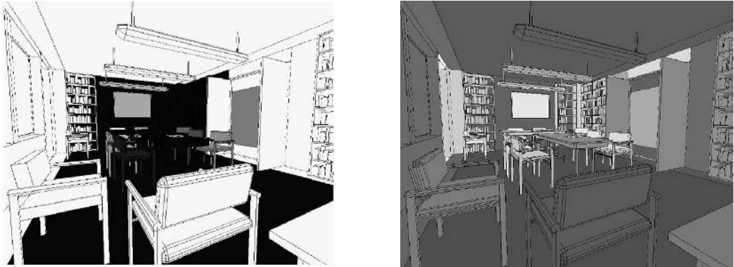
Figure 8.1 Images of Funkhouser’s architectural walk-through system showing the relative benefit of objects where the focus (eccentricity) factor is set to (a) 1.0 and (b) 0.01. Darker grayscales represent higher benefit values [Funkhouser 93a].
