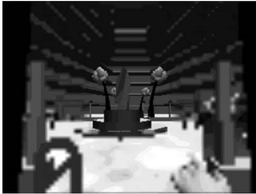
Figure 9.8 Display with reduced fidelity in the periphery as used in [Watson 97d].
