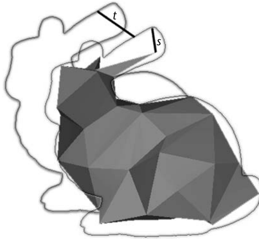
Figure 10.27 IO differencing to manage the tradeoff of visual and temporal detail. The full-detail model positioned according to latest input is silhouetted at the lower right. Rendering that model (silhouetted upper left) introduces a temporal error t . Rendering a coarse approximation (shown in polygonal form) introduces spatial error s , but eliminates t . In this case temporal error is dominant—we should render the coarse model.
