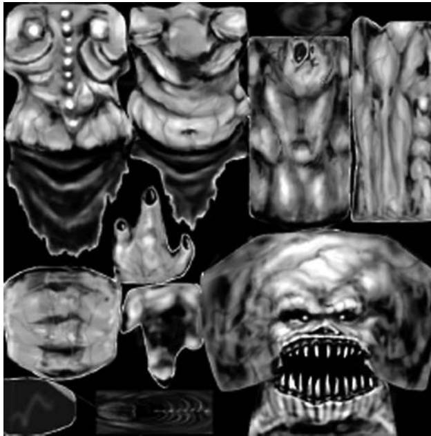
Figure 6.3 Texture compositing optimizes texture memory by creating a single texture map of a number of subtextures.
