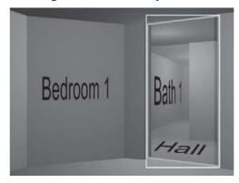
Figure 16.13: The bounding box of a portal polygon
