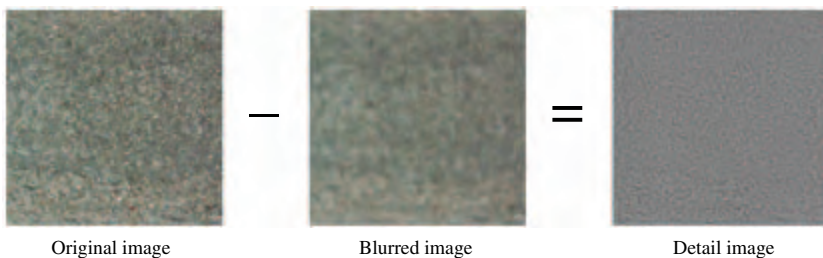
Figure 14.27 Subtracting out low frequencies.
