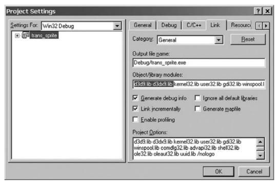
Figure 8.2 Adding support for Direct3D to the project
