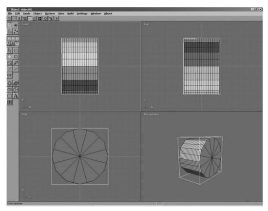
Figure 12.33 The wheel mesh has been subdivided and is now more detailed.
