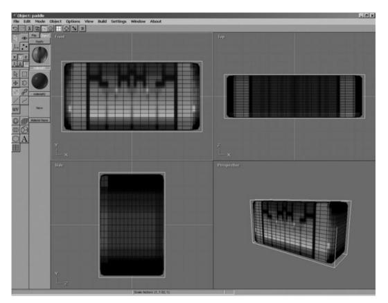
Figure 14.11 The paddle is a subdivided rectangular solid that was "smithed" into the desired shape.
