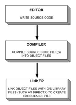
**Figure 1.3** The compilation process takes a source code file, compiles it, then links it into an executable.
