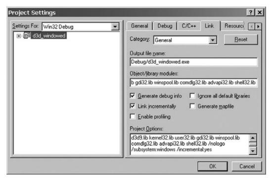
Figure 5.2 Opening the Link tab in the Project Settings dialog
