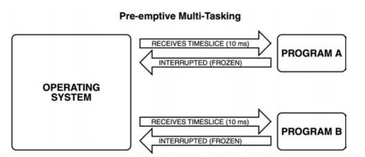
**Figure 1.6** A pre-emptive multi-tasking O/S has full control over the system and allocates slices of time for each running process and thread.
