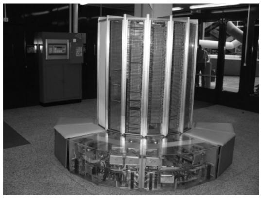
**Figure 9.7** Cray-1 supercomputer, circa 1976–1980.
