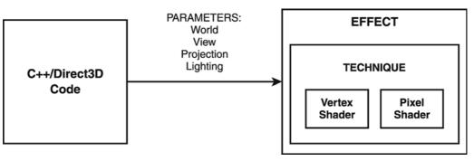
Parameters define how shader functions will manipulate vertices and render pixels.
