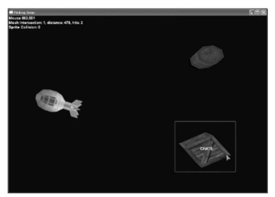
Figure 17.1 A ray is fired from the mouse cursor position to test for mesh collisions.
