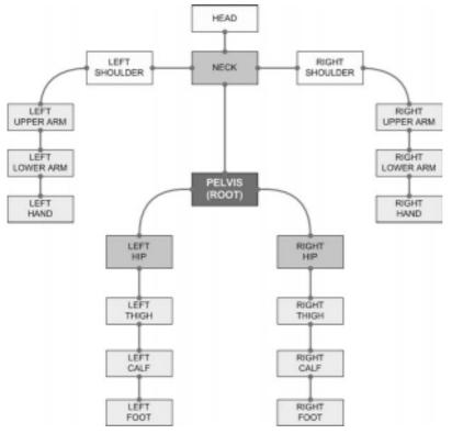
An illustration of the hierarchical structure of a biped character, showing the root and first three high-level nodes (Neck, Left Hip, Right Hip).
