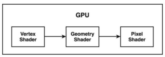
A GPU that supports DirectX 10 and later will also have a geometry shader.
