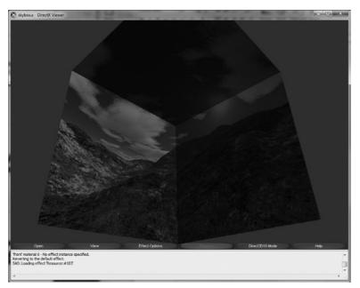
Figure 11.2 Note how the inverse normals cause the faces to reflect light from *inside* the skybox.
