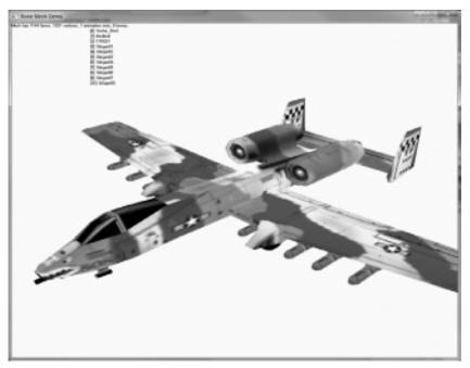
A non-hierarchical mesh may still have many frames containing sub-meshes, such as the detachable missiles on this "USAF A-10 Thunderbolt II" aircraft.
