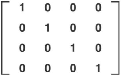
Figure 7.7 An identity matrix is used to reset transformations.
