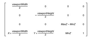
Working backwards, transforming a world space point W(X, Y, Z) by the viewport transformation matrix, yields the screen space point S(X, Y). Following are the two equations to solve for S. The 2D image displayed by your graphics card after rasterization does not contain any depth information (Z).
