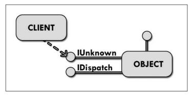
Figure 32.1 Communication between a client and a COM component.
