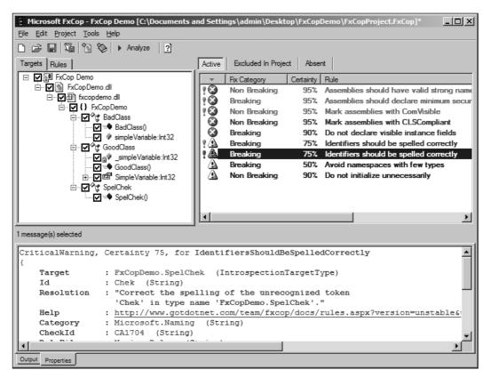
Figure 13.4 Screen capture of the FxCop tool after analysis has been performed.
