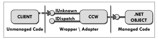
Figure 32.2 Communication between a client and a .NET object through a COM Callable Wrapper.
