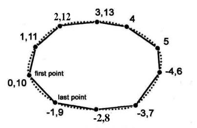
FIGURE 2.6.1 *Replicating points for a closed spline.*
