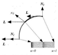
**FIGURE 5.2.1** In this figure Nj, N<sub>2</sub>, **#WN**<sub>3</sub> are the normal vectors at the surface. L represents the directional light vector. Note that when N<sub>1</sub> • L=0, where i= 1, we are at u=0 in the texture; when N<sub>1</sub> • L=.5, i=2, the transition point or hard boundary in the texture occurs. This is when the transition occurs between the highlight and shadow color. Finally, when N<sub>1</sub> • L=l, n=3 and the texture coordinate i=i reached.
