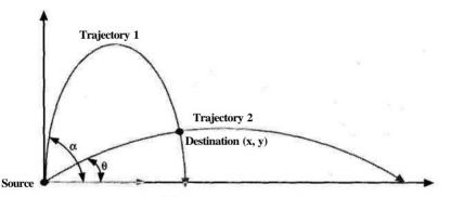
FIGURE 2.4.2 Two angle of elevation solutions OC and § for a given Vj.
