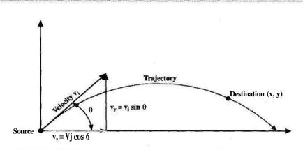
FIGURE 2.4.1 Trajectory between two points in two dimensions.
