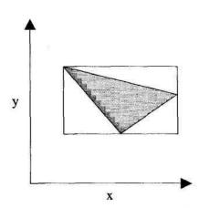
FIGURE 4.4.1 The sides of an AABB are parallel to the coordinate axes.
