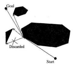
FIGURE 3.10.2 The path must go around each corner.
