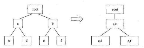
FIGURE 4.4.5 For a set of four triangles, the uncompressed tree requires seven nodes, whereas the tree on the right requires onlyfour.
