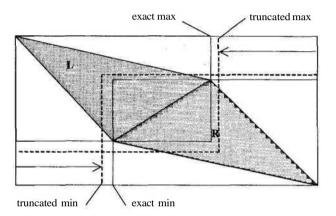
**FIGURE 4.4.3** When approximating extents with unsigned 8-bit integers, min values are measured from the left, while max values are measured from the right.
