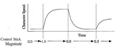
FIGURE 4.11.4 Character speed based on controller input with exponential dampening.
