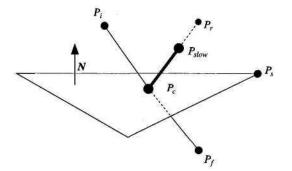
FIGURE 2.2.6 Calculating a damped reflection vector.
