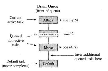
FIGURE 3.4.1 An AItask list in the form of a brain queue.
