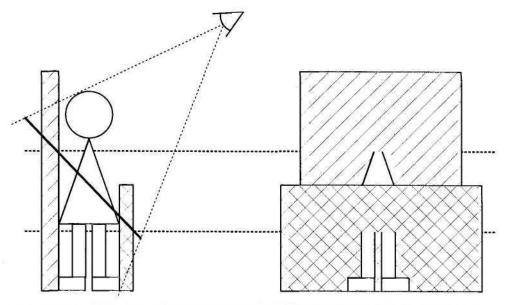
FIGURE 5.7.1 Side view and rendered view of a billboard impostor showing Z-buffer problems.
