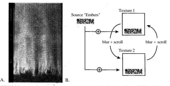
FIGURE 5.8.2 Fire and smoke animation using Listing 5.8.1 s offiets A with a scroll offset. The bright "embers" at the bottom are rendered to the texture each frame before blurring and scrolling upward. B) shows the progression of rendering operations.
