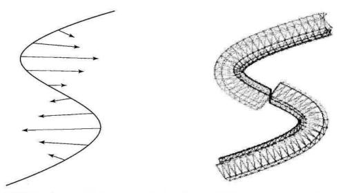
**FIGURE 2.5.2** Second derivative on an S-shaped curve, and Frenet Frame generated tube from the same curve.
