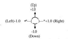
FIGURE 4.11.2 Values from an analog controller.
