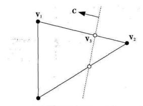
FIGURE 4.8.2 Clipping a polygon against a plane.
