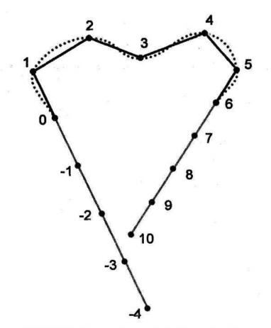
FIGURE 2.6.2 Creating phantom points for an open spline.
