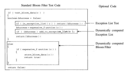
FIGURE 1.20.3 Bloom Filter configurations.
