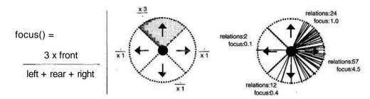
**FIGURE 3.8.3** Simple computation of the focus values for waypoint ~w in the example terrain. All relations are projected on a 2D dish withfour 90-degree sectors. Thefocus of a sector is a weighted ratio of its relations versus the relations in other sectors.
