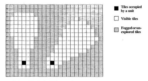
FIGURE 3.5.2 Noncircular LOS areas with two rotations of a searchlight pattern.
