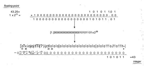
FIGURE 2.1.3 The number 43.25 is converted to an integer by manipulating the floating-point format. The underlined bits in the mantissa do not fit in memory and are discarded (with rounding).
