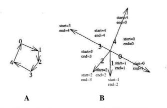
FIGURE 3.9.5 Ordering by edge vectors, start and end expansion for an edge.
