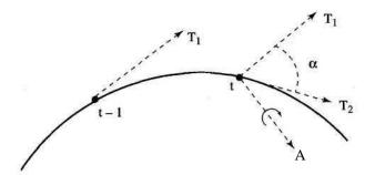
FIGURE 2.5.1 The frame at t-1 is rotated about A by Of to calculate the frame at t.
