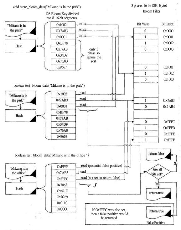
FIGURE 1.20.1 Flow of a Bloom Filter.
