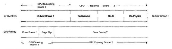
FIGURE 5.5.1 Parallelism of the GPU I CPU in an ideal game engine.
