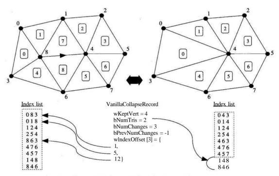
FIGURE 4.1.1 An edge collapse with before and after index lists and the VanillaCollapseRecord.
