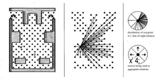
**FIGURE 3.8.1** (*left*) A top view of the example terrain, featuring two entrances!exits, and one objective o. The terrain is covered by a good number ofwaypoints, including waypoint w. (center) The waypoints in the example terrain, and the valid lines of sight from waypoint w to other waypoints. (right) The distribution of lines of sight from w, and the proposed sectors to aggregate them.
