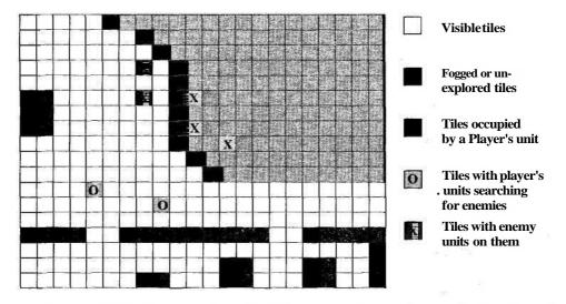
**Figure 3.5.3** Demonstration of which enemy units can be seen by the player. By respecting the total LOS, the searching units will only see the enemy units on the left, even though the units in the FOWare closer.
