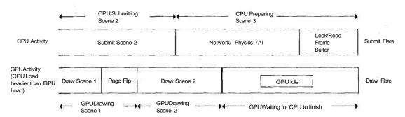
FIGURE 5.5.3 Pipeline stall caused by flush before end of frame, after CPU work.
