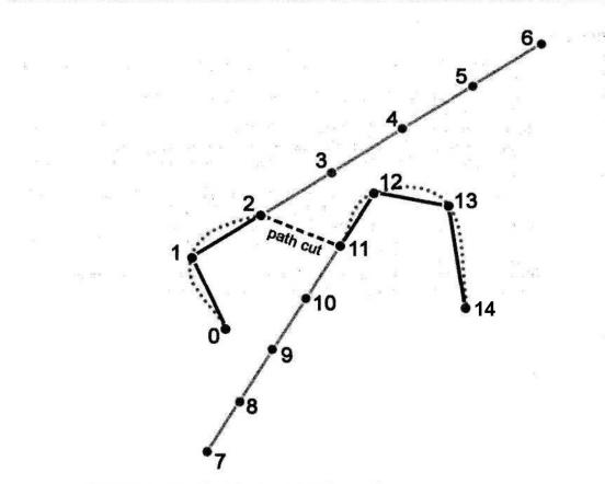
FIGURE 2.6.3 Creating phantom points for a path cut segment.
