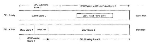
FIGURE 5.5.2 Pipeline stall caused by flush at end of rendering.
