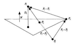
FIGURE 2.2.2 Finding the collision pointP<sub>c</sub>.
