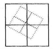
**FIGURE 5.6.3** The dashed line shows the texture sample positions lined up with the priority buffer. This mismatch of size and orientation causes aliasing.
