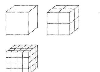
**FIGURE 4.9.2** Subdividing the skybox's faces will improve image quality at the cost of increased texture memory and polygon count. Upper left) One texture per side. Upper right) Four textures per side. Lower left) Sixteen textures per side.
