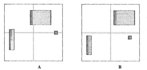
**FIGURE 4.5.1** A) Objects that cross the node's midlines cannot be stored in child nodes. B) Objects that don't cross the midlines are stored in child nodes.
