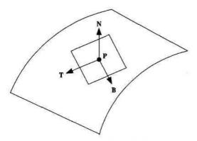
FIGURE 4.8.1 Configuration of a decal.
