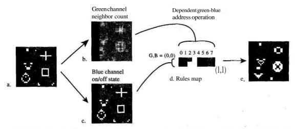
FIGURE 5.8.7 Steps in the production of the next generation of cells in Conways "Game of Life. "A) is the initial cell field. B) is the green component of the condition texture that is each 'cell's number of active neighbors. C) is the blue component of the condition that reflects whether the cell is on or off. D) is an 8x2 pixel texture that encodes the rules of the game. E) is the resulting generation of cells that will be used again as the new input a.
