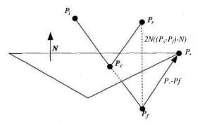
FIGURE 2.2.4 Calculating the reflected vector.
