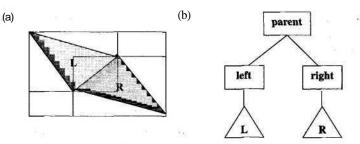
**FIGURE 4.4.2** A) The AABBs for two connected triangles will always intersect. B) The AABB tree structure for this particular geometry.
