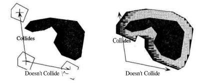
FIGURE 3.9.2 Collision shape in polygonal environment, point in expanded environment.
