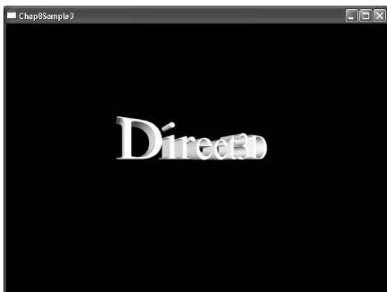
Figure 9.1: 3D text created with the D3DXCreateText function
