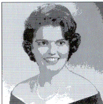
Figure 11.5 A continuous-tone photograph, digitized to a resolution of 351 \times 351 and displayed using the 2 \times 2 patterns of Fig. 11.4. (Courtesy of Alan Paeth, University of Waterloo Computer Graphics Lab.)
