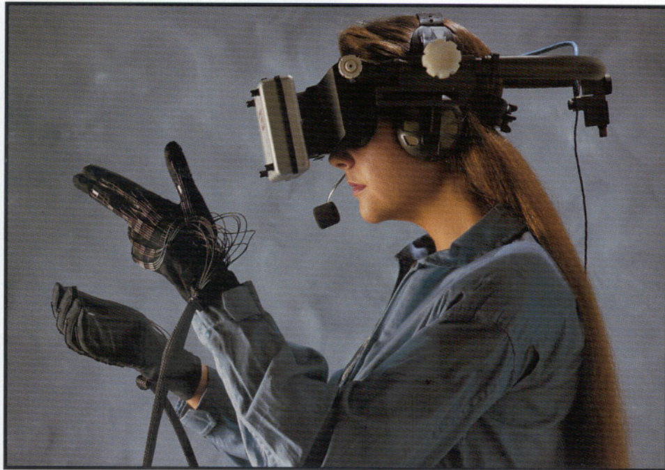
Plate 7. A User wearing a head-mounted stereo display, DataGloves, and microphone for issuing commands. These devices are used to create virtual reality for the user, by changing the stereo display presentation as the head is moved, with the DataGloves used to manipulate computer-generated objects. (Courtesy of Michael McGreevey and Scott Fisher, NASA Ames Research Center, Moffett Field, CA.)
