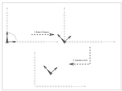
Figure 6-17: Rotational, then translational movement in *rotspikes*. The spike undergoes a local rotational movement around the origin, which happens also to be the spike's local origin. This is similar to the earth spinning around its own axis. Then, the spike is translated to its final position.
