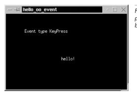
Figure 2-9: The subclassed hello\_oo\_event program, which displays X events in real time on a black XImage background.
