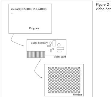
Figure 2-1: Full-screen, direct access to video hardware.
