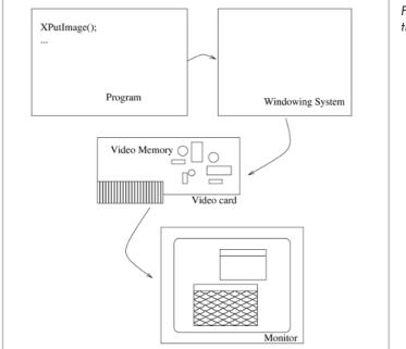
Figure 2-3: Access to screen through window manager
