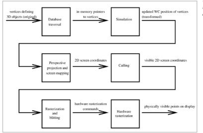
Figure 5-28: One example of a 3D pipeline.
