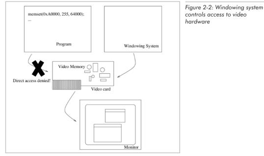
The windowing system forms a middle layer between the application and the video hardware. Graphics applications can, in general, no longer directly access the video hardware but instead direct requests to the windowing system to display images within the application's window (Figure 2-3).
