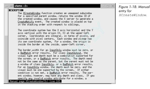
The manual entry contains a detailed, complete specification of the XCreateWindow function. Standard C library functions, X functions, and Linux system functions all have similarly complete entries in the online manual.
