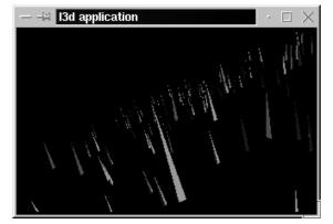
Figure 6-27: Output from sample program *camspikes*. Notice that the viewpoint is slightly above the spikescape, looking diagonally down, with a tilted horizon.
