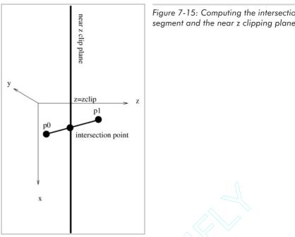
Figure 7-15: Computing the intersection between a crossing segment and the near z clipping plane.
