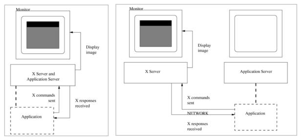
Figure 1-7: X on a single-user system.
