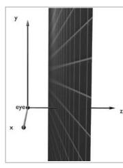
Figure 7-14: The near z clipping plane.
