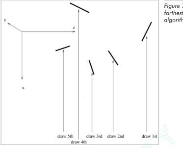
Figure 7-26: We sort polygons from farthest to nearest for the painter's algorithm.
