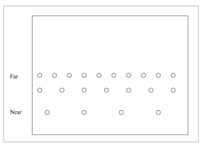
Figure 4-10: Plotting runway lights on the screen. Chapter 4: 3D Vision and Perception
