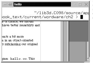
Figure 2-6: The window created by the sample program is not empty, but instead appears to contain "leftover" graphics from another window.
