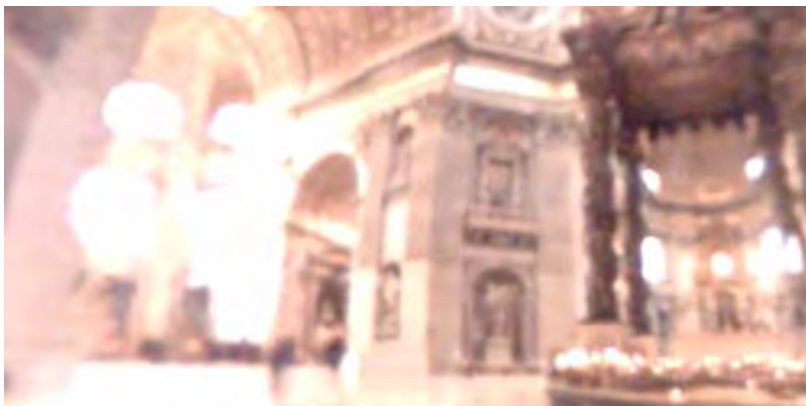
Figure 8.8: Application of the contrast-preserving scale factor to the image works well in some parts of the image, though it doesn't do well at preserving detail in the very bright areas. Any operator that uses a single global scale factor is susceptible to this problem.
