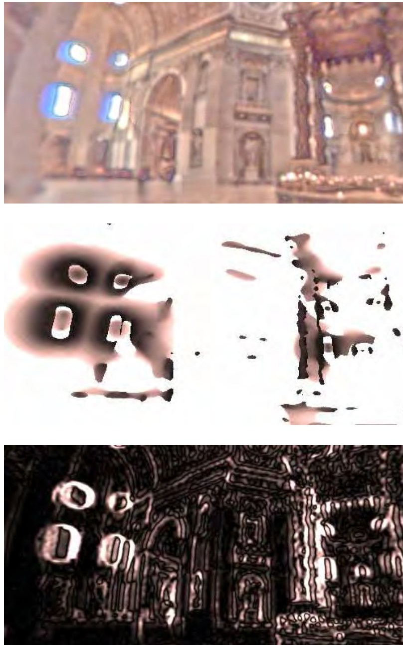
Figure 8.10: The high-contrast tone reproduction operator computes a spatially-varying adaptation luminance while paying attention to boundaries between areas with substantially different luminances. The result of its use on the St. Peter's image is shown at the top. It does an excellent job of remapping this image to a small dynamic range. The middle image is a grey-scale visualization of the blur radius that was used to compute adaptation luminance at each pixel; boundaries with large luminance changes are successfully detected, indicated by small radii, while areas with slower change in luminance compute adaptation luminance over a wider area. The bottom image shows the local contrast computed at each pixel with a blur radius of 1.5 and 3 pixels.
