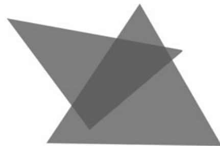
Figure 13.8 Overlapping polygons in the small map can create strange color artifacts when rendered using alpha blending.
