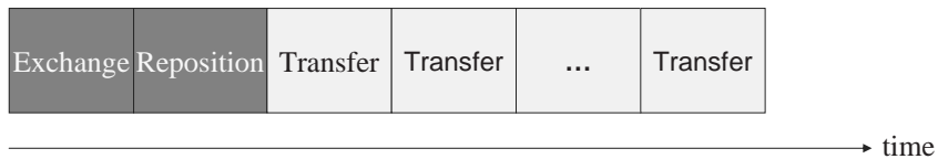
Figure 9.5. The major time spent in serving a request at the tertiary storage devices
