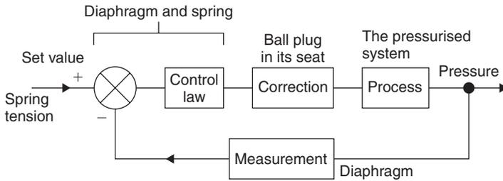
**Figure 18.67: Fuel supply control system**
