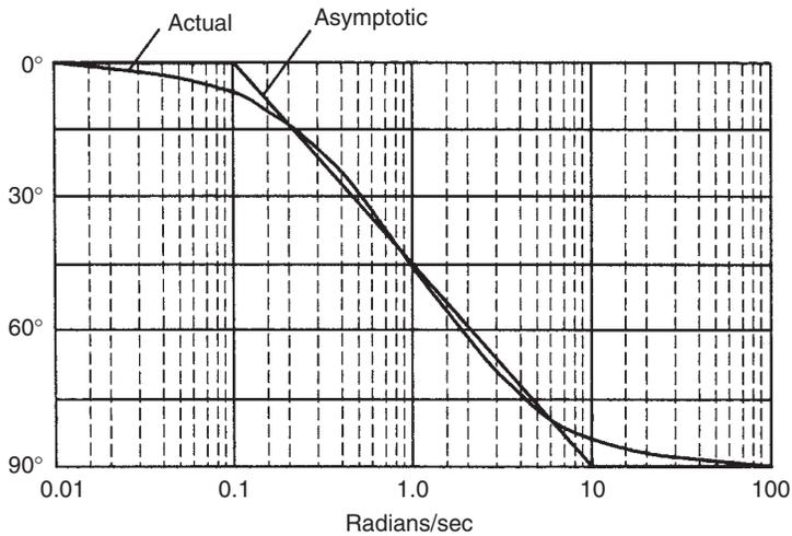
**Figure 15.16: Phase responses of an R/C low-pass filter**
