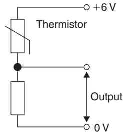
**Figure 18.34: Resistance to voltage conversion for a thermistor**
