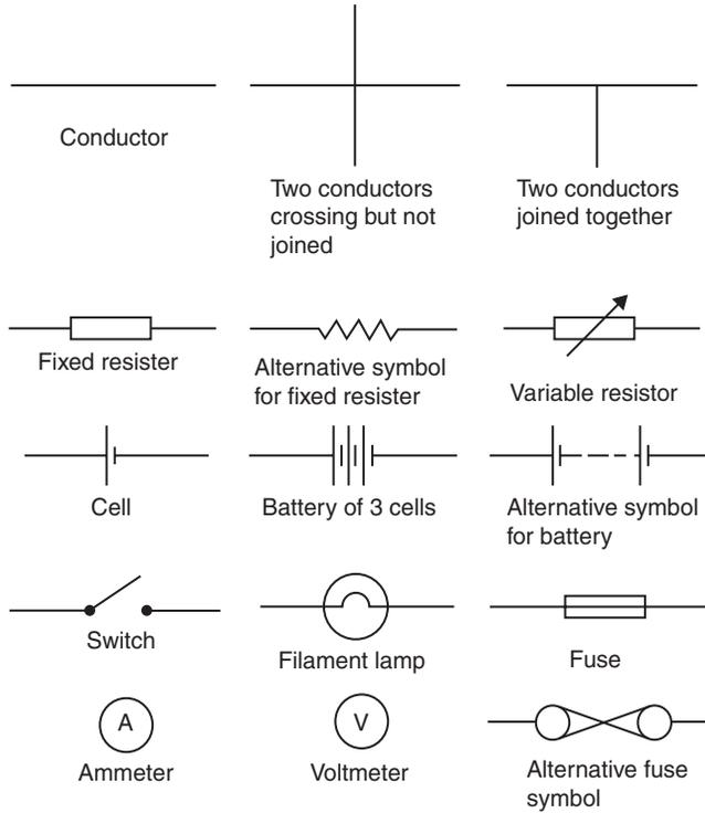
Figure 1.1: Common electrical component symbols
