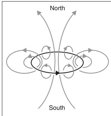
**Figure 21.4: Magnetic field lines surrounding a current loop**
