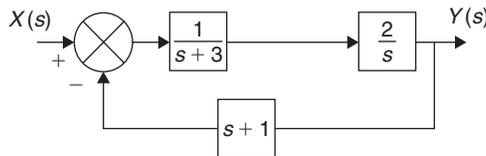
Figure 18.125: System with disturbance put equal to zero
