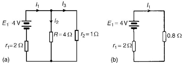
**Figure 5.12: (a) Redrawn circuit; (b) Equivalent circuit**
