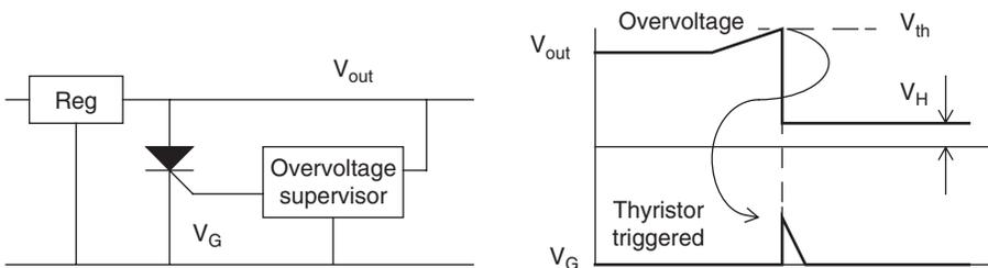
Figure 15.38: Overvoltage protection
