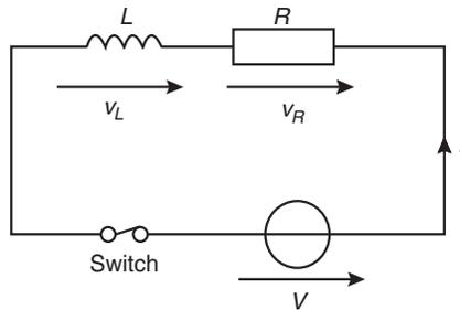
Figure 8.6: Series R-L circuit
