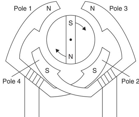
**Figure 18.58: The basic principles of the permanent magnet stepper motor (2-phase) with a rotor giving**
