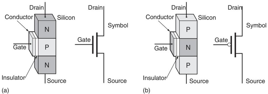
Figure 10.7: Metal-oxide semiconductor field-effect transistors (MOSFETs)
