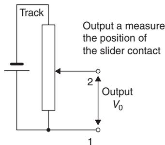
**Figure 18.13:** Potentiometer as a sensor of position
