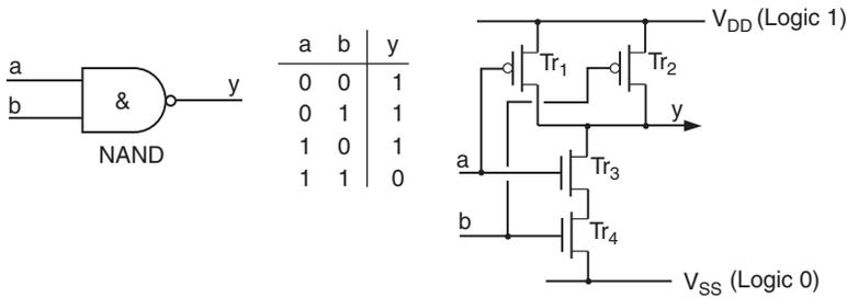
Figure 10.23: CMOS implementation of a 2-input NAND gate
