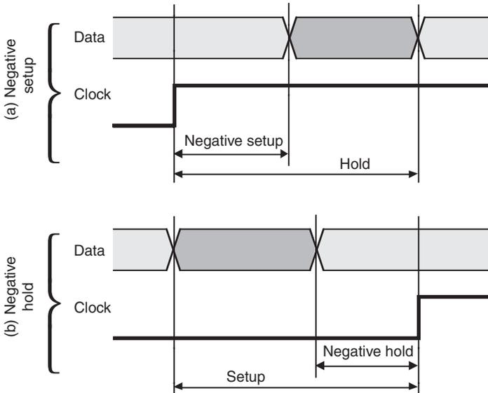
**Figure 10.79: Negative setup and hold times**
