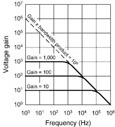
Figure 11.5: Frequency response curves for an operational amplifier
