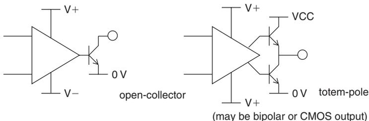
Figure 11.37: Comparator outputs
