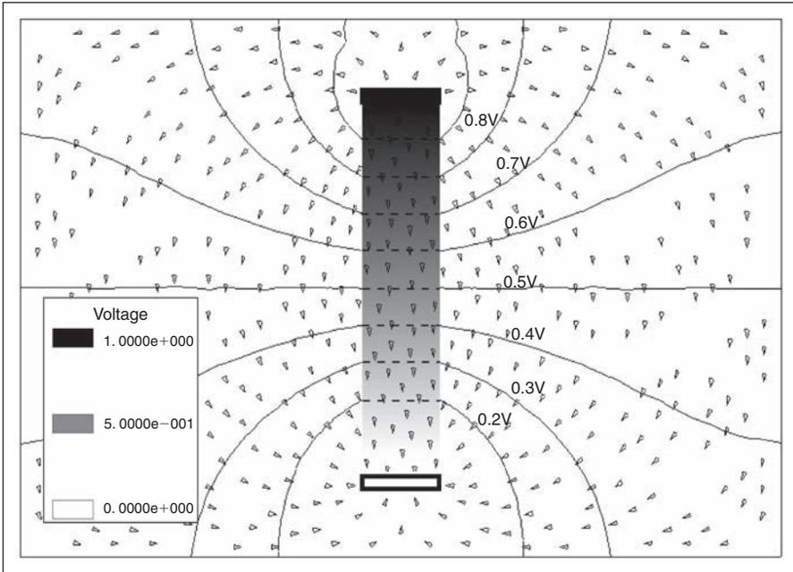
**Figure 20.23: Electric field of DC voltage across a conducting wire. Arrowheads show the direction of the electric field. Voltage is shown by shade inside the conductor and as contours outside the conductor. This figure was created using Ansoft Corporation’s Maxwell 2D field solver software (<http://www.ansoft.com>)**
