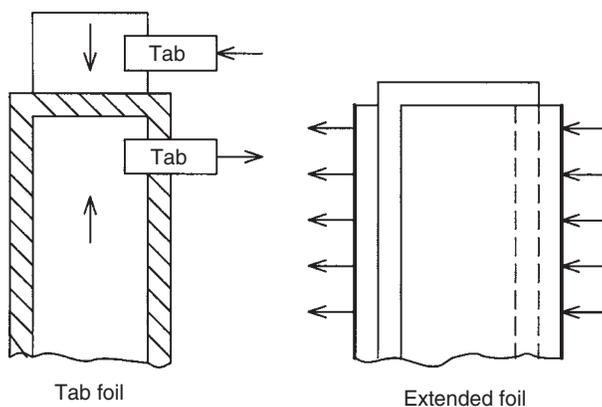
**Figure 15.4: Capacitor construction**
