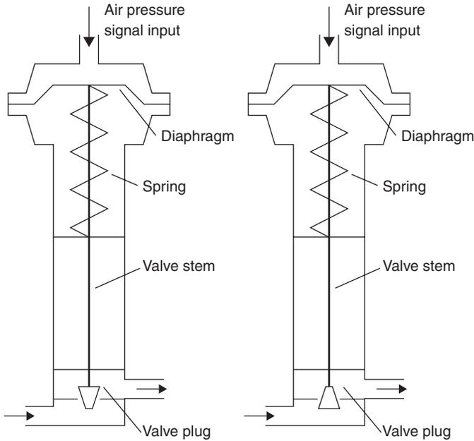
**Figure 18.54: Direct action: (a) air pressure increase to close; (b) air pressure increase to open**
