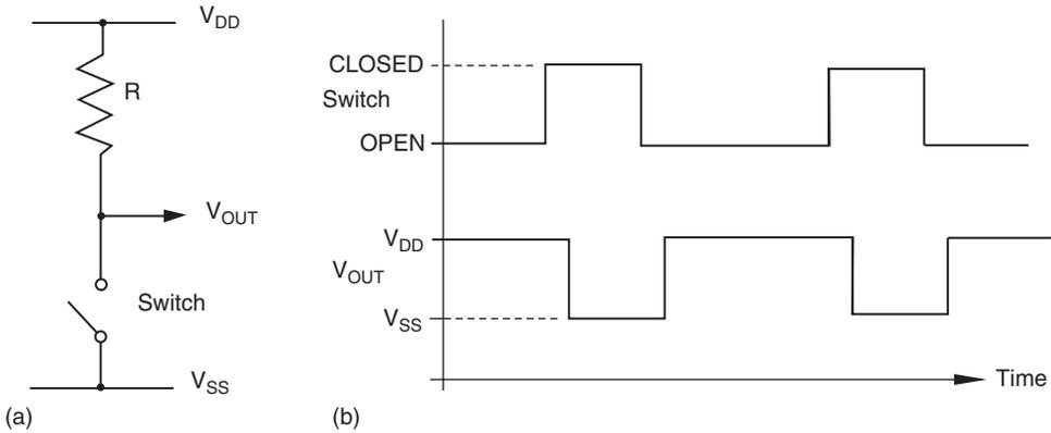
**Figure 10.8: Resistor-switch circuit (a) Circuit; (b) Waveform**
