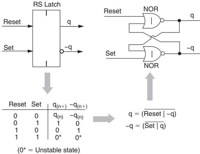
Figure 10.62: NOR implementation of an RS latch
