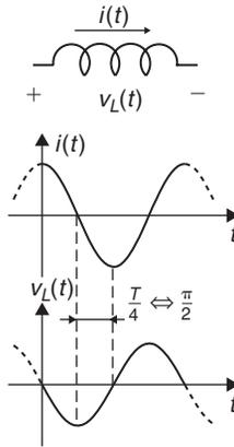
Figure 9.7: Voltage and current in an inductor
