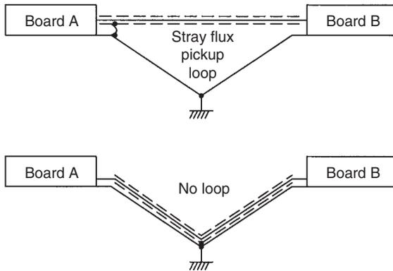
Figure 22.1: Signal wire routing
