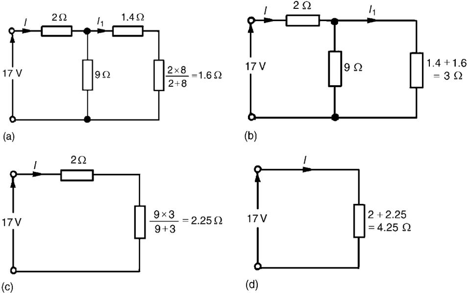
Figure 3.23: Solution to Example 3.13, in four stages
