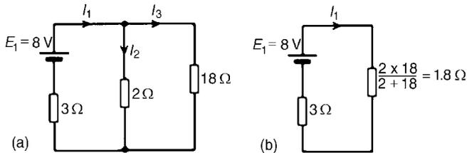
Figure 5.17: (a) Redrawn circuit; (b) Equivalent circuit
