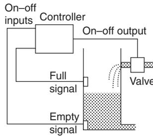
**Figure 18.12:** Discrete-event control with the controller switching the valve open when empty signal received and closed when the full signal
