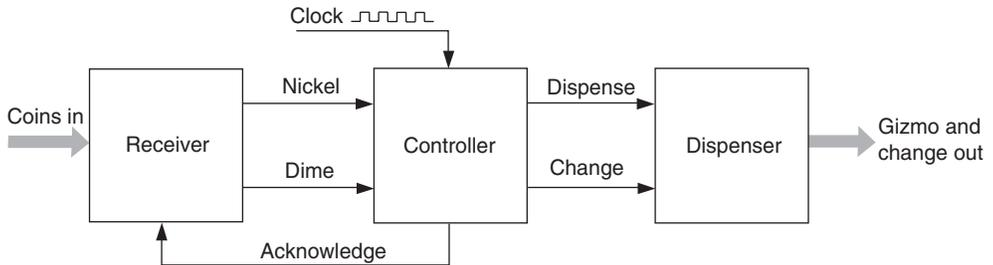
Figure 10.80: Block diagram of a coin-operated machine
