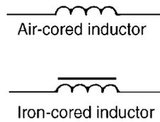
Figure 4.16: Standard electrical symbols for air-cored and iron-cored inductors
