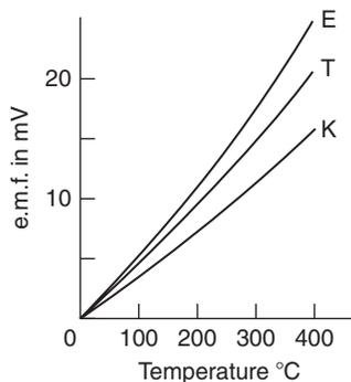
**Figure 18.31: Thermocouples: chromel-constantan (E), chromelalumel (K), copper-constantan (T)**
