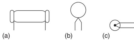
**Figure 18.29: Thermistors: (a) rod; (b) disc; (c) bead**
