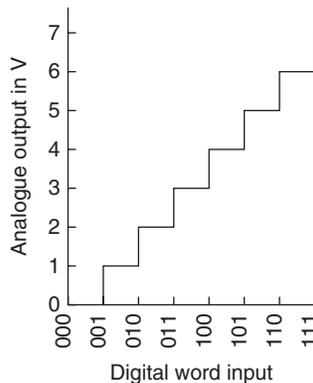
Figure 18.41: Digital-to-analog conversion
