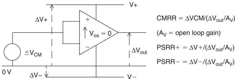
Figure 11.25: Common mode and power supply rejection ratio
