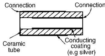
Figure 4.12: Cross-section of tube of ceramic material
