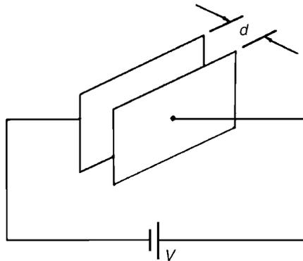
Figure 4.3: Two parallel conducting plates separated by air
