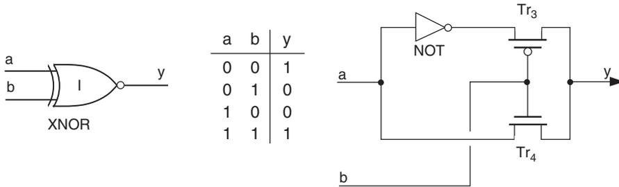
Figure 10.28: CMOS implementation of a 2-input XNOR gate
