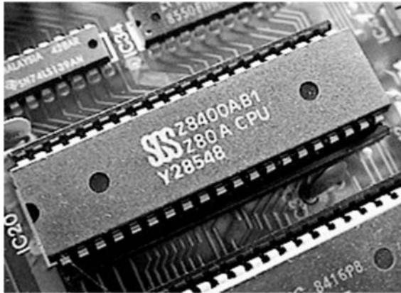
Figure 14.2: A Z80 microprocessor
