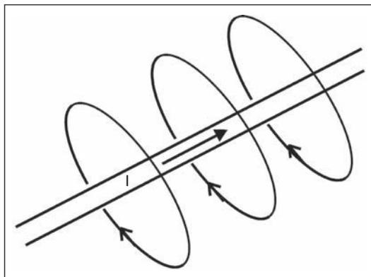
Figure 21.1: Magnetic field lines surrounding a current-carrying wire
