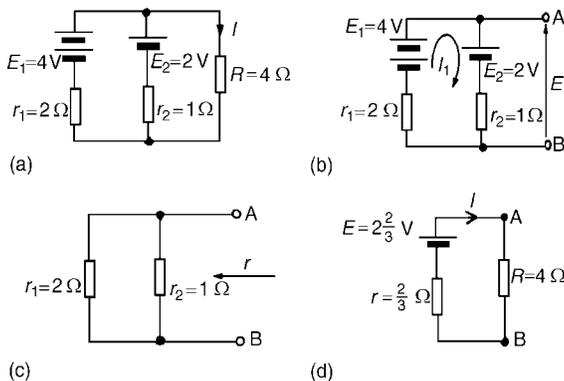
Figure 5.30: Circuit for Example 5.9 showing steps for solution
