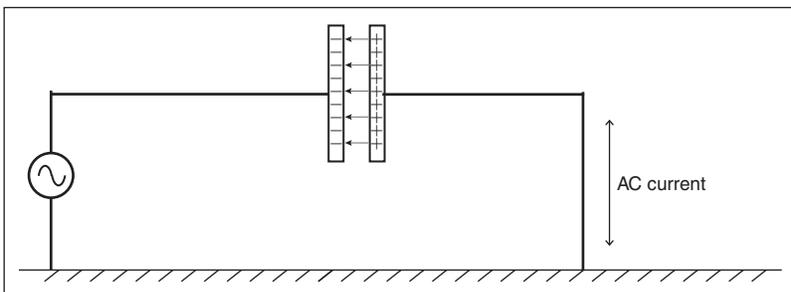
Figure 20.17: Spheres are replaced by metal plates
