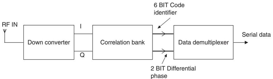
Figure 19.49: CCK decoding
