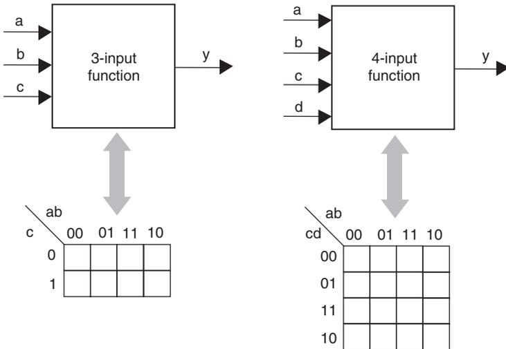
Figure 10.47: Karnaugh maps for 3-input and 4-input functions
