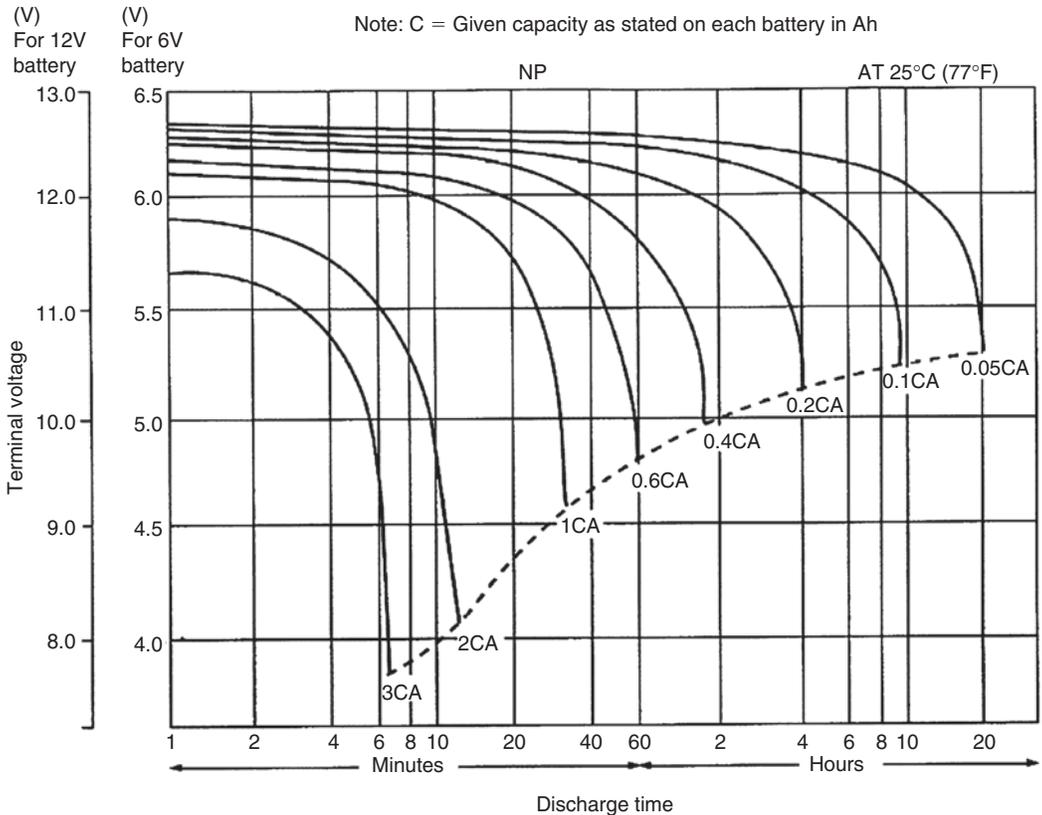
**Figure 15.42: Discharge characteristics for sealed lead-acid batteries.**
