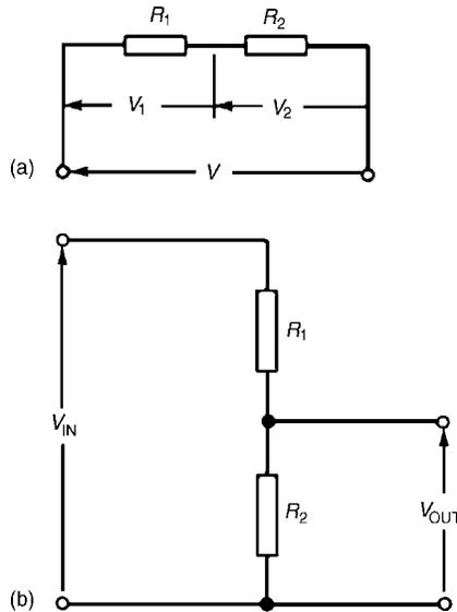
Figure 3.5: Potential divider circuit
