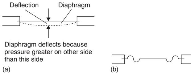
**Figure 18.20: Diaphragm sensors**
