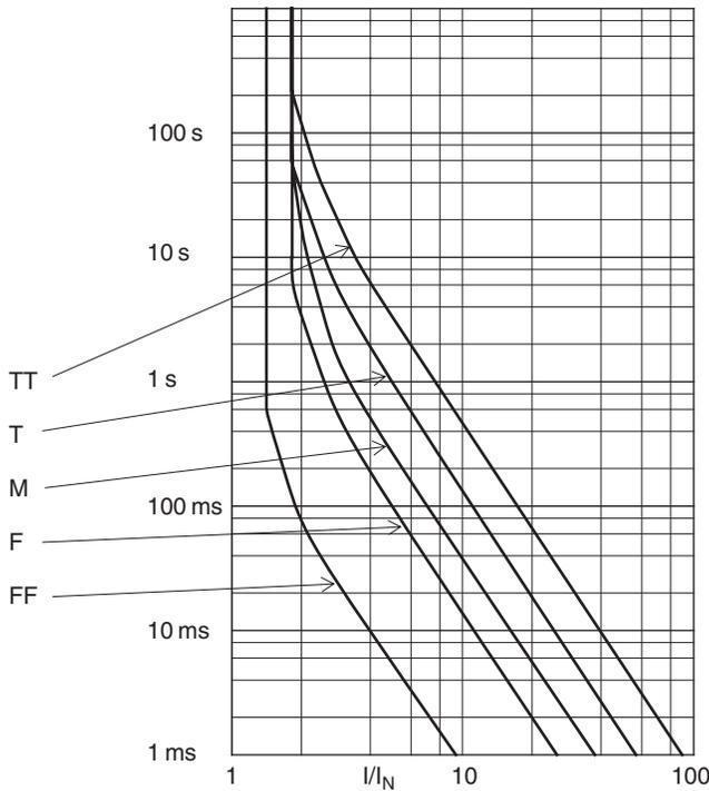
Figure 15.23: Typical fuse time-current curves
