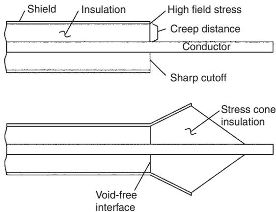
Figure 15.3: Stress cone termination for shielded cable
