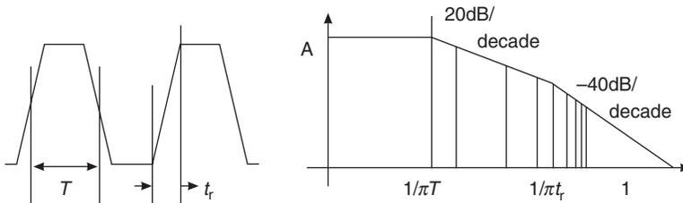
Figure 25.5: Waveform and spectrum of a digital signal
