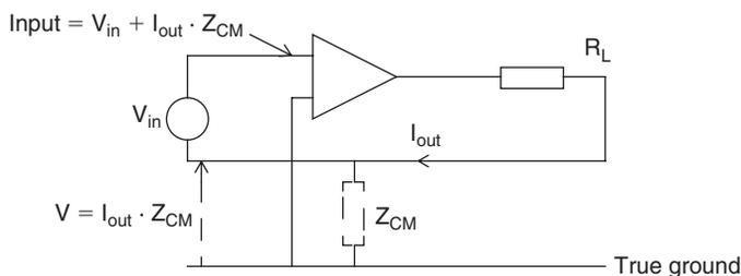
Figure 11.32: Common-impedance ground coupling
