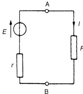
Figure 5.39: Source  $E$  in series with resistance  $r$  feeding load resistance  $R$
