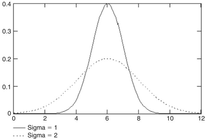
**Figure 19.33: Gaussian density function with different standard deviations**
