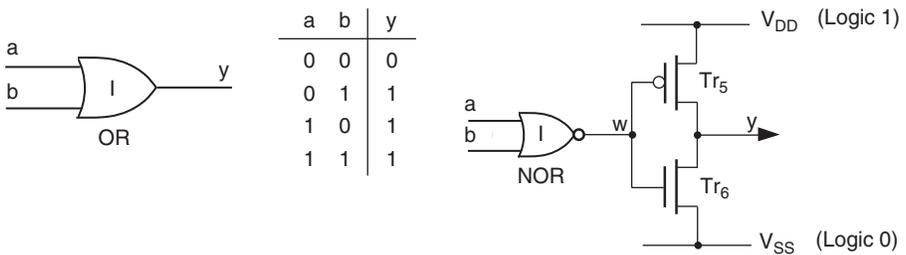
Figure 10.27: CMOS implementation of a 2-input OR gate
