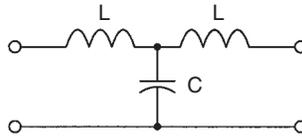
Figure 22.4: T-section filter
