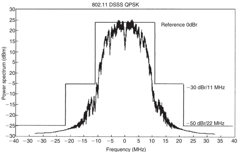
Figure 19.42: 802.11 DSSS spectral mask
