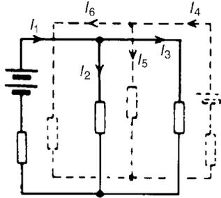
Figure 5.14: Superimposed circuits
