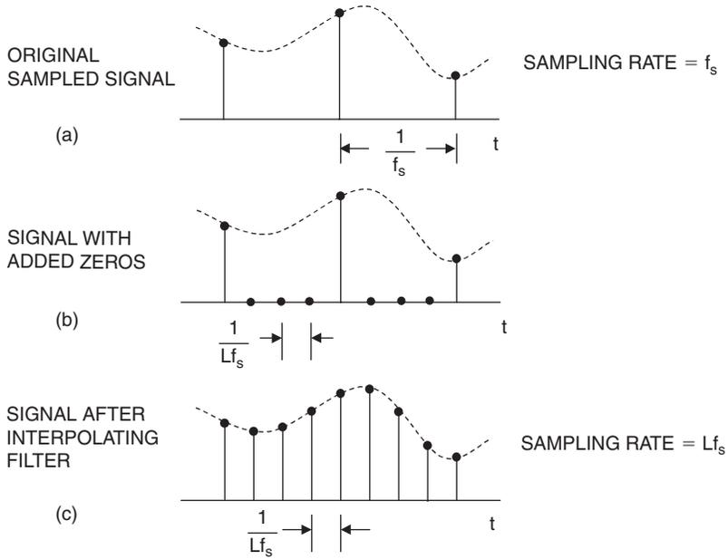
Figure 17.116: Interpolation by a factor of  $L$
