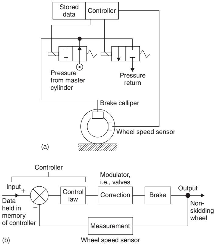
**Figure 18.68: Antilock brakes: (a) schematic diagram; (b) block form of the control system**
