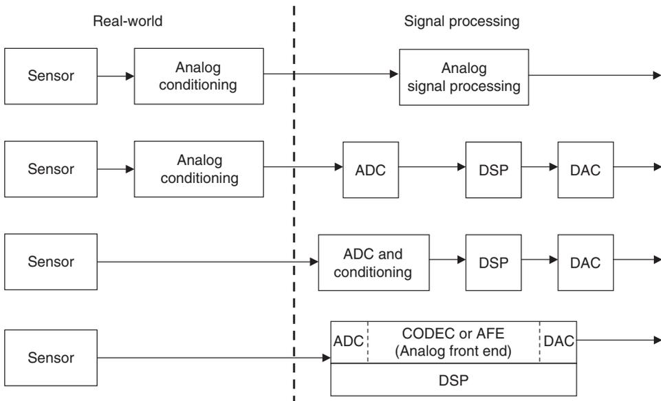
Figure 16.3: Analog and digital signal processing options
