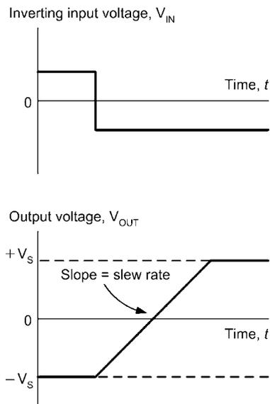
Figure 11.4: Slew rate for an operational amplifier
