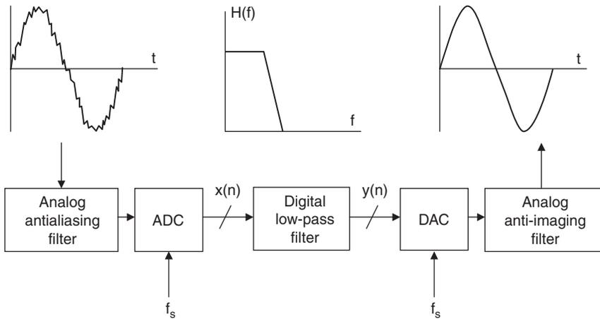
**Figure 17.76: Digital filtering**
