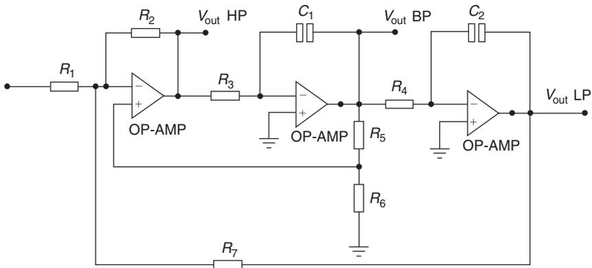
Figure 17.37: State variable filter
