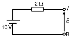
Figure 5.20: Example circuit
