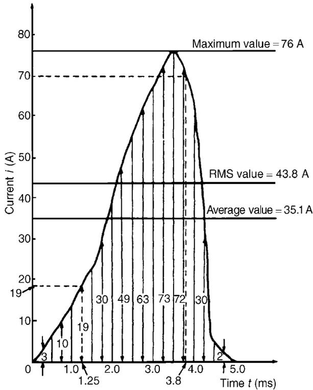
Figure 6.6: Half cycle of alternating current for Example 6.5
