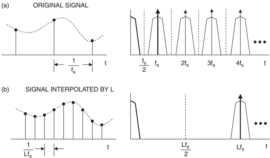
Figure 17.117: Effects of interpolation on frequency spectrum
