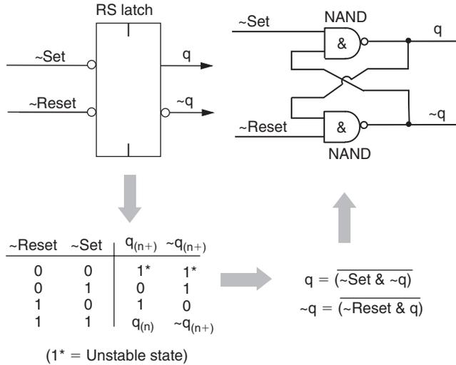
**Figure 10.66: NAND implementation of an RS latch**
