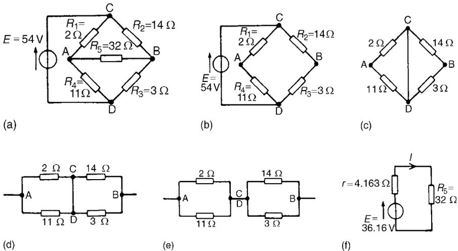
Figure 5.32: Network for Example 5.11 showing steps for solution
