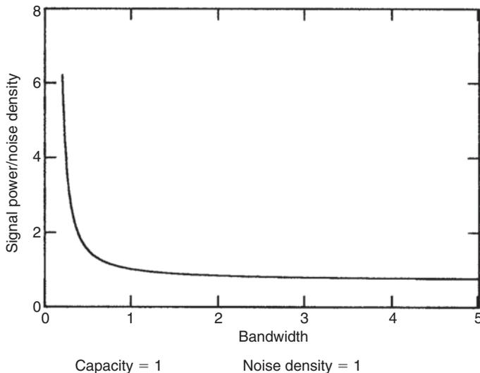
**Figure 19.34: Signal power vs. bandwidth at constant capacity**
