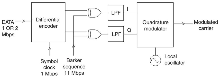
Figure 19.44: DSSS modulation
