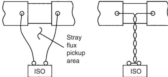
Figure 22.5: Shunt wiring
