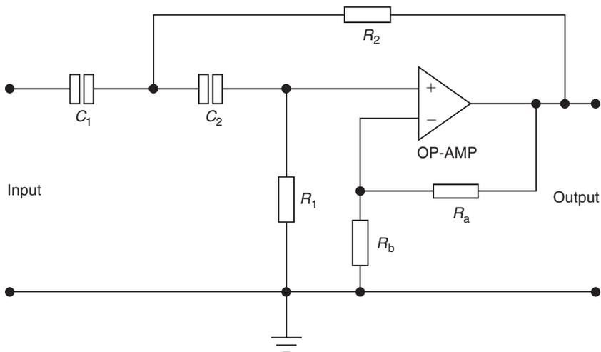
Figure 17.19: Sallen-Key circuit for high-pass filter
