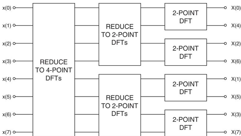
**Figure 17.61: Computation of an 8-Point DFT in three stages using decimation-in-frequency**
