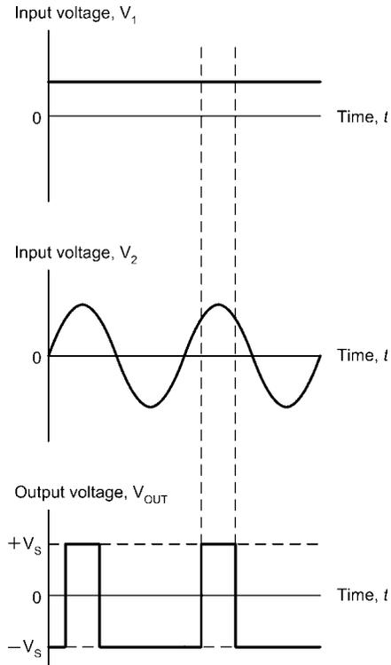
**Figure 11.18:** Typical input and output waveforms for a comparator
