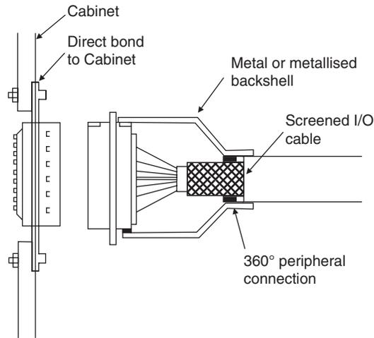
**Figure 25.14: Correct 360° peripheral termination of screened cable**
