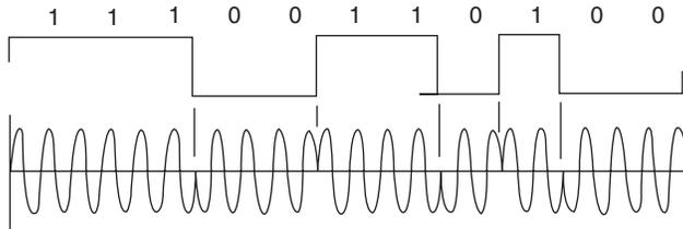
**Figure 19.24: Binary phase-shift keying (BPSK)**
