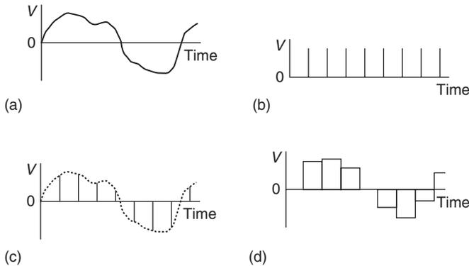
**Figure 18.38:** (a) Analog signal; (b) time signal; (c) sampled signal; (d) sampled and held signal
