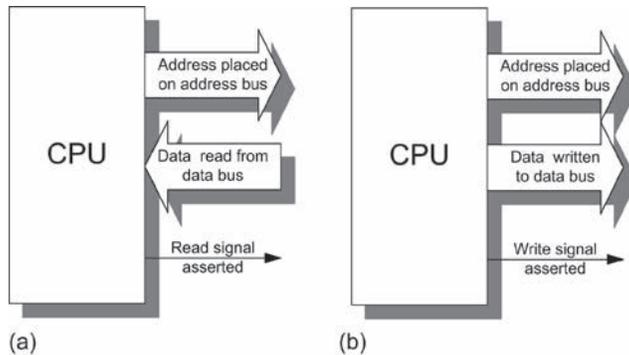
Figure 14.6: (a) Read; and (b) write operations
