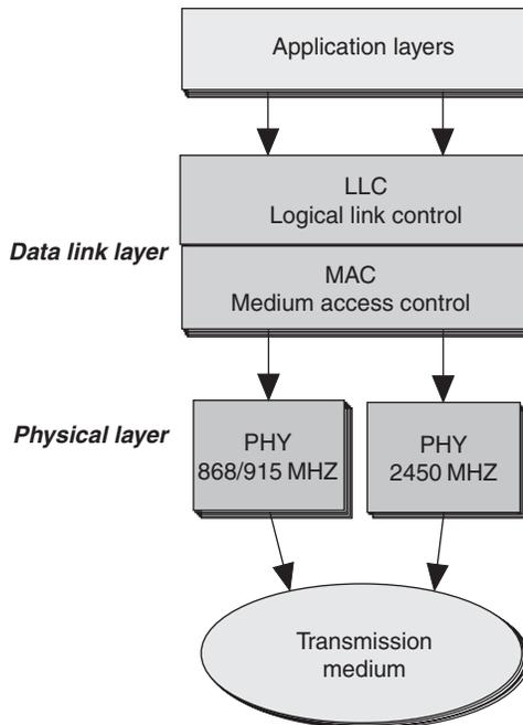
Figure 19.56: Zigbee architecture
