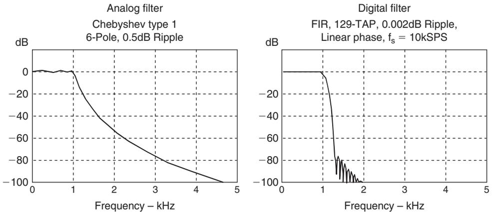
Figure 17.78: Analog vs. digital filter frequency response comparison
