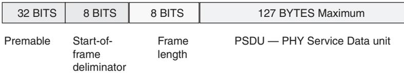
**Figure 19.59: Transmission packet**
