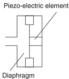
Figure 18.22: Basic form of a piezo-electric sensor
