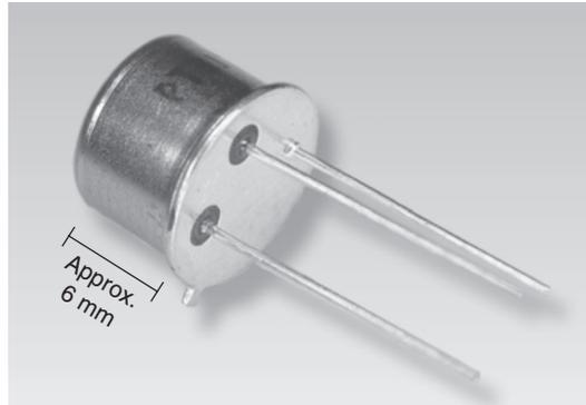
Figure 10.6: Individually packaged transistor (photo courtesy of Alan Winstanley)
