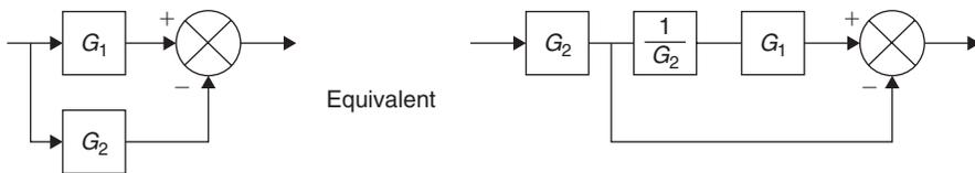
**Figure 18.116: Removing a block from a forward path**
