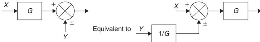
Figure 18.114: Moving a summing point beyond a block
