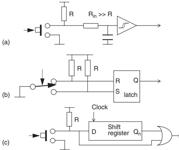
**Figure 13.4: Switch de bouncing circuits**
