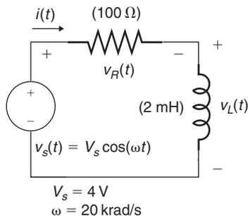
Figure 9.9: RL circuit
