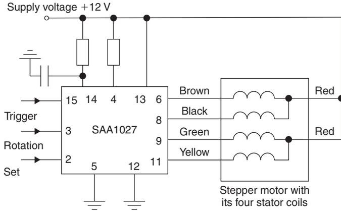
**Figure 18.60: Driver circuit SAA 1027 for a 12V 4-phase stepper motor**
