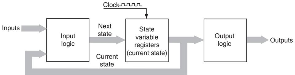
**Figure 10.83: Block diagram of a Moore machine**
