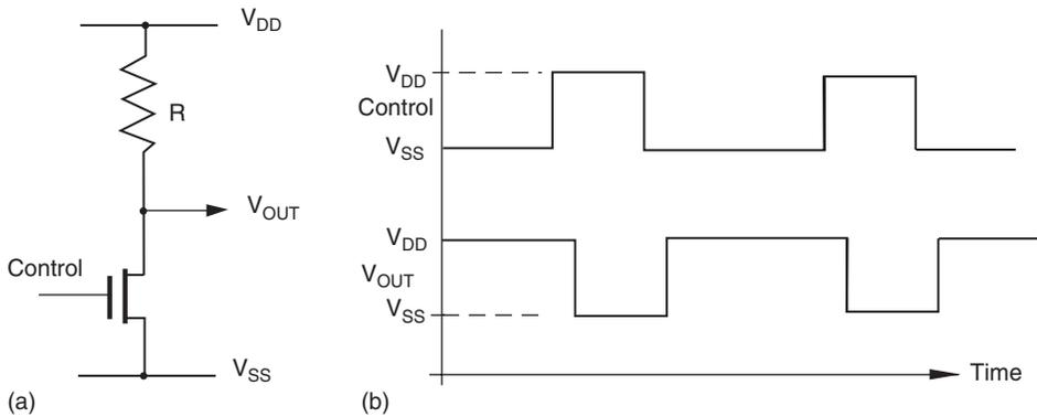
**Figure 10.9: Resistor-NMOS transistor circuit (a) Circuit; (b) Waveform**
