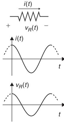
Figure 9.5: Voltage and current in a resistance
