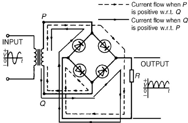
Figure 6.16: Bridge rectifier
