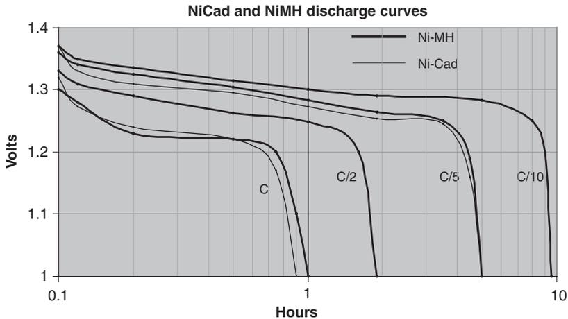
Figure 15.43: NiCad and NiMH discharge characteristics
