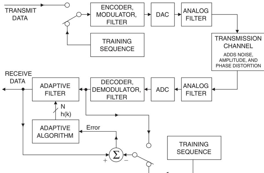
Figure 17.121: Digital transmission using adaptive equalization
