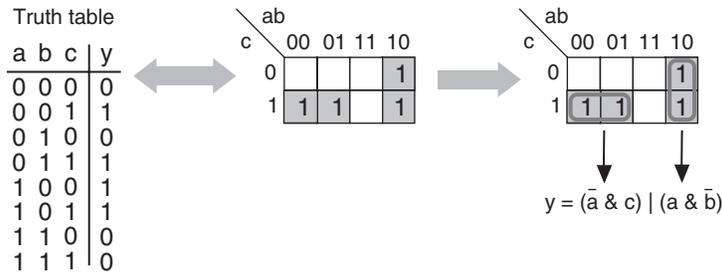
Figure 10.49: Karnaugh map minimization of example 3-input function
