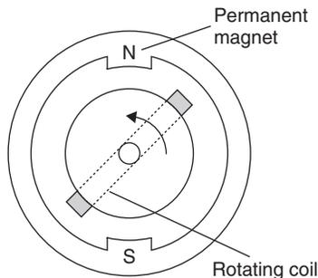
Figure 18.19: The tachogenerator
