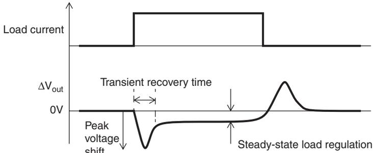
**Figure 15.33: Load transient response**
