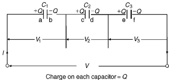
Figure 4.7: Three capacitors connected in series
