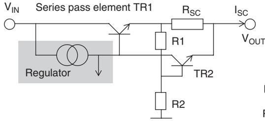
As before, \$TR2\$ diverts base drive away from \$TR1\$; \$R1\$ and \$R2\$ provide positive feedback once output current exceeds the "knee" current \$I\_K\$, such that the short-circuit current \$I\_{SC}\$ is less than \$I\_K\$.
