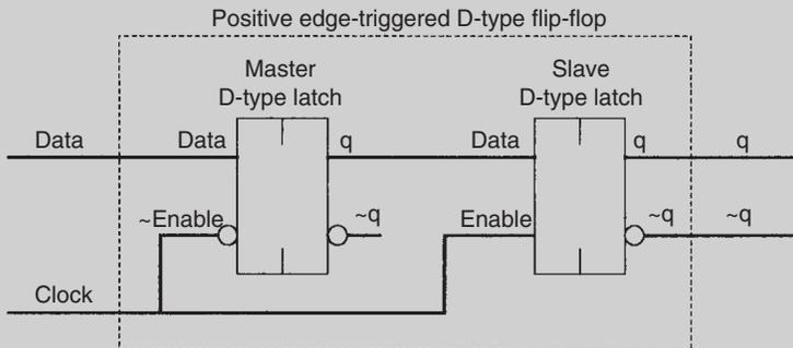
The first rising edge of the clock loads the 0 on the data input into the flip-flop, which (after a small delay) causes  $q$  to change to 0 and  $\sim q$  to change to 1. The second rising edge of the clock loads the 1 on the data input into the flip-flop;  $q$  goes to 1 and  $\sim q$  goes to 0.
