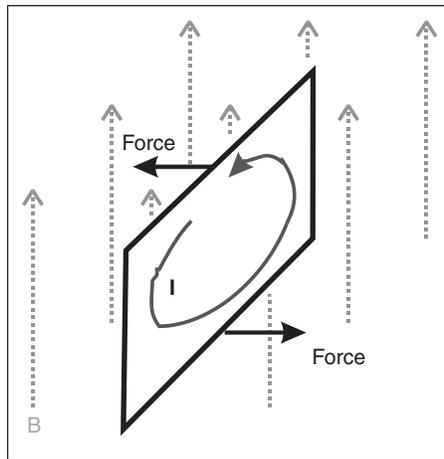
**Figure 21.15: A current-carrying loop experiences a torque (rotational force) causing it to line up with an applied magnetic field**
