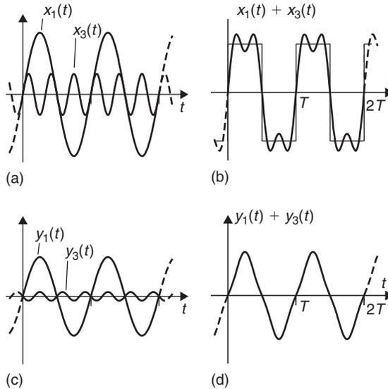
**Figure 9.20:** (a) The first two non-zero terms of the Fourier series for the periodic rectangular waveform; (b) The sum of first two non-zero terms of the Fourier series as an approximation to the periodic rectangular waveform; (c) The first two non-zero terms of the Fourier series for the periodic triangular waveform; (d) The sum of first two non-zero terms of the Fourier series as an approximation to the periodic triangular waveform
