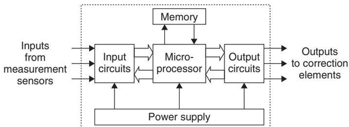
Figure 18.77: Microprocessor-based controller
