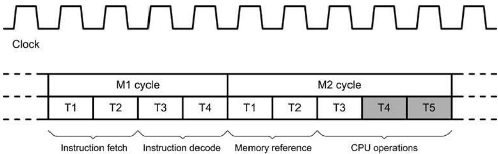
Figure 14.7: A typical timing diagram for a microprocessor's fetch-execute cycle
