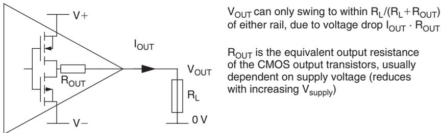
**Figure 11.27: Limits on rail-to-rail swing with CMOS outputs**
