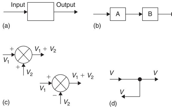
**Figure 18.4: Block diagram elements: (a) system element; (b) information paths; (c) summing junction; (d) takeoff point**
