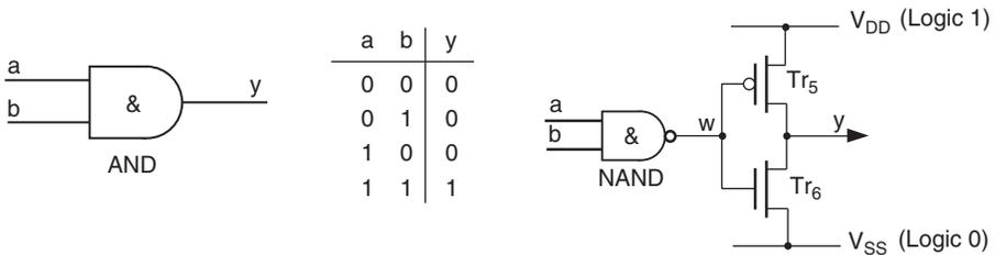
Figure 10.25: CMOS implementation of a 2-input AND gate
