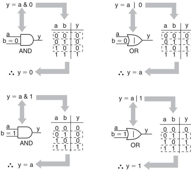
Figure 10.31: Combining a single variable with a logic 0 or logic 1
