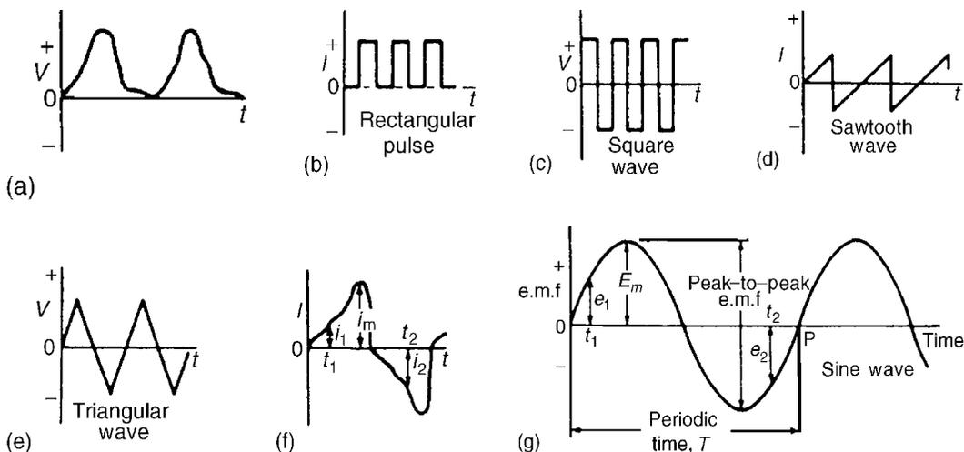
Figure 6.3: Typical waveforms
