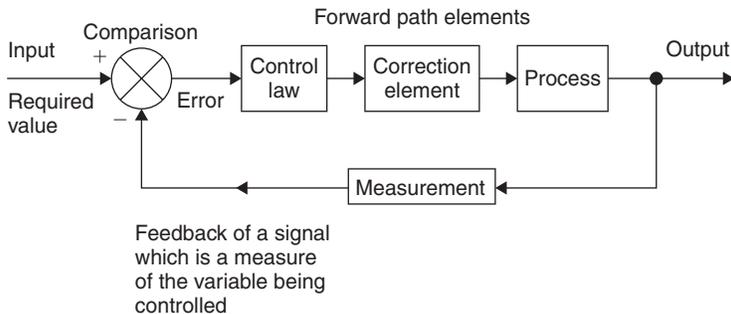
**Figure 18.10: Basic elements of a closed-loop control system**
