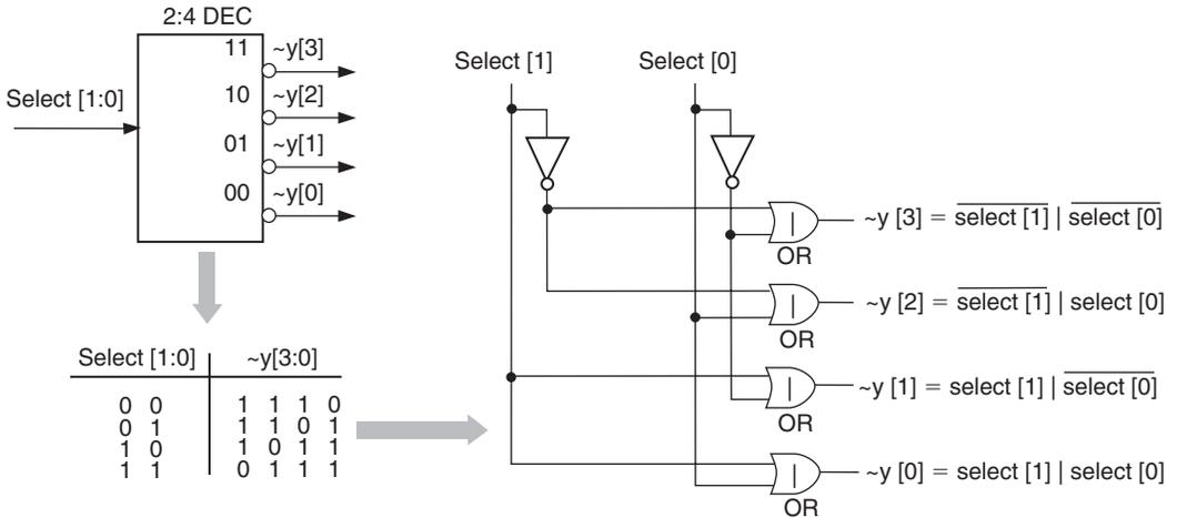
Figure 10.59: A 2:4 decoder with active-low outputs
