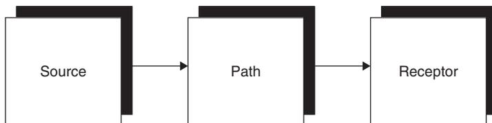
**Figure 25.2: Source-Path-Receptor model**
