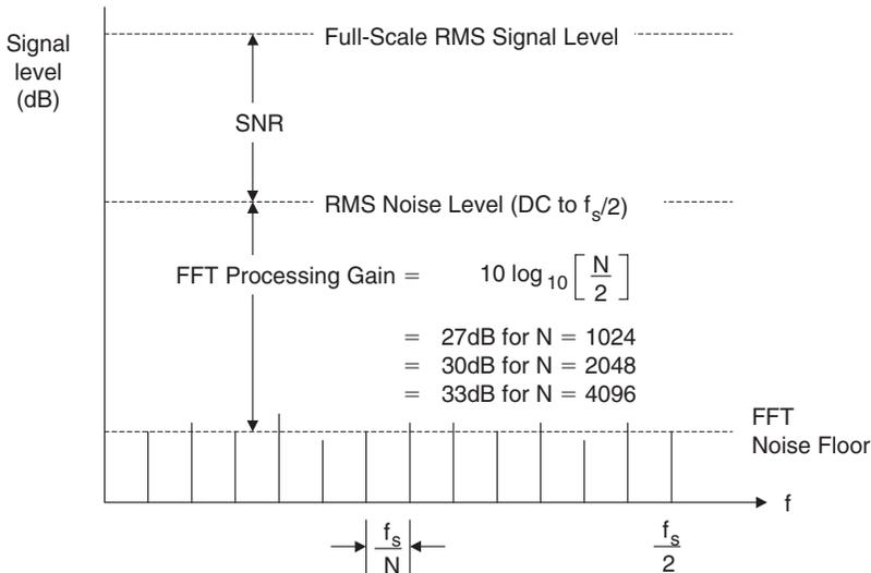
**Figure 17.69: FFT processing gain neglecting round-off error**
