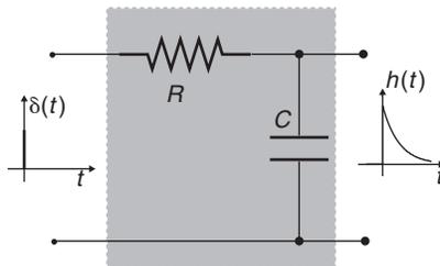
Figure 9.43: Impulse response of an RC circuit
