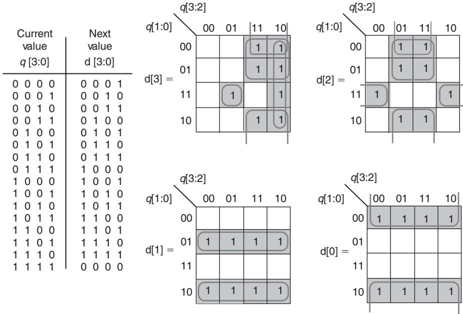
$$d[3] = (q[3] \& \overline{q[1]}) \mid (q[3] \& \overline{q[2]}) \mid (q[3] \& \overline{q[0]}) \mid (\overline{q[3]} \& q[2] \& q[1] \& q[0])$$
