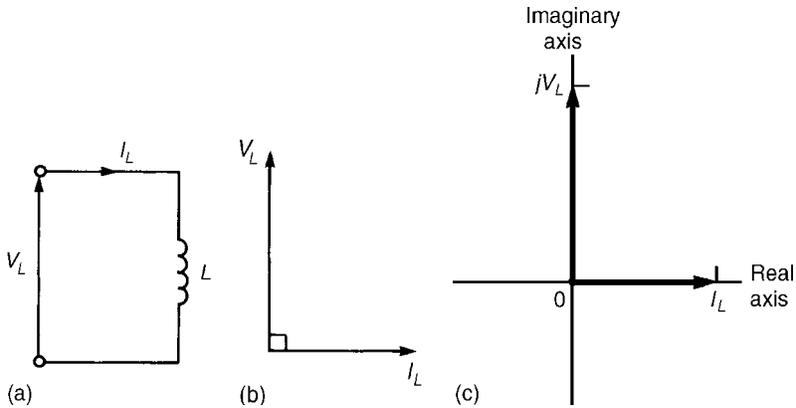
Figure 7.5: (a) Circuit diagram; (b) Phasor diagram; (c) Argand diagram
