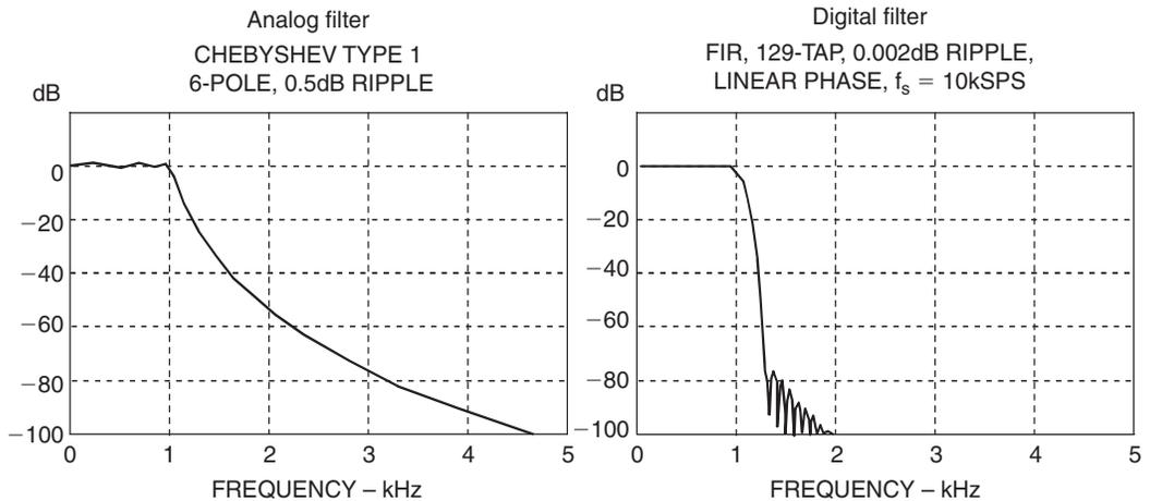
Figure 16.5: Analog versus digital filter frequency response comparison
