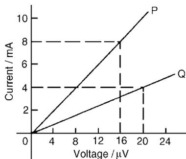
Figure 1.5: Current/voltage for two resistors A and B
