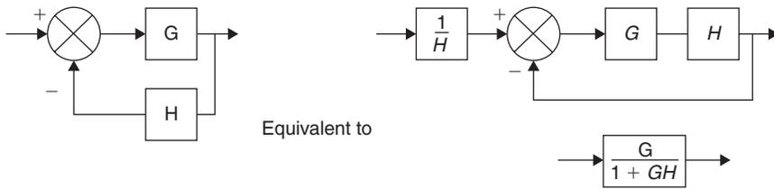
**Figure 18.115: Removing a block from a feedback path**
