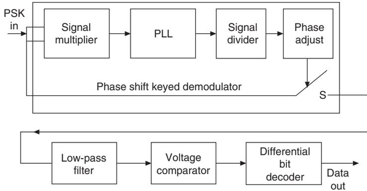
**Figure 19.26: Circuit to demodulate a BPSK waveform**
