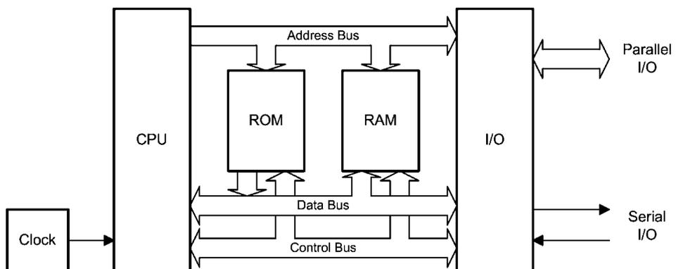
Figure 14.1: Block diagram of a microprocessor system
