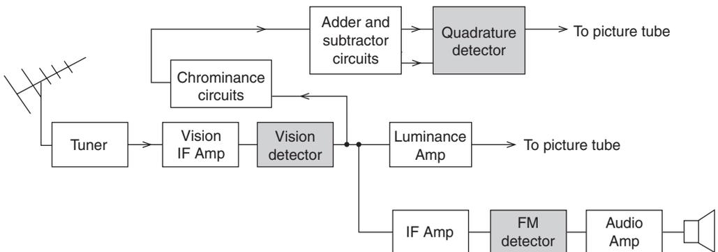
Figure 19.1: Block diagram of color TV receiver
