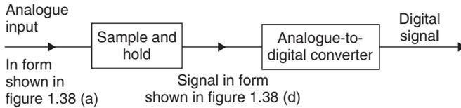
**Figure 18.39: Analog-to-digital conversion**
