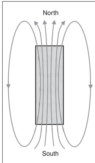
**Figure 21.6: Magnetic field lines surrounding a bar magnet**
