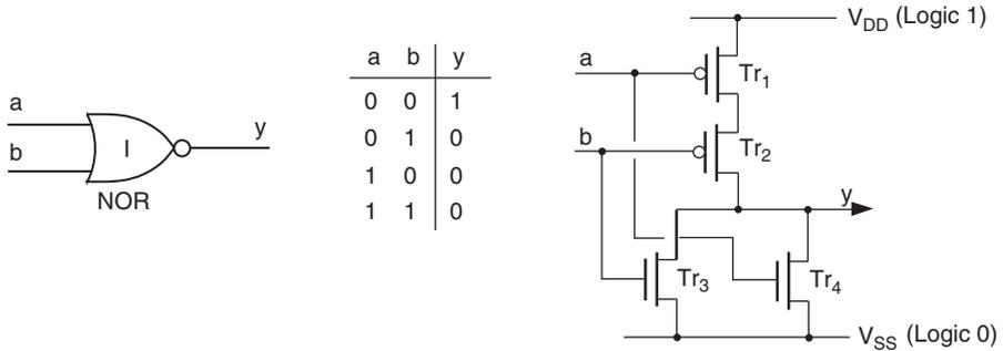
Figure 10.26: CMOS implementation of a 2-input NOR gate
