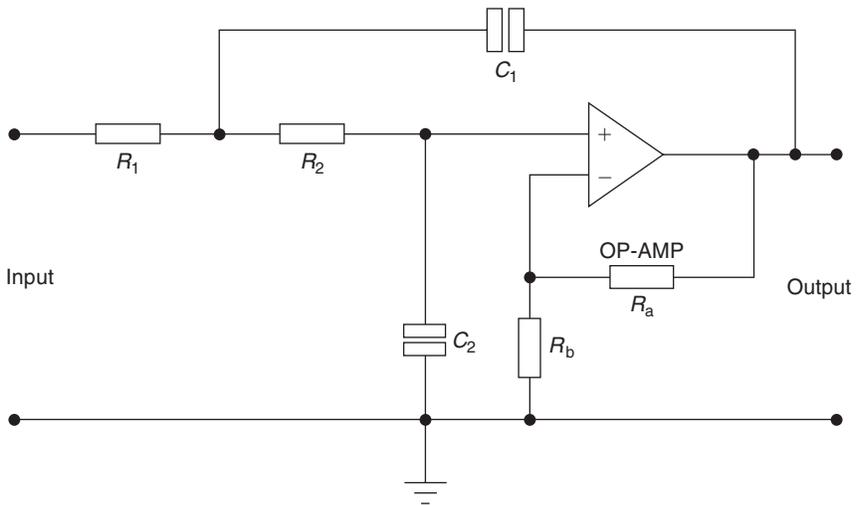
Figure 17.15: Sallen-Key circuit
