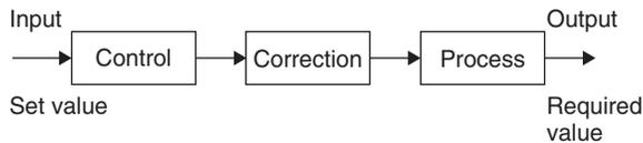
**Figure 18.9:** Basic elements of an open-loop control system
