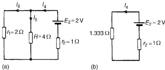
Figure 5.13: (a) Redrawn circuit; (b) Equivalent circuit
