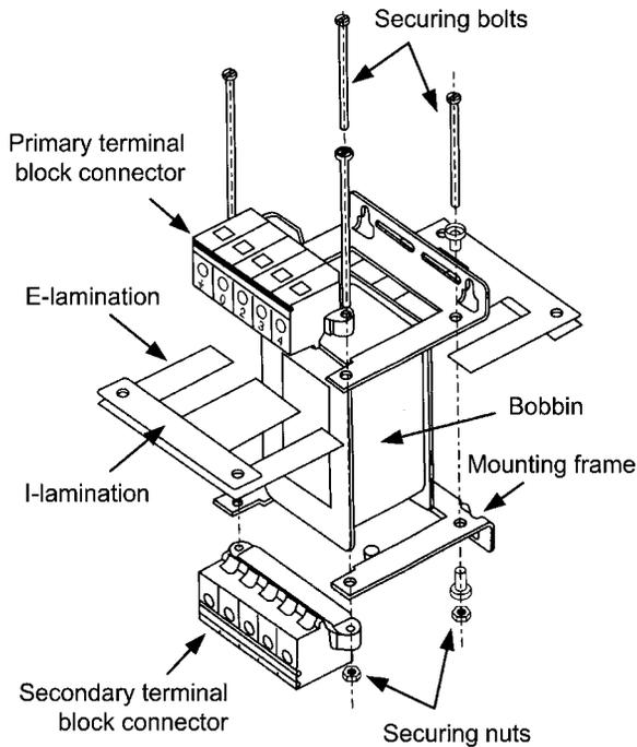
Figure 24.3: Construction of a typical iron-cored transformer
