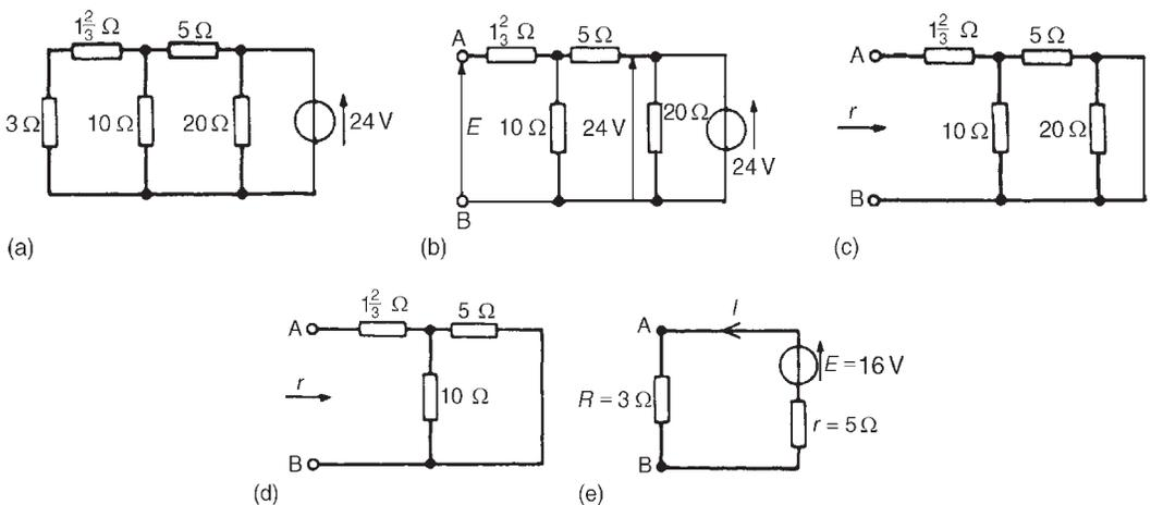
Figure 5.31: Circuit for Example 5.10 showing steps for solution
