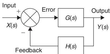
**Figure 18.105: System with negative feedback**
