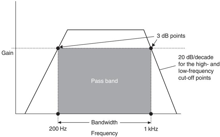
Figure 17.27: Response for filter of Example 17.12
