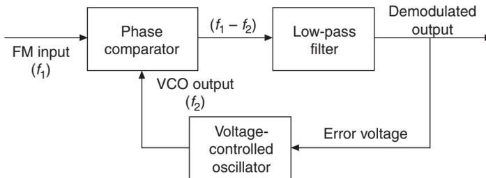
**Figure 19.17: Block diagram of phase-locked loop demodulator**
