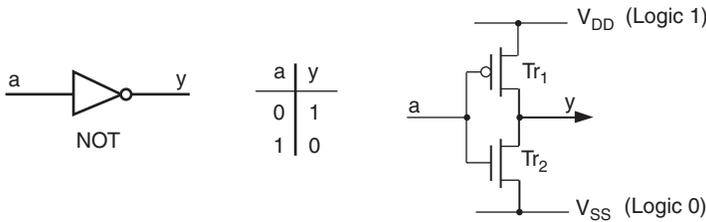
**Figure 10.20: CMOS implementation of a NOT gate**
