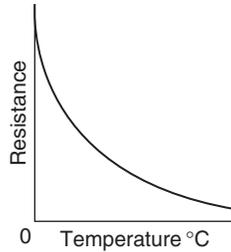
**Figure 18.28: Variation of resistance with temperature for thermistors**
