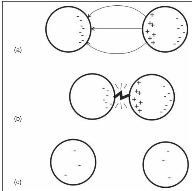
**Figure 20.20: (a) A neutral sphere (right) is brought close to the negative sphere (left); (b) The spheres become very close and a path of ionized molecules forms in the air, causing a spark; (c) After the spark has dissipated, some of the charge has been carried away by the ions in the air. The remaining charge is split equally between the spheres**
