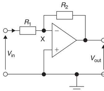
Figure 18.43: Inverting amplifier
