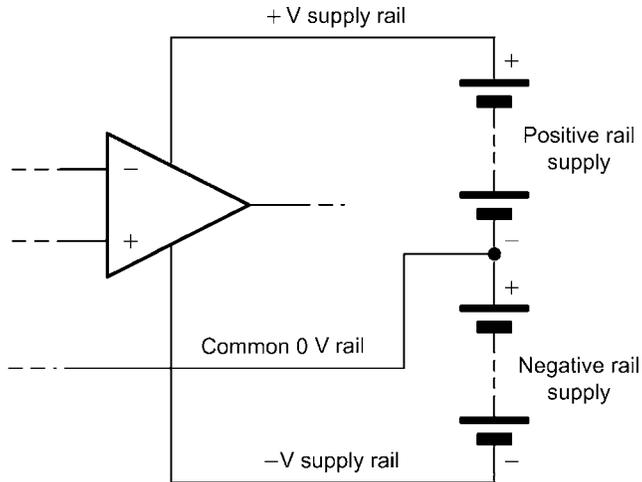
Figure 11.3: Supply connections for an operational amplifier
