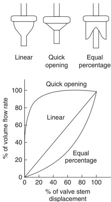
Figure 18.55: Effect of plug shape on flow
