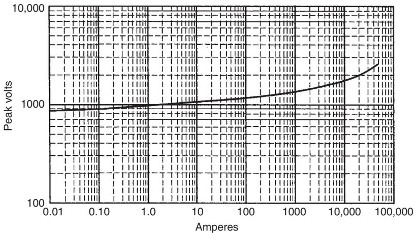
Figure 15.7: 480V, 60-mm MOV characteristic
