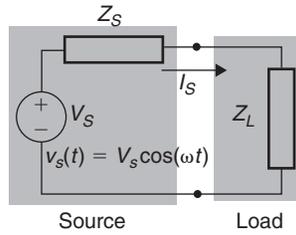
Figure 9.18: Circuit model to derive maximum power transfer
