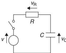
**Figure 18.89:** Electrical system with resistance and capacitance
