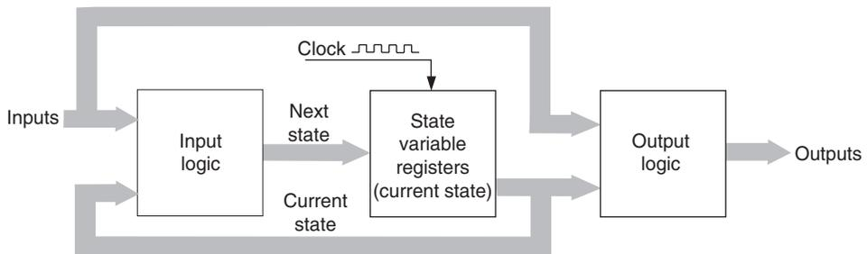
**Figure 10.84: Block diagram of a Mealy machine**
