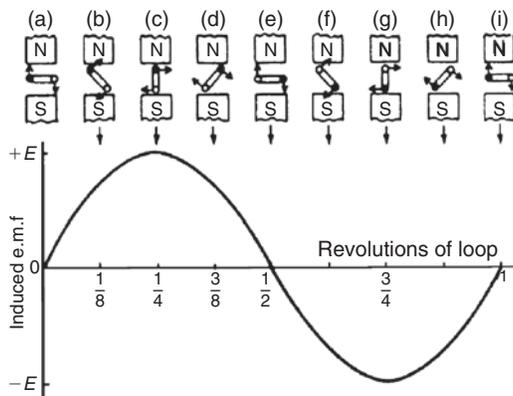
Figure 6.2: One cycle of alternating e.m.f produced
