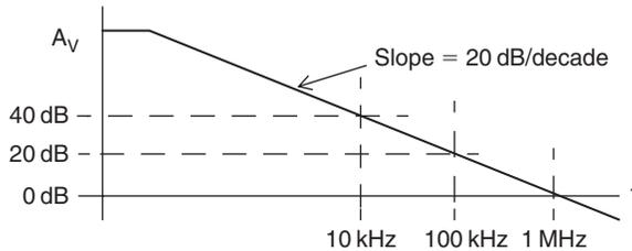
**Figure 11.31: Gain-bandwidth roll-off**
