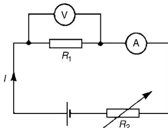
Figure 1.3: Circuit in which current can be varied
