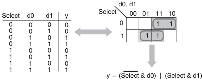
Figure 10.58: Deriving the 2:1 multiplexer equation by means of a Karnaugh Map
