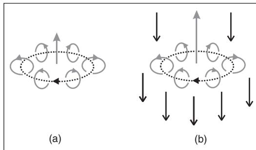
**Figure 21.17: (a) A circulating electron in which the magnetic moment points upward; (b) Applying a downward magnetic field increases the upward moment of the electron. (Recall that an electron has negative charge.)**
