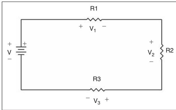
Figure 20.2: A simple circuit demonstrating Kirchhoff's voltage law ( $V = V_1 + V_2 + V_3$ )
