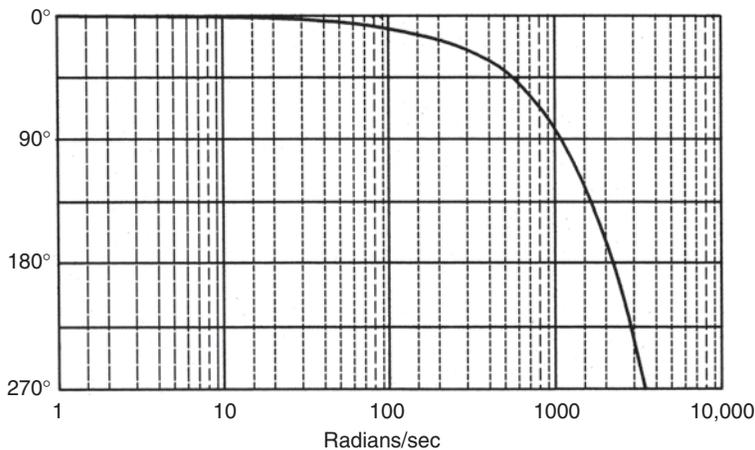
**Figure 15.17: Phase lag of a 1.4-ms transport lag**
