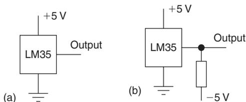
Figure 18.33: LM35 connections
