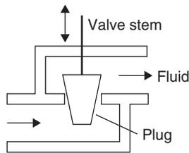
Figure 18.52: Flow controlled by movement of a plug
