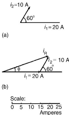
Figure 6.11: Phasor diagrams for Example 6.15
