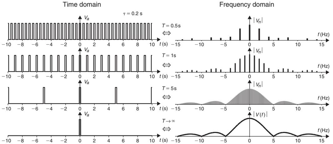
Figure 9.36: The Fourier transform of a rectangular pulse
