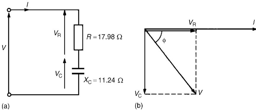
Figure 7.15: (a) Circuit diagram; (b) Phasor diagram
