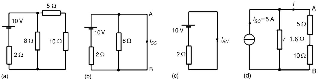
Figure 5.34: Circuit for Example 5.12 showing steps
