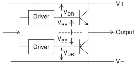
**Figure 11.26: Output voltage swing restrictions**
