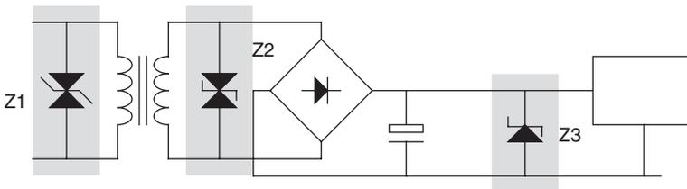
Figure 15.37: Transient suppression in a linear supply
