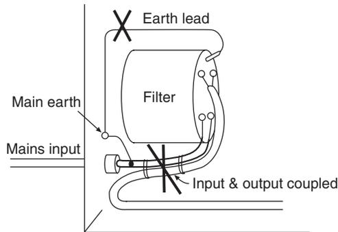
**Figure 25.10: Example of very poor filter installation**
