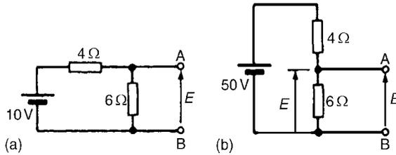
Figure 5.21: (a) Example circuit; (b) Redrawn circuit
