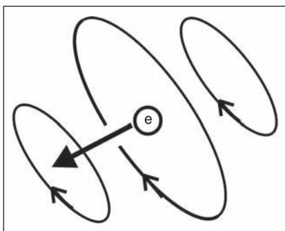
Figure 21.2: Magnetic field lines surround a moving electron
