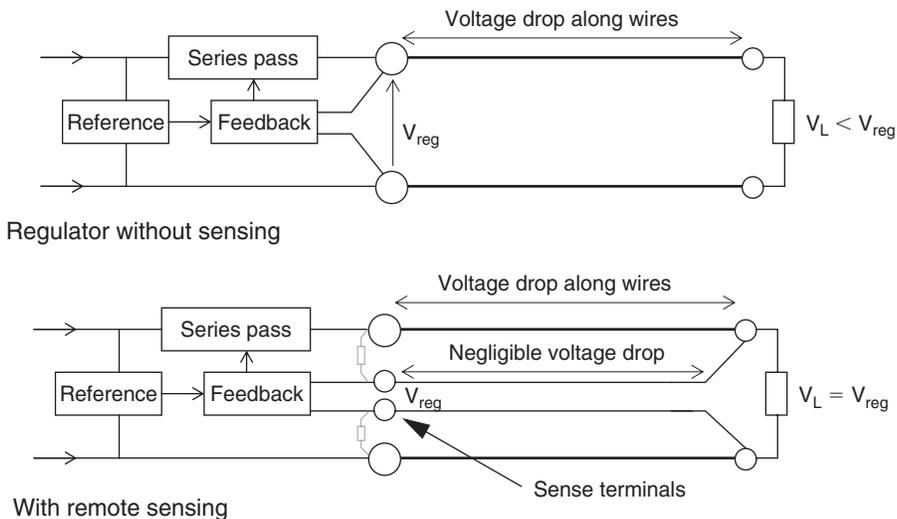
Figure 15.30: Load sensing
