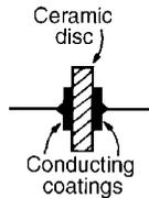
Figure 4.14: Disc construction
