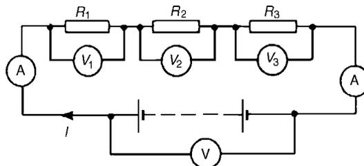
Figure 3.1: Series circuit
