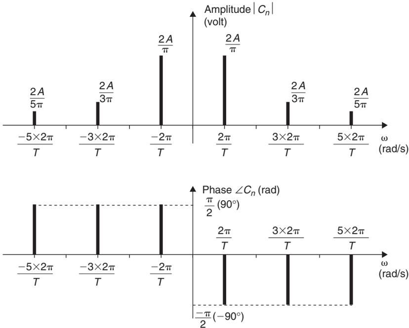
Figure 9.22: Line spectrum of the rectangular waveform
