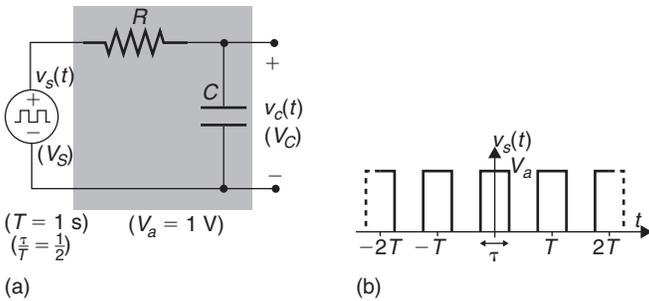
Figure 9.23: (a) Periodic voltage applied to an RC circuit; (b) The periodic voltage  $v(t)$
