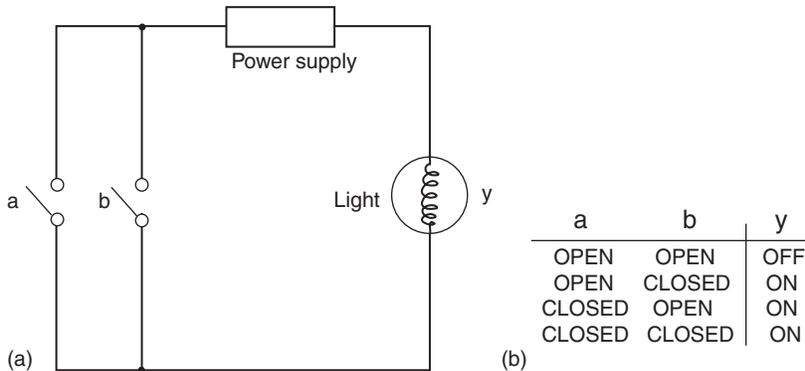
**Figure 10.12: Switch representation of a 2-input OR function (a) Circuit; (b) Truth table**
