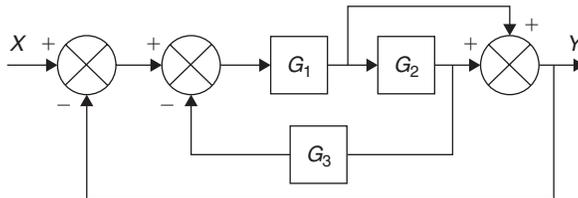
**Figure 18.117: The circuit to be simplified**
