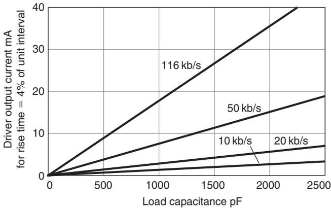
Figure 13.6: EIA-232F transmit driver output current versus  $C_L$
