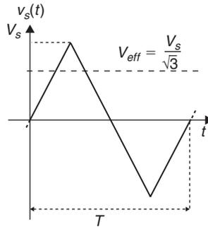
Figure 9.4: Triangular voltage waveform and its corresponding effective voltage
