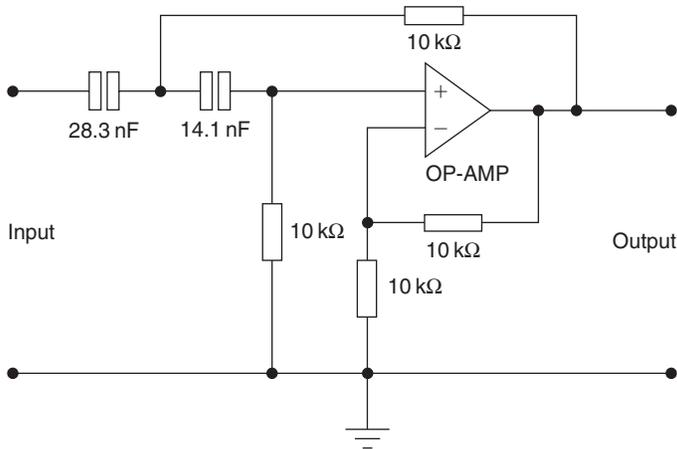
Figure 17.28: High-pass filter (Example 17.13)
