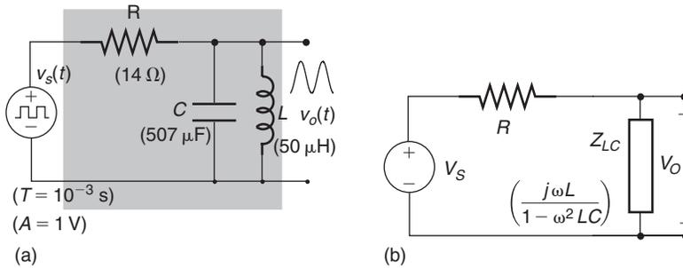
Figure 9.31: (a) RLC circuit; (b) AC equivalent circuit
