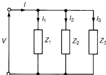
Figure 7.16: Circuit with three impedances in parallel
