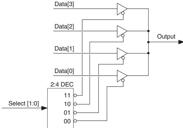
Figure 10.61: Multiple devices driving a common signal
