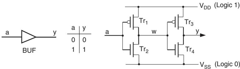
Figure 10.22: CMOS implementation of a BUF gate
