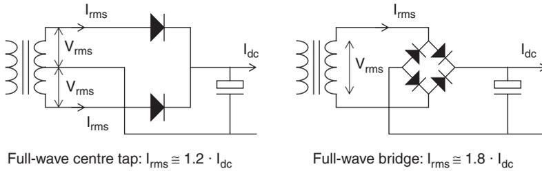
**Figure 15.28: Rectifier configuration**
