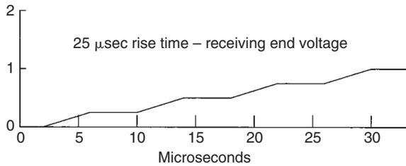
**Figure 23.4: Front-of-wave shaping**
