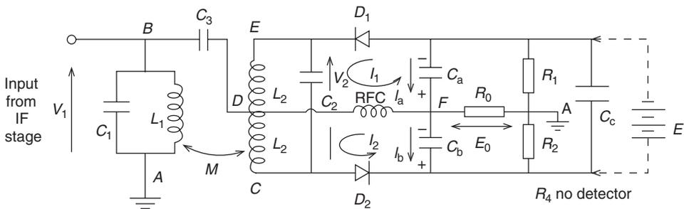
Figure 19.18: Commonly used circuit for FM demodulation
