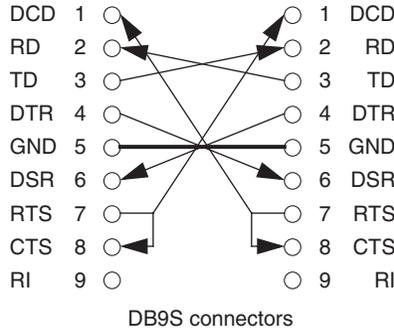
Figure 13.5: The null modem
