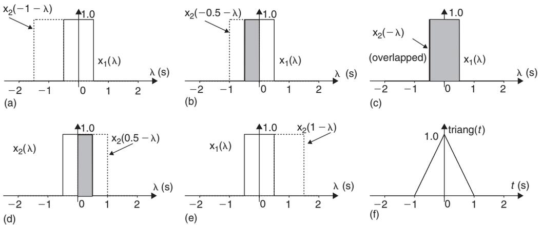
Figure 9.48: Convolution of two identical rectangular waveforms
