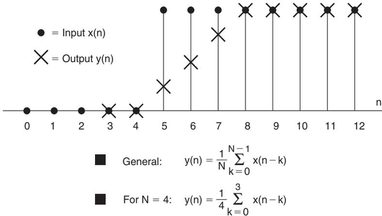
Figure 17.83: 4-tap moving average filter step response
