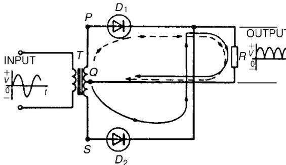
Figure 6.15: Full-wave rectification
