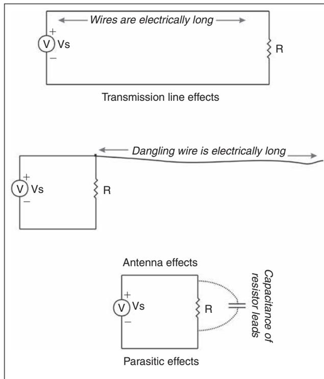
Figure 20.6: Some effects that occur in high-frequency circuits
