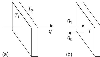
Figure 18.91: (a) Thermal resistance; (b) thermal capacitance
