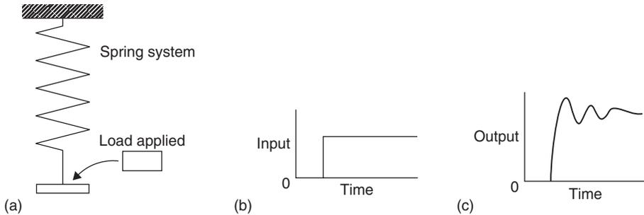
**Figure 18.79: (a) The spring system with a constant load applied at some instant of time; (b) the step showing how the input varies with time; (c) the output showing how it varies with time for the step input**
