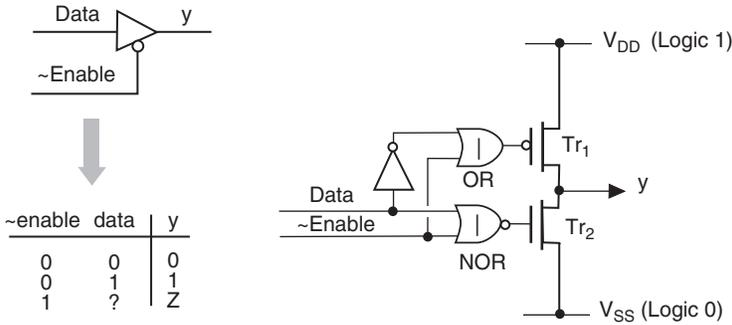
Figure 10.60: Tri-state buffer with active-low enable
