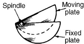
Figure 4.9: End view of variable air capacitor
