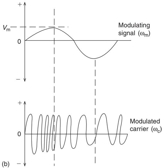
**Figure 19.11: Use of modulating square or sine wave in frequency modulation**
