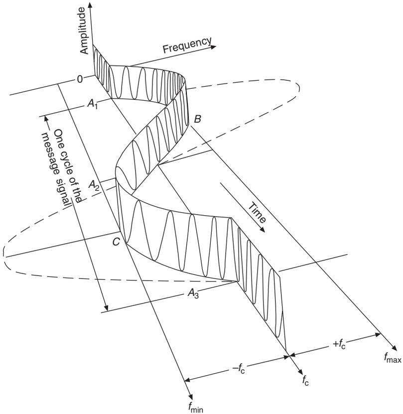
**Figure 19.10: Constant-amplitude carrier is frequency-modulated by single tone**
