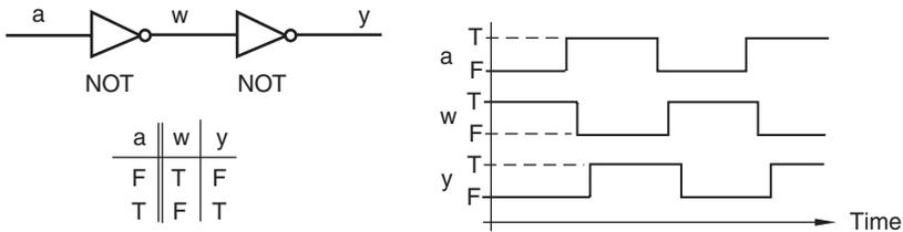
Figure 10.14: Two NOT functions connected together in series
