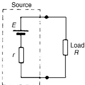
Figure 5.47: When  $r = R$ , power transfer is maximum
