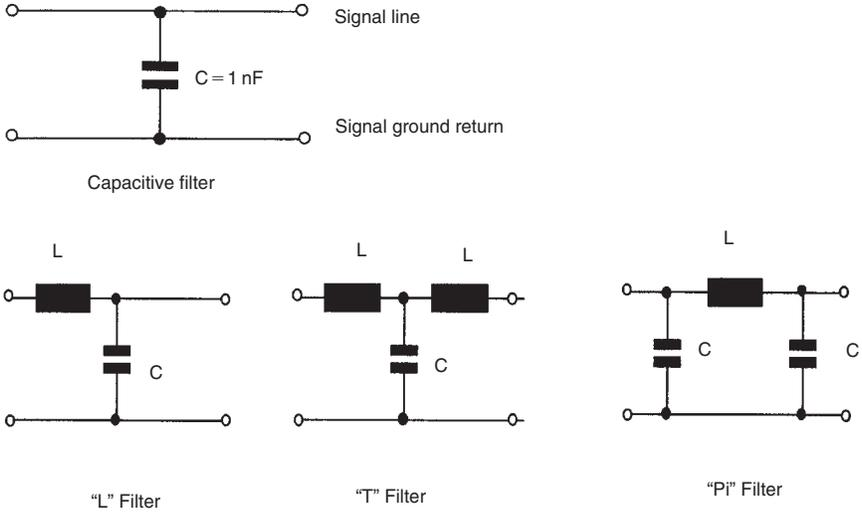
Figure 25.8: Signal line filters
