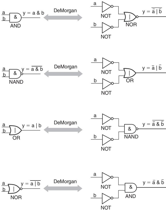
Figure 10.41: DeMorgan Transformations of AND, NAND, OR, and NOR functions
