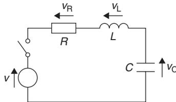
Figure 18.90: Electrical system with resistance, inductance and capacitance
