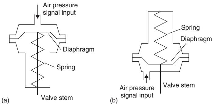
Figure 18.53: (a) Direct action; (b) reverse action
