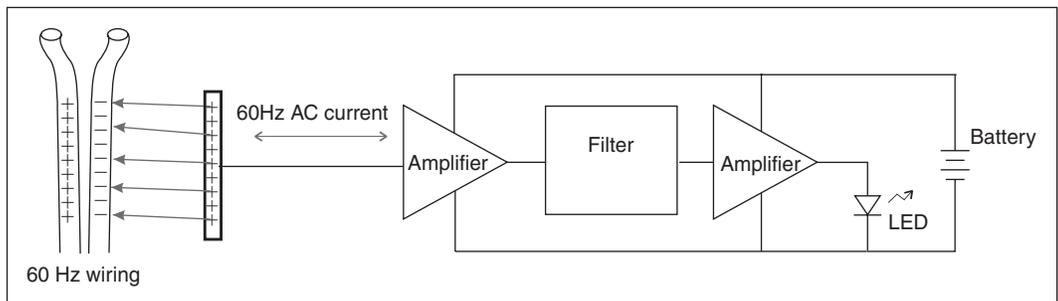
Figure 20.18: Block diagram for a noncontact field detector
