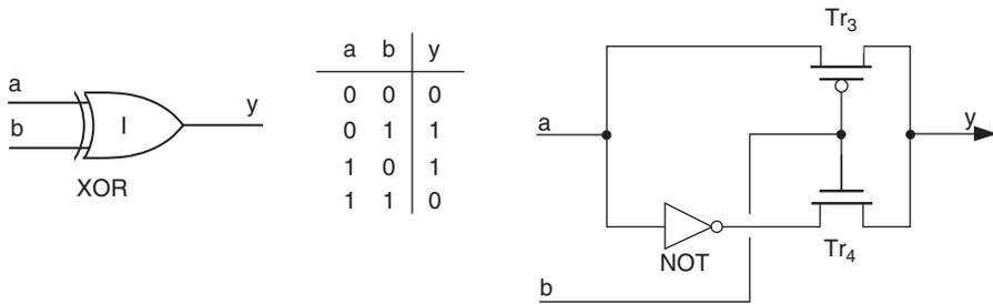
Figure 10.29: CMOS implementation of a 2-input XOR gate
