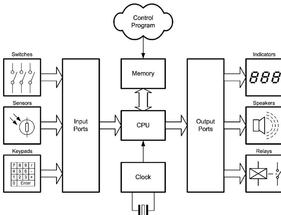
**Figure 14.11: A microcontroller system with typical inputs and outputs**
