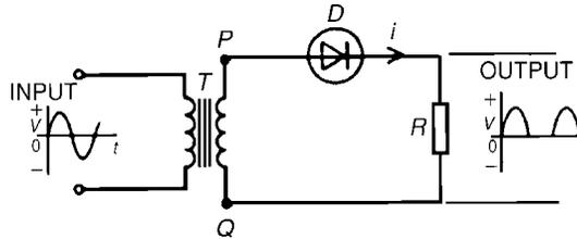
Figure 6.14: Half-wave rectification
