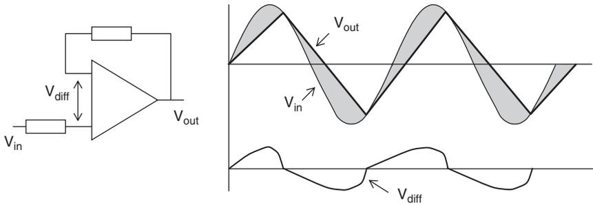
**Figure 11.30: Slewing distortion**
