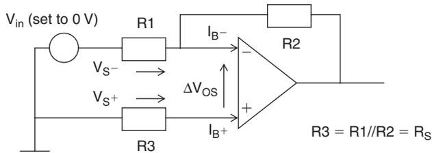
Ideal situation:  $I_B$ ,  $R_S$  equal at + and - terminals, so  $V_{S+} = V_{S-} = I_B \cdot R_S$  and  $\Delta V_{OS} = 0$
