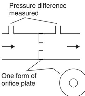
Figure 18.24: Orifice plate
