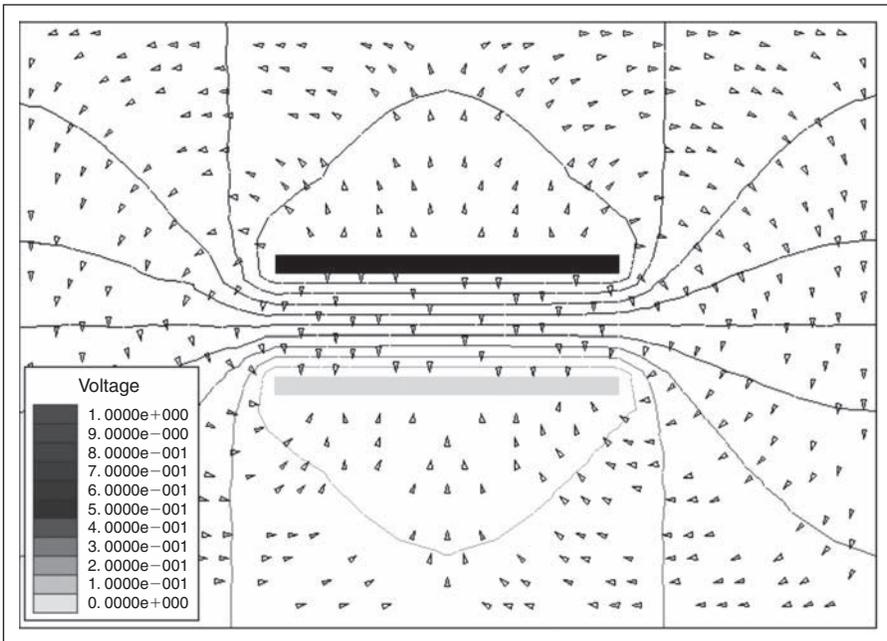
**Figure 20.21:** Electric field surrounding a capacitor with DC voltage applied. This figure was created using Ansoft Corporation's Maxwell 2D field solver software (<http://www.ansoft.com>)
