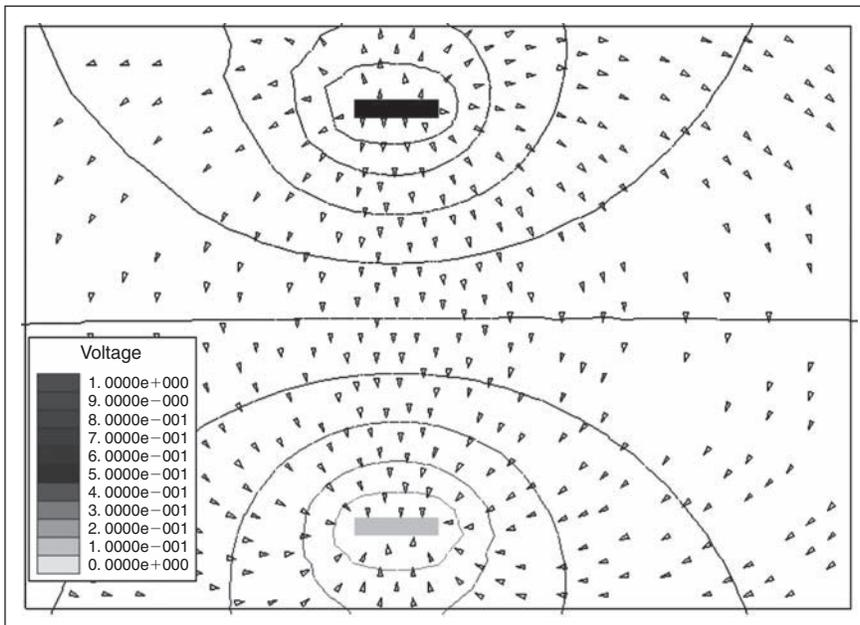
**Figure 20.22: Electric field surrounding another capacitor with DC voltage applied. This figure was created using Ansoft Corporation's Maxwell 2D field solver software (<http://www.ansoft.com>)**
