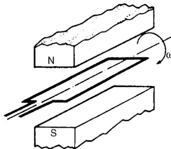
Figure 6.1: Coil rotates at constant angular velocity
