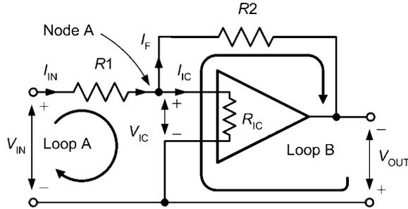
**Figure 11.6: Operational amplifier with negative feedback applied**
