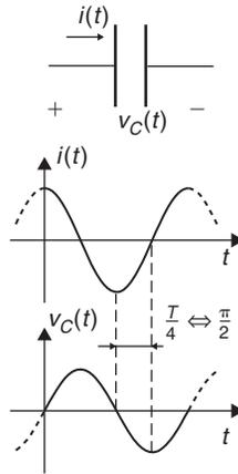
Figure 9.6: Voltage and current in a capacitor
