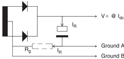
**Figure 15.31: Incorrect reservoir connection**
