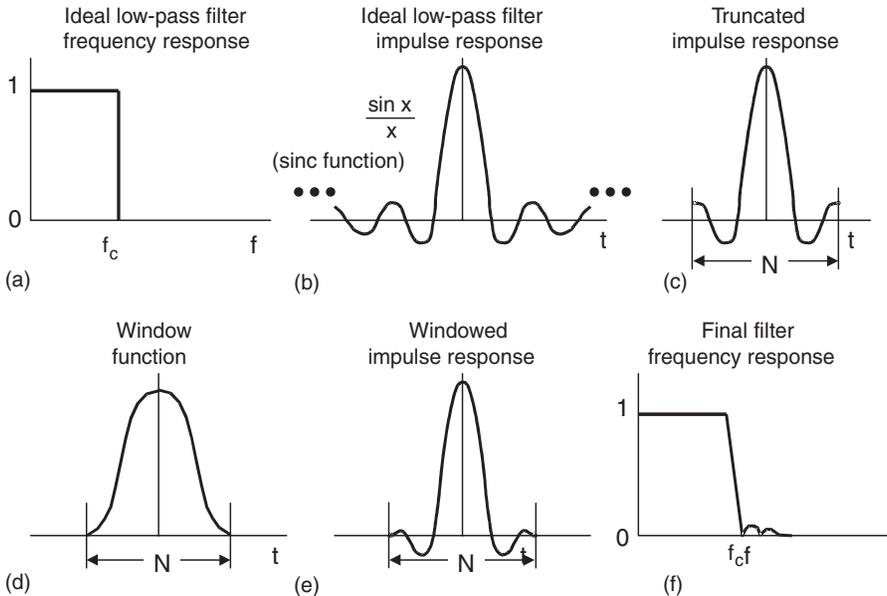
**Figure 17.94: FIR filter design using the windowed-sinc method**
