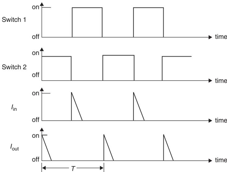
Figure 17.32: Current into and out of switched capacitor filter
