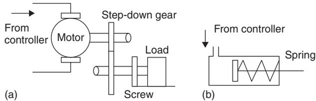
Figure 18.11: Actuator examples: (a) motor; (b) cylinder
