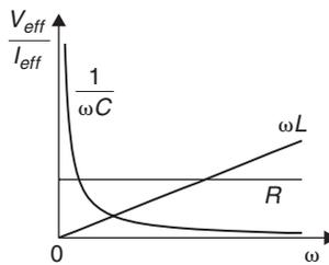
Figure 9.8:  $V_{eff}/I_{eff}$  versus  $\omega$  for passive elements
