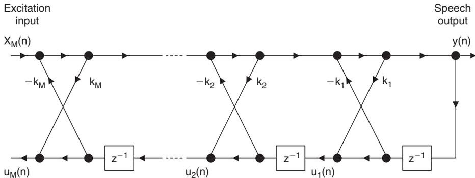
Figure 17.124: All pole lattice filter
