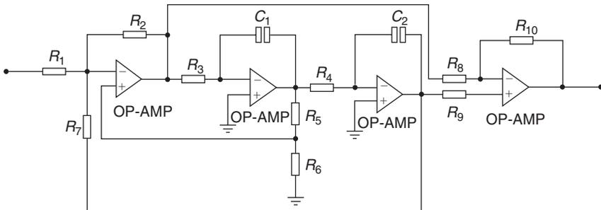
Figure 17.38: Using state variable filter as notch filter
