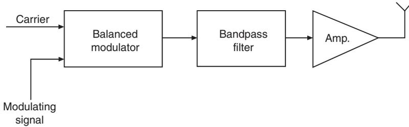
**Figure 19.7:** Basic principle of single-sideband suppressed carrier modulation
