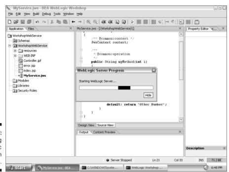
Figure 11-7: Running WebLogic from Workshop. If you access the URL of the web service from a browser, you enter a web application that WebLogic provides for testing your web service. Using this approach, you can quickly test your web application without the need to create a client program.
