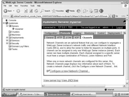
Figure 4-3: Current network channels.
