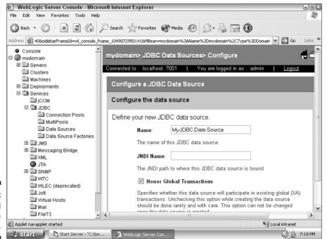
Figure 12-4: Configuring the data source. Now you're ready to see whether your EJBs can access your newly created data source and connection pool. This topic is covered in the next section.
