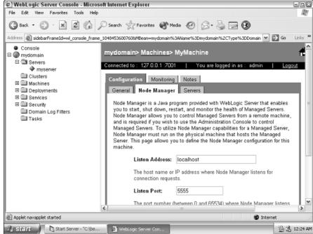
Figure 4-6: Setting up an address and a port.
