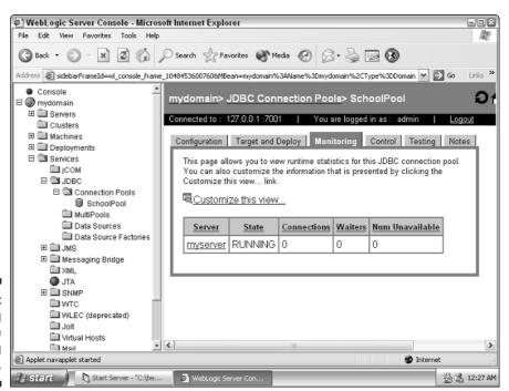
Figure 4-8: Beginning the monitoring process. The monitoring page shows you how many connections are active, how many threads are waiting on a connection, and how many connections are unavailable. From here, you can monitor your connection.
