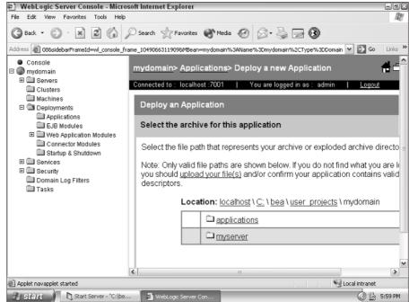
Figure 8-2: Deploying a new application.
