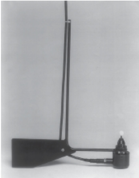
Fig. 5.5 Submersible scalar irradiance sensors. (a) Li-Cor Spherical Quantum Sensor LI-193SB, in lowering frame (Li-Cor Inc., Lincoln, Nebraska, USA). (b) Biospherical Quantum Scalar Irradiance Sensor QSP-200, in lowering frame (courtesy of Biospherical Instruments Inc., San Diego, California, USA).
