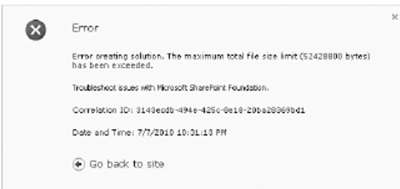
Figure 12.18 Error that results from attempting to create a template that is too large.
