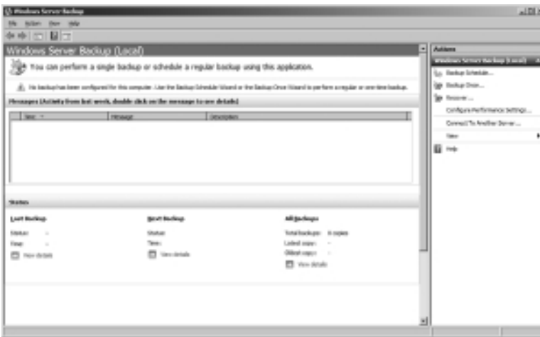
Figure 5.23 The Windows Server Backup MMC snap-in.
