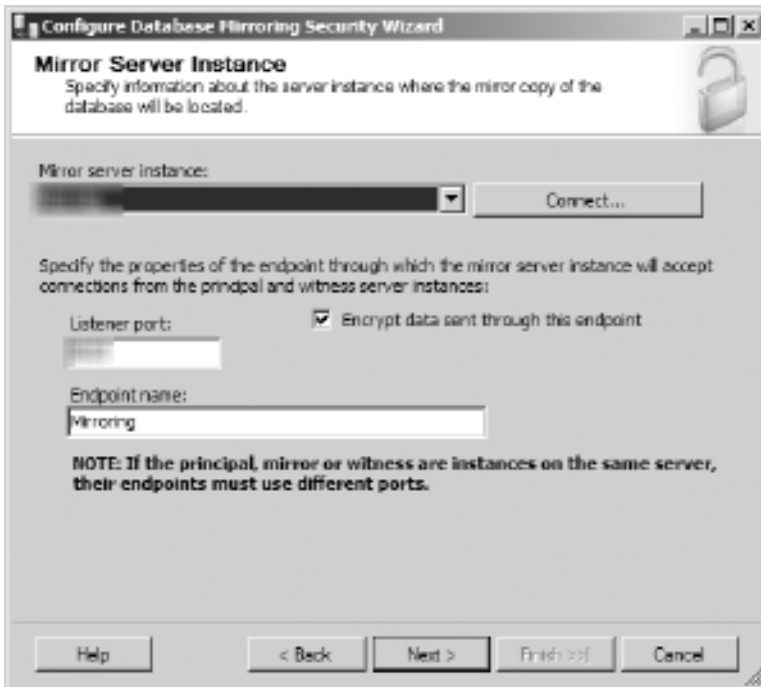
Figure 8.17 The Mirror Server Instance screen in the Configure Database Mirroring Security Wizard.
