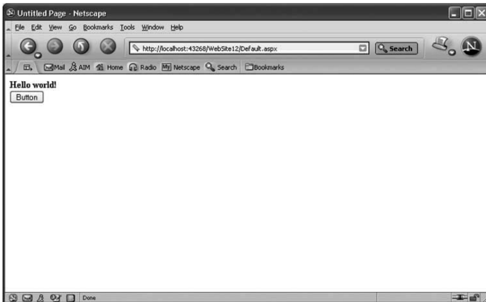
Figure 7-2 The DisplayMessage() subroutine is called when the visitor clicks the Display button.
