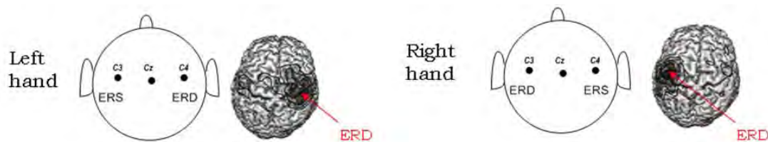
Figure 16. ERD/ERS from left/right-hand motor imagery
