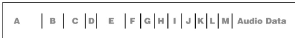
Figure 2.5. The MP3 frame header represented visually
