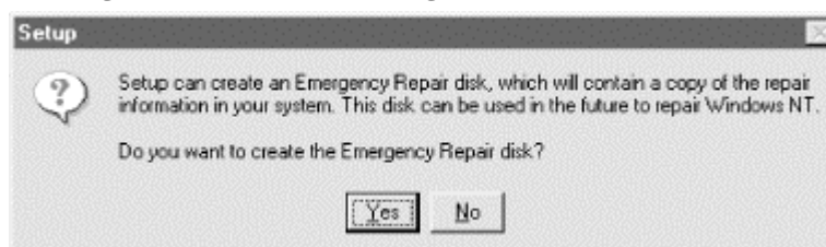
Figure 3.4. Generating an ERD with RDISK
