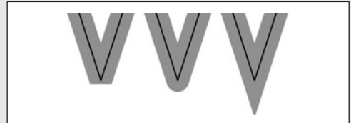
F The three joint styles, bevel (left), round (middle), and miter (right).
