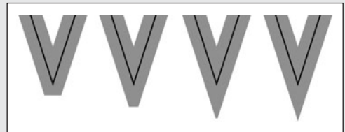
G This small angle is chopped off with miter limits of 1, 2, and 3 but extends fully with a limit of 4 or greater.
