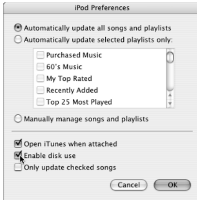
Figure 25-1: Select the Enable Disk Use option to use the iPod as a Mac hard drive.
