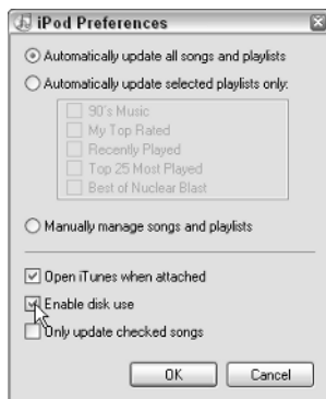
Figure 25-3: Select the Enable Disk Use option to use the iPod as a Windows hard drive.
