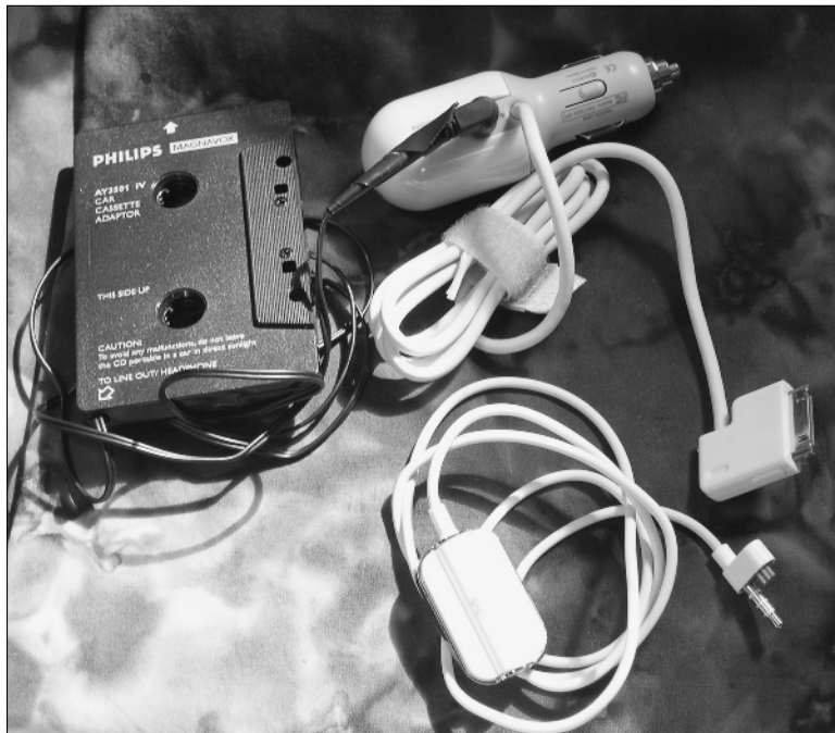
Figure 17-1: Our car accessories: cassette-player adapter (left); power adapter (upper right); and Apple Remote (lower right).
