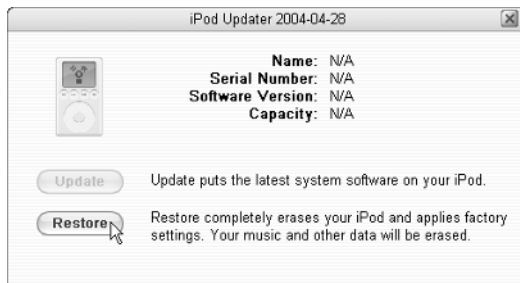
Figure 2-6: Use the iPod Updater to restore the iPod to factory con- ditions for Windows.
