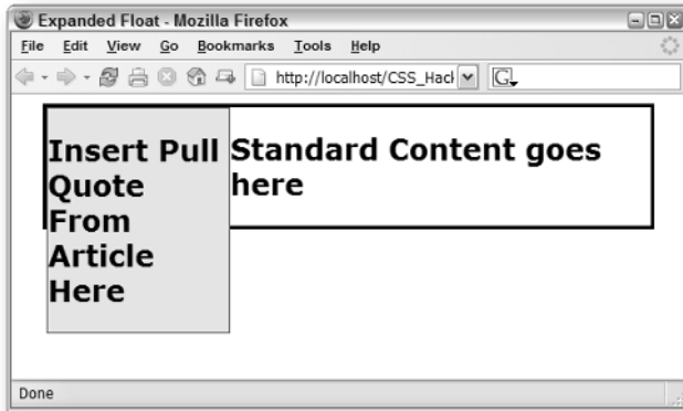
FIGURE 3-10: It may look funky, but the expanded float dropping outside of the container is actually the way CSS specifications intended it.
