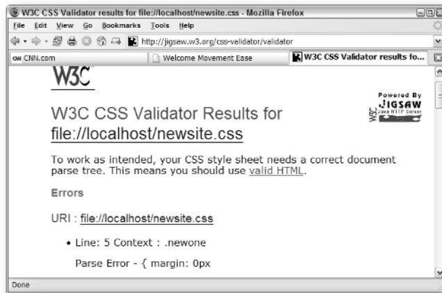
FIGURE 11-4: Validate your CSS to check for syntax errors such as omitted closing curly brackets.
