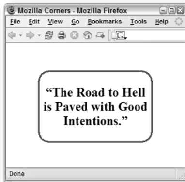
FIGURE 7-6: You can get a rounded border without images, but only in Gecko-based browsers for now.
