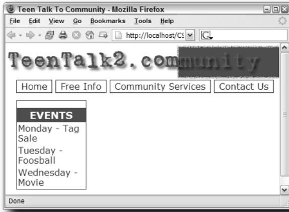
FIGURE 9-6: To maintain both positioning and flexibility, wrap your absolutely positioned styles with a position: relative style.
