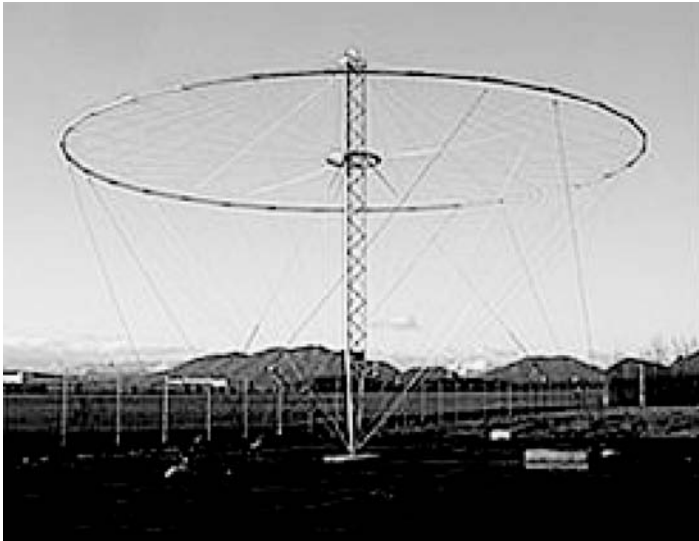
Figure 10.25 HF omnidirectional antenna. Reproduced from Andrew Corporation.
