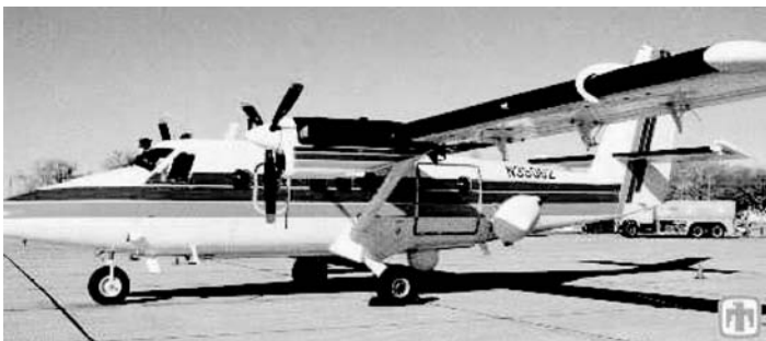
Figure 11.35 Typical small private aircraft antennas (VHF and HF on top of fuselage).
