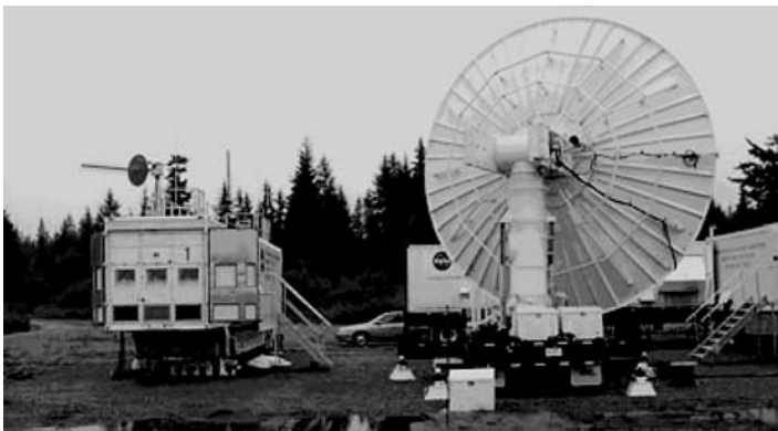
Figure 6.5 Telemetry system in the S band 2.3–2.4 GHz.
