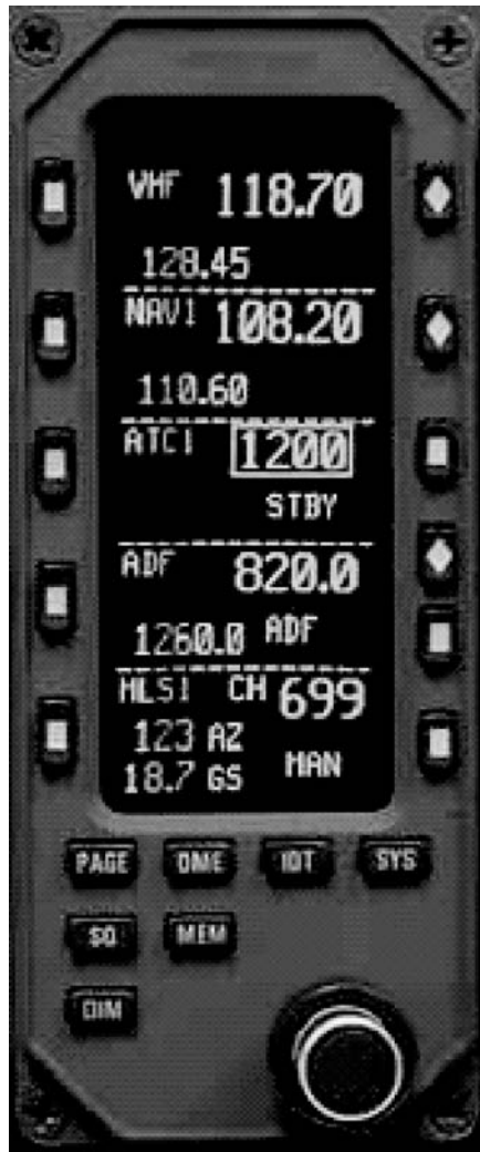
Figure 11.21 NAV/COMM control panel.
