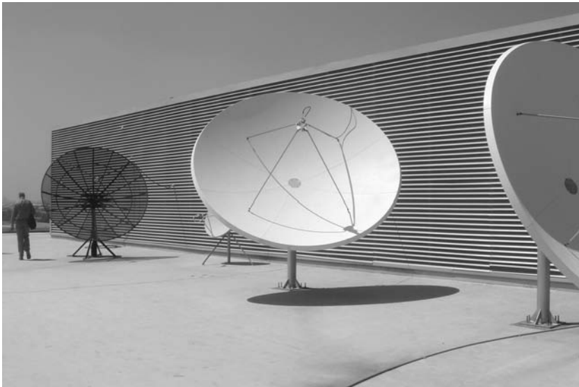
Figure 10.23 Parabolic dish antenna (high-performance, low-wind-loading and Gridpack versions).
