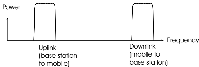
Figure 2.74 Frequency domain duplex (FDD) operation.
