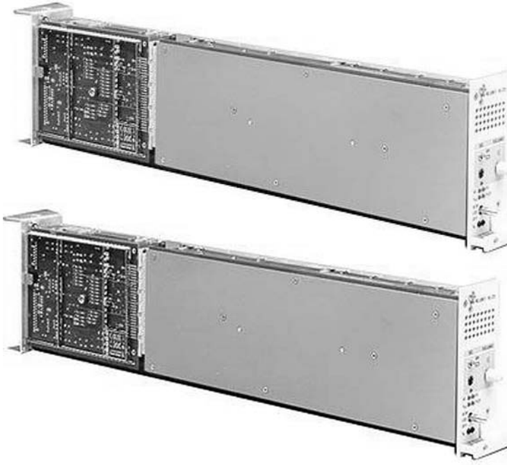
Figure 10.2 Typical rack mount transmitter. Reproduced from Rohde and Schwarz.
