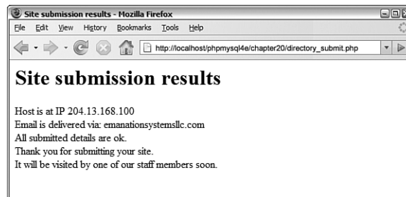
Figure 20.3 This version of the script displays the results of checking the hostnames for the URL and email address; a production version might not display these results, but it is interesting to see the information returned from the checks.
