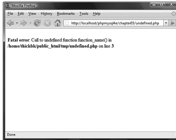
Figure 5.3 This error message is the result of calling a function that does not exist.
