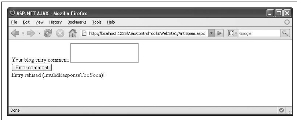
Figure 12-9. The server refuses the data because it was submitted multiple times too quickly
