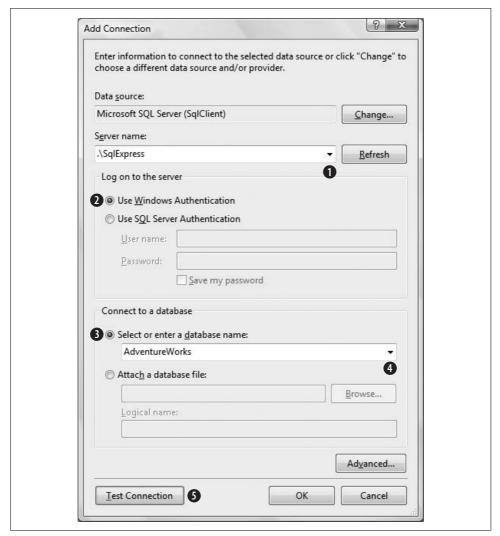
**Figure 4-5**. The Add Connection dialog is where you specify a new connection for your data source. Select the server, the logon credentials, and finally the database you want to use.
