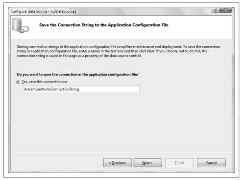
**Figure 4-7**. It's a good idea to save the connection string in the application's web.config file, so you can use it again with other controls.
