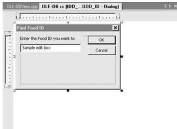
**Figure 8-2:** The Find Food ID dialog box enables the user to search for a specific record.
