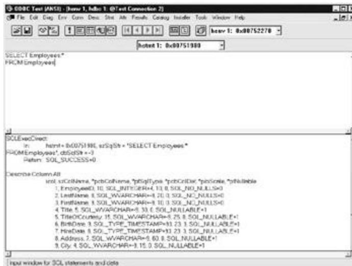
**Figure 7-4:** Working with ODBC Test often means combining SQL statements with menu commands to achieve a specific result.
