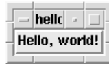
Figure 2.1. The “hello world” application. All of the decorations around the “Hello, world!” button are provided by the mwm window manager. If you use a different window manager then your decorations may be different.
