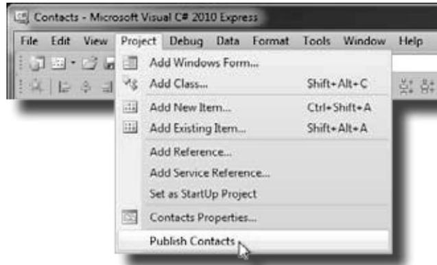
Building the solution just copies the files to your local machine. Publish creates a Setup executable and a configuration file so that any machine could install your program.
