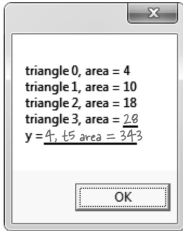
The setArea() method uses the height and length fields to set the area field. Since it's not a static method, it can only be called from inside an instance of Triangle.
