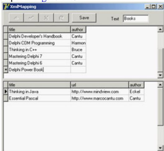
Figure 22.8: The XmlMapping example uses a TransformProvider component to make a complex XML document available for editing within multiple ClientData-Set components.
