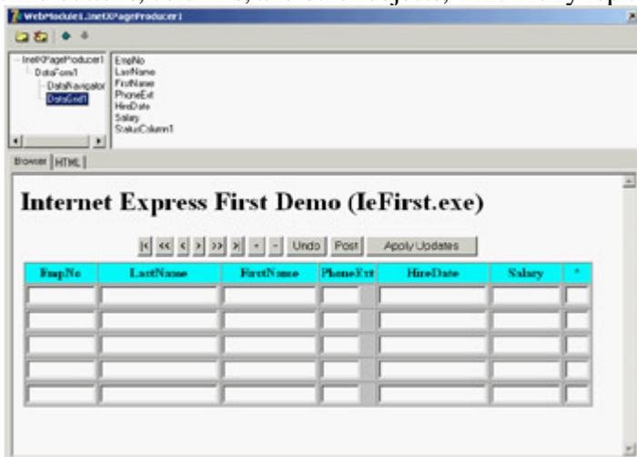
Figure 22.10: The InetXPage-Producer editor allows you to build complex HTML forms visually, similarly to the AdapterPageProducer.
