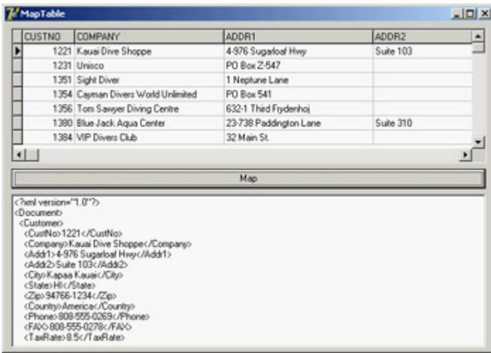
Figure 22.9: The MapTable example generates an XML document from a database table using a custom transformation file.
