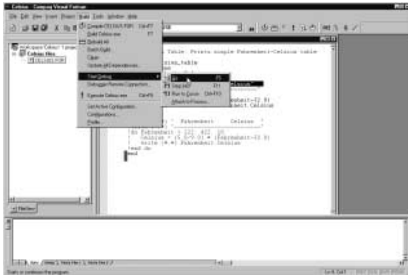
Figure 6-3 Starting the Debugger
