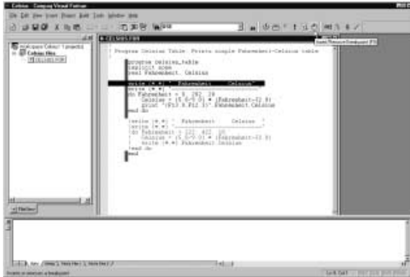
Figure 6-2 Setting the Initial Breakpoint in the Debugger
