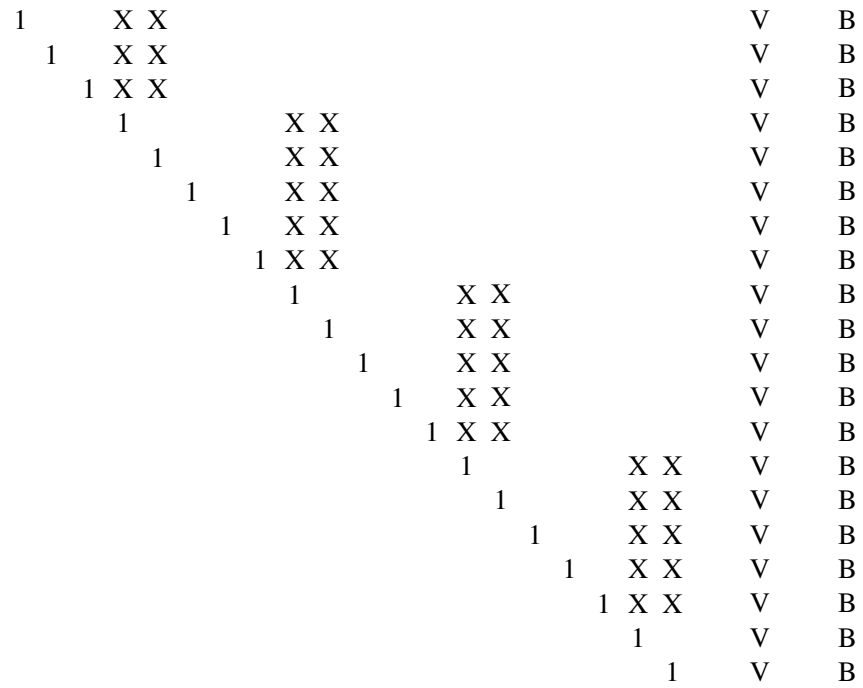
Figure 17.3.2. Target structure of the Gaussian elimination. Once the matrix of Figure 17.3.1 has been reduced to this form, the solution follows quickly by backsubstitution.
